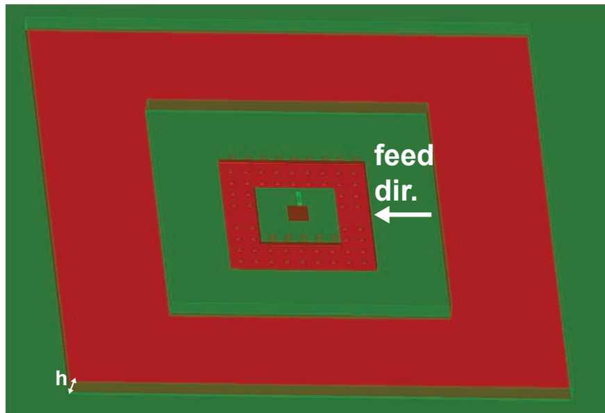
Figure 5.60: Patch with grounded via ring and partial substrate removal
