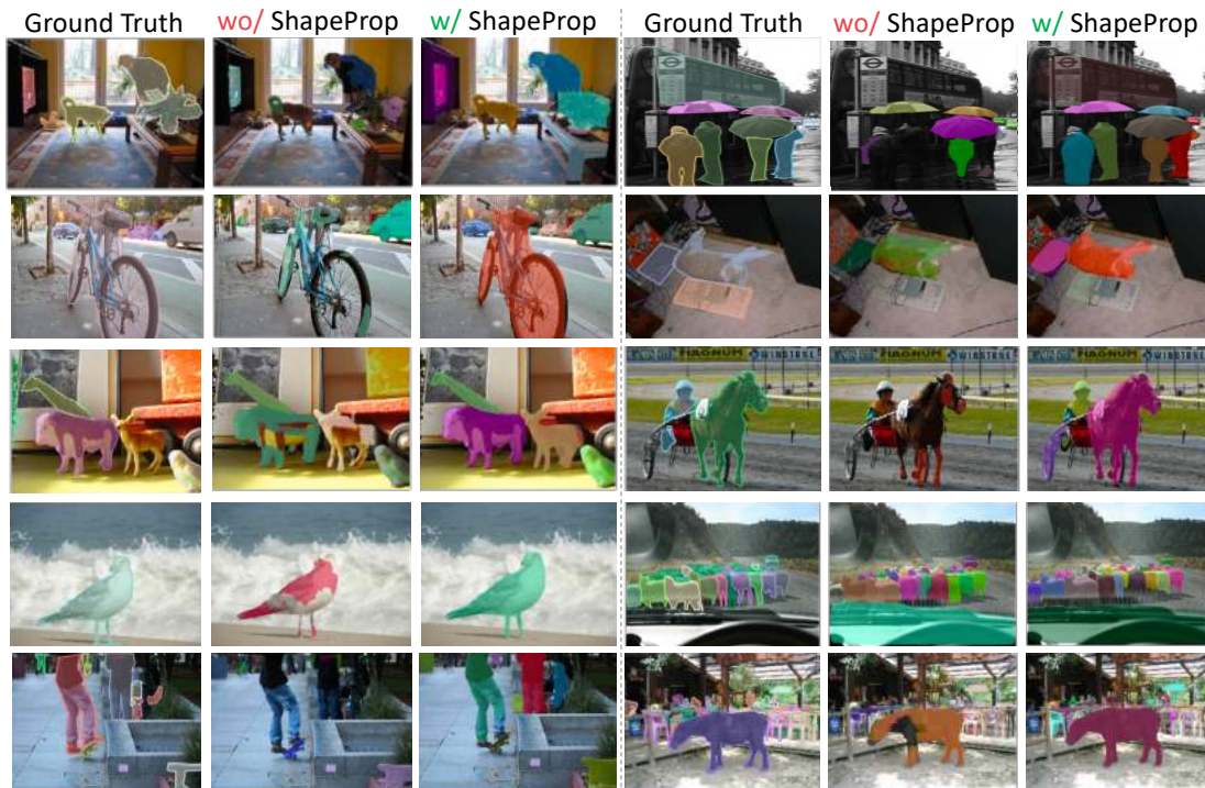
Figure 8.7: Visualization of Mask R-CNN (w/ or wo/ ShapeProp)’s results on novel categories.
