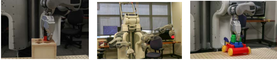
(a) Shape matching, the PR2 robot insert shape into its matching hole. (b) Reaching, the PR2 moves its end-effector to an pre-specified goal. (c) Lego stacking, the PR2 assembles one lego block on top of another.
