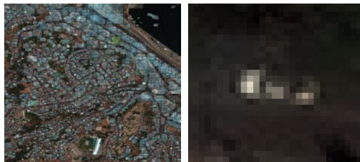
Figure 5.3: Example of dense detections in an urban chip and the low resulting resolution of a small object (car)
