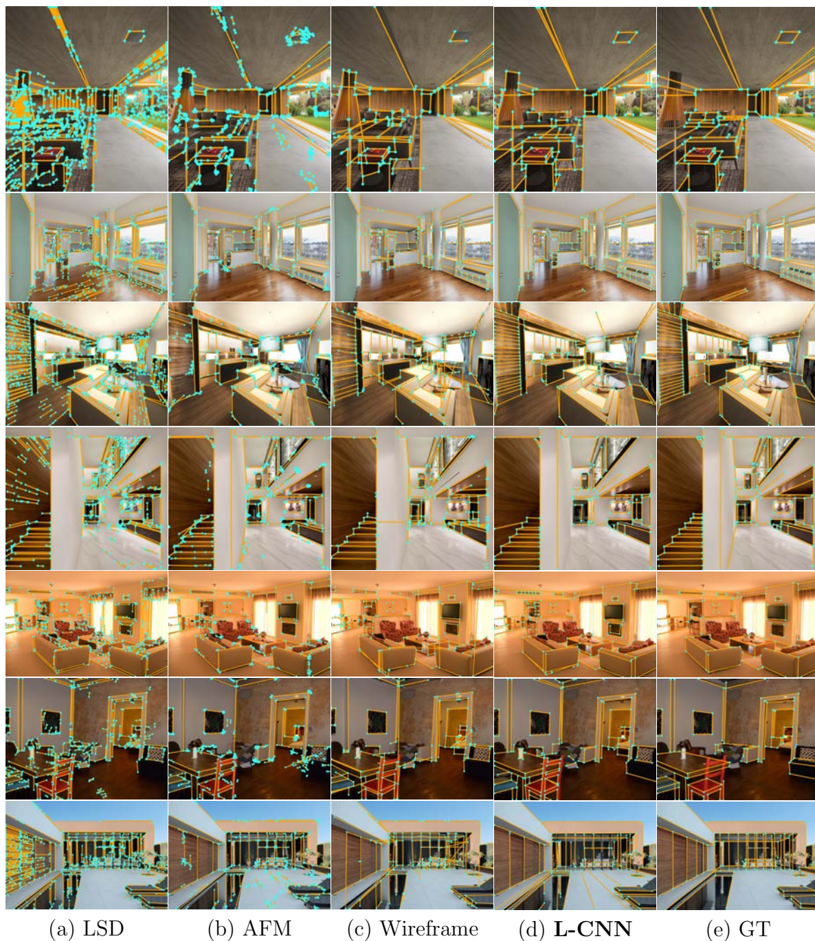
Figure 2.5: Qualitative comparison of wireframe and line detection methods. From left to right, the columns shows the results from LSD [146], AFM [162], Wireframe [63], L-CNN (ours), and the ground truth. We also draw the detected junctions from Wireframe and L-CNN and the line endpoints from LSD and AFM.
