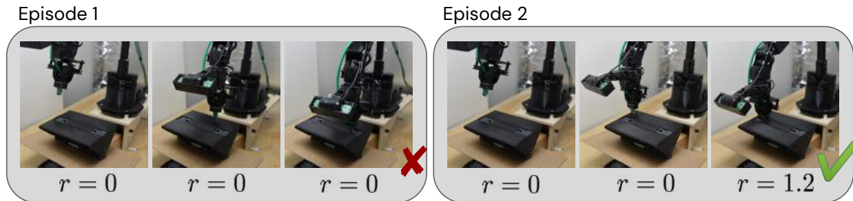
Figure 19: At test time our algorithm MELD enables a 5-DoF WidowX robot to insert the ethernet cable into a novel insertion location and orientation within two episodes of experience, operating from image observations and a sparse task completion signal when the cable is correctly inserted. MELD achieves this result by meta-training a latent dynamics model to capture task and state information, as well a policy that conditions on this information to explore and identify the correct insertion point.
