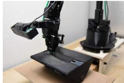
Figure 26: Ethernet cable insertion problem. The automatic reset mechanism changes the position and orientation of the router across tasks.
