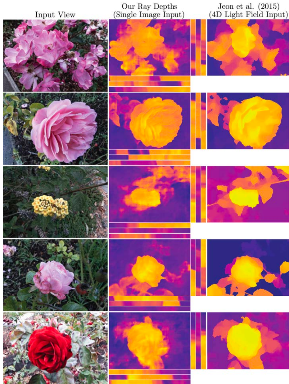
Figure 2.6. We validate our ray depths against the state-of-the-art light field depth estimation. We give Jeon et al. [58] a distinct advantage by providing them a ground-truth 4D light field to predict 2D depths, while we use a single 2D image to predict 4D depths. Our estimated depths are comparable, and in some cases superior, to their estimated depths, as shown by the detailed varying depths of the flower petals, leaves, and fine stem structures.
