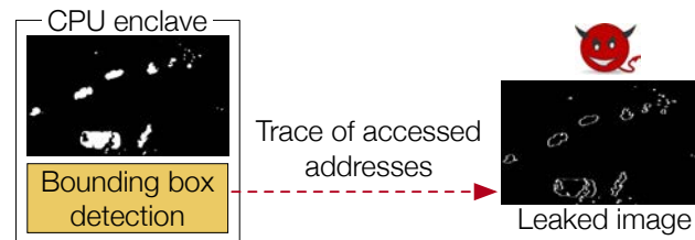
Figure 6.2: Attacker obtains all the frame’s objects (right) using access pattern leakage in the bounding box detection module.
