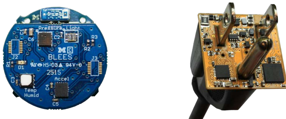
Figure 2.3: BLEES and PowerBlade. At left is BLEES: an environmental sensor capable of sensing temperature, humidity, pressure, light, and acceleration. At right is PowerBlade: a low-profile, plug-load power meter. Both sensors broadcast periodic measurements using BLE advertisements.
