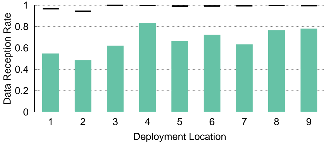
Figure 4.1: Data reception rate by deployment location. Data reception rate is determined by counting sequence numbers received throughout the deployment duration and dividing that by the expected count of sequence numbers. Expected DRR is marked as a black line above each bar. While we expect a DRR of greater than 99% for the majority of locations, we instead find that most locations receive between 50% and 80% of expected measurements.
