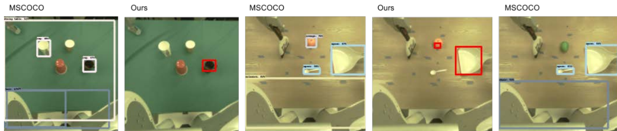
Figure 4.2: Faster RCNN trained on MSCOCO does not differentiate between cups and mugs, and gives higher probability to the cup, making it difficult to train a policy that needs to locate the mug. With our method, the attention can learn to prioritize mugs over cups. The dustpan is labeled as a spoon and thus can be distracted by other spoon-like objects. As limes are not in the MSCOCO dataset, the object detector does not label them.
