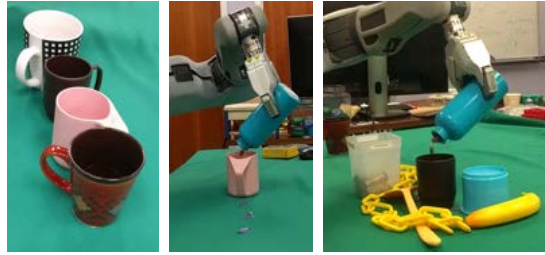
Figure 4.6: Left: Mugs used for evaluation. Note that only the brown mug was seen during training. Center: Successful pouring into the pink mug. Right: Pouring into the brown mug in a cluttered environment that was not seen during training.
