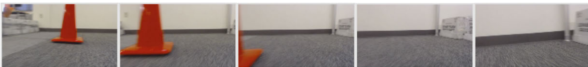
Figure 8.8: Real-world RC car experiments: An RC car learns to drive while avoiding obstacles using our uncertainty-aware reinforcement learning for collision avoidance algorithm (Alg. 7). A successful rollout is shown above.
