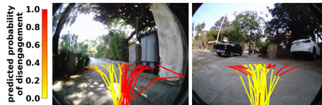
Figure 6.9: Visualization of planning with the disengagement predictive model. Each image shows the candidate paths considered during planning, and are color coded according to their predicted probability of disengagement. These visualizations show the learned model can accurately predict which action sequences would lead to disengagements, including driving into obstacles (left) or streets or driveways (right).
