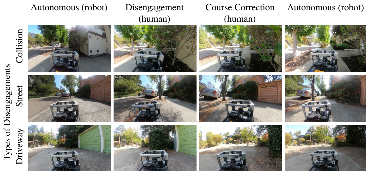
Figure 6.5: Our LaND approach learns to navigate from disengagements. For the sidewalk navigation task studied in our experiments, there are three types of scenarios that will cause the human overseer to disengage the robot’s autonomy mode: colliding with an obstacle, driving into the street, and driving into a driveway. After the robot is disengaged, the human repositions the robot onto the sidewalk and then re-engages autonomy.
