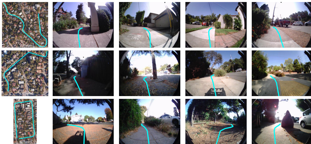
Figure 6.1: LaND is a learning-based approach for autonomous mobile robot navigation that directly learns from disengagements—any time a human monitor disengages the robot’s autonomy. These disengagement datasets are ubiquitous because they are naturally collected during the process of testing these autonomous systems. LaND is able to navigate in a diverse set of sidewalk environments, including parked bicycles, dense foliage, parked cars, sun glare, sharp turns, and unexpected obstacles.
