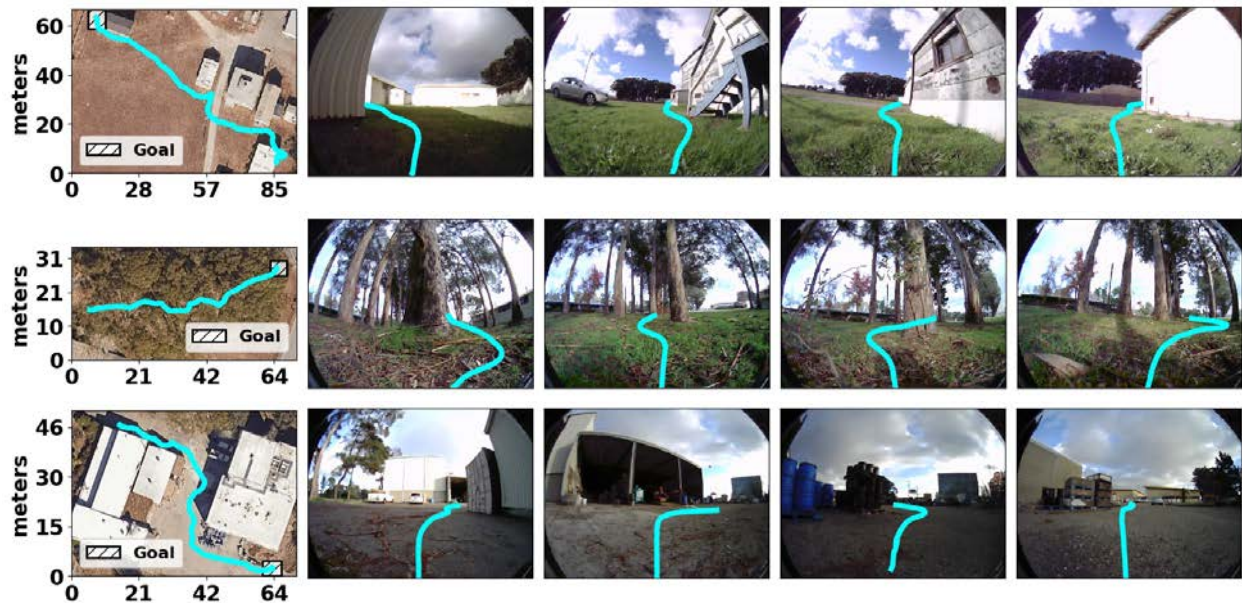
Figure 4.12: Our BADGR policy can generalize to novel environments not seen in the training data. Each row shows the BADGR policy executing in a different novel environment. The first column shows the approximate path followed by the BADGR policy. The remaining columns show sampled images from the onboard camera while the robot is navigating, with the future path of the robot overlaid onto the image.
