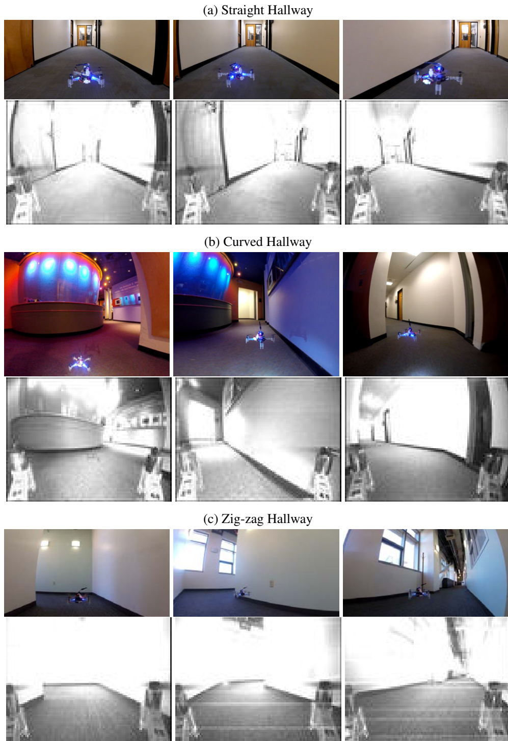
Figure 3.4: Our learning-based approach, using only the onboard, grayscale, 72 \times 96 resolution camera images, flying through a straight, curved, and zig-zag hallway.
