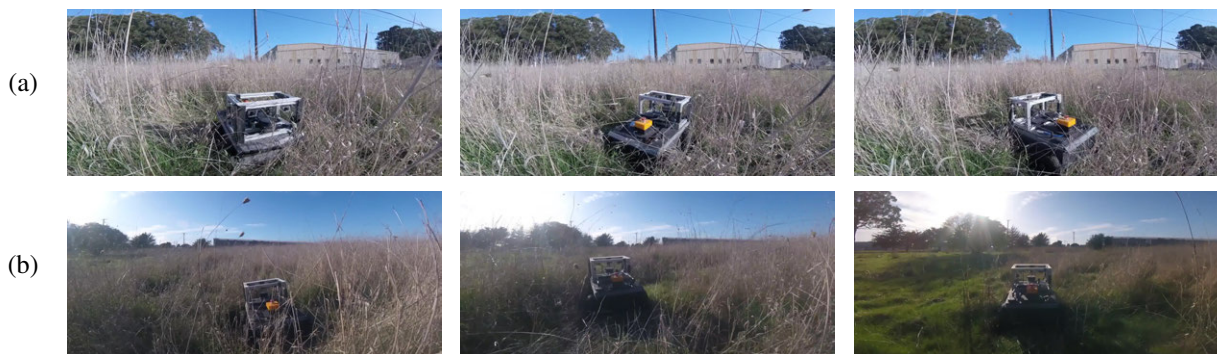
Figure 4.7: Comparison of LIDAR (top) versus our BADGR approach (bottom) in a tall grass portion of the off-road environment. The LIDAR policy incorrectly labels the grass as untraversable, and therefore rotates in-place in an attempt to find a traversable path; after completing a full rotation and failing to detect any traversable path, the LIDAR policy determines the robot is trapped. In contrast, our BADGR approach has learned from experience that some tall grass is indeed traversable, and is therefore able to successfully navigate the robot towards the goal.
