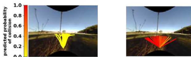
Figure 4.8: Comparison of our BADGR policy (left) versus the LIDAR policy (right). Each image shows the candidate paths each policy considered during planning, and the color of each path indicates if the policy predicts the path will result in a collision. The LIDAR policy falsely predicts the paths driving left or straight will result in a collision with the few strands of tall grass. In contrast, our BADGR policy correctly predicts that the grass is traversable and will therefore drive over the grass, which will result in BADGR reaching the goal 1.5\times faster.
