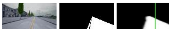
(c) To enable our CAPs approach to learn to stay in the right lane, we trained a model to take as input the onboard RGB image (left) and predict where the road is (right) using labels (center). Once trained the learned segmentation model autonomously labels where the center of the right lane is (green vertical line), the CAPs model can learn to keep the center of the right lane in the middle of its camera view.
