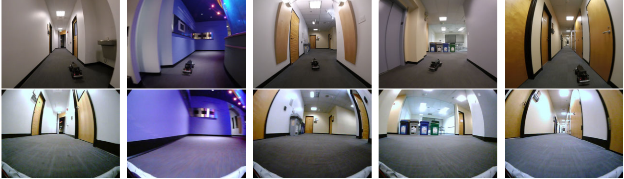
Figure 5.5: Third-person images (top row) and first-person images from the onboard camera (bottom row) from the RC car navigating through the 5th floor of Cory Hall at UC Berkeley for the task of avoiding collisions, following desired goal headings, and going towards doors using our CAPs approach.
