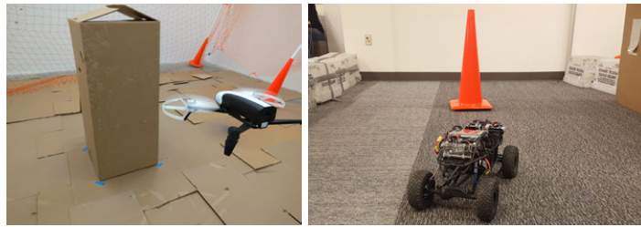
Figure 8.1: Uncertainty-aware collision prediction model for collision avoidance: A quadrotor and an RC car are tasked with navigating in an unknown environment. How should the robots navigate while avoiding collisions? We propose a model-based reinforcement learning approach in which the robot learns a collision prediction model by experiencing collisions at low speed, which is unlikely to damage the vehicle. We formulate a velocity-dependent collision cost that uses collision prediction estimates and their associated uncertainties to enable the robot to only experience safe collisions during training while still approaching the desired task performance.
