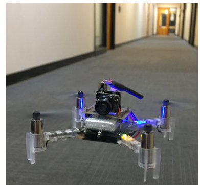
Figure 3.1: Our autonomous quadrotor navigating a building from raw monocular images using a learned collision avoidance policy trained with a simulator and one hour of real-world data.
