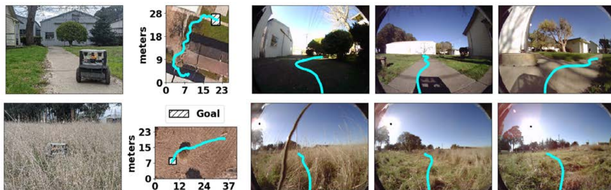
Figure 4.1: BADGR is an end-to-end learning-based mobile robot navigation system that can be trained with self-supervised off-policy data gathered in real-world environments, without any simulation or human supervision. Using only RGB images and GPS, BADGR can follow sparse GPS waypoints without colliding while (top row) preferring smooth concrete paths and (bottom row) ignoring geometrically distracting obstacles such as tall grass.
