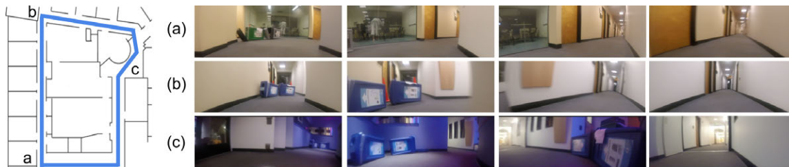
Figure 2.9: Real-world RC car experiments on the 5th floor of Cory hall. The path the robot can follow is drawn on the floor plan (left), however, this path is not provided to the RC car. Three example trajectories of the RC car navigating with our learned policy are shown.
