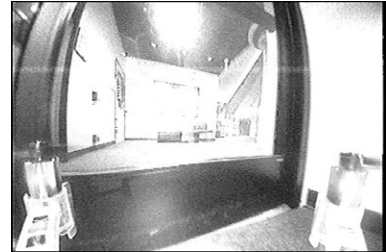
Figure 3.5: Example failure: collision with a glass door.
