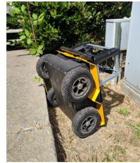
Figure 4.4: While collecting data, the robot will periodically require a manual intervention to reset from catastrophic failures, though recovery is usually automatic.
