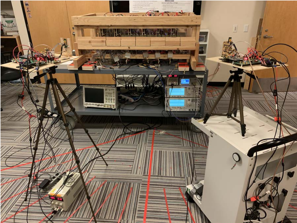
Figure 5.3: Configuration of base station and user equipment for measurement.
