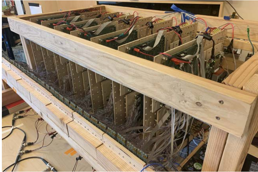
Figure 4.4: Spine slices assembled into full base station
