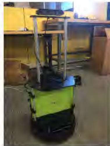
Figure 7.7: Our Turtlebot 2 hardware platform uses a Yujin Kobuki base, Gigabyte Aero Laptop, and Orbbec Astra camera.
