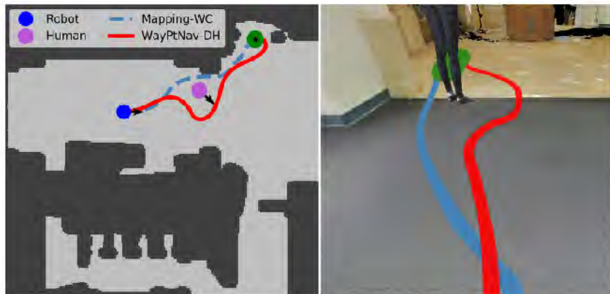
Figure 7.14: Topview of the trajectories taken by Mapping-WC and LB-WayPtNav-DH from the same state and the corresponding RGB image with the trajectories superimposed. Mapping-WC reaches the goal faster than LB-WayPtNav-DH as it has access to precise geometry of the scene and the human state and thus plans a path between the human and the wall which narrowly avoids collision. LB-WayPtNav-DH, on the other hand, takes a more cautious path as it does not have access to the human state.
