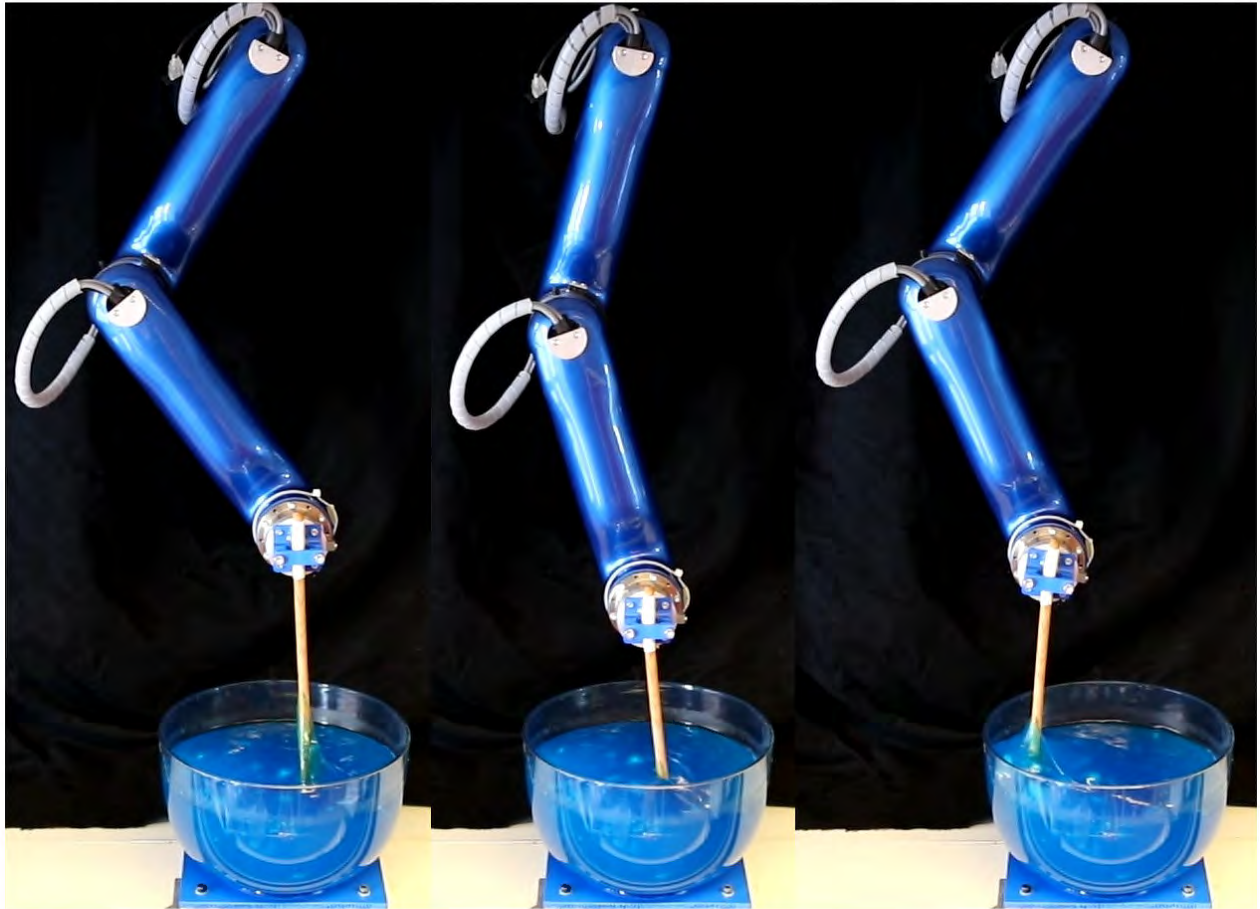
Figure 6.12: Stirring viscous liquid with the 3-dof SCARA robot CARBO using aDOBO.
