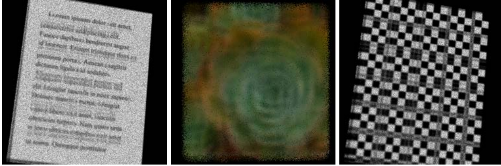
Figure 31: Images showcasing the double image artifact. In the text image every other line appears twice. The checkerboard image shows how the artifact is periodic and occurs both vertically and horizontally through the image.
