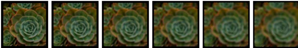
Figure 28: A comparison of different pupil diameters starting at 3mm on the left and increasing to 8mm on the right. In each, the eye has the same defocus error of 130mm created by setting the focal plane at 380mm away while the display is 250mm away.
