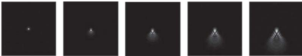
Figure 2: The effect of varying levels of coma aberration shown using the point spread function. The level of coma increases from left to right.
