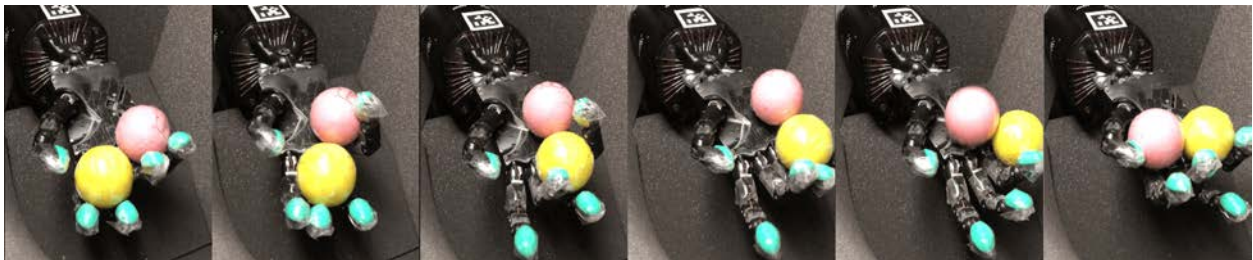
Figure 4.2: PDDM can efficiently and effectively learn complex dexterous manipulation skills in both simulation and the real world. Here, less than 4 hours of experience is needed for the Shadow Hand to learn to rotate two free-floating Baoding balls in the palm, without any prior knowledge of system dynamics.
