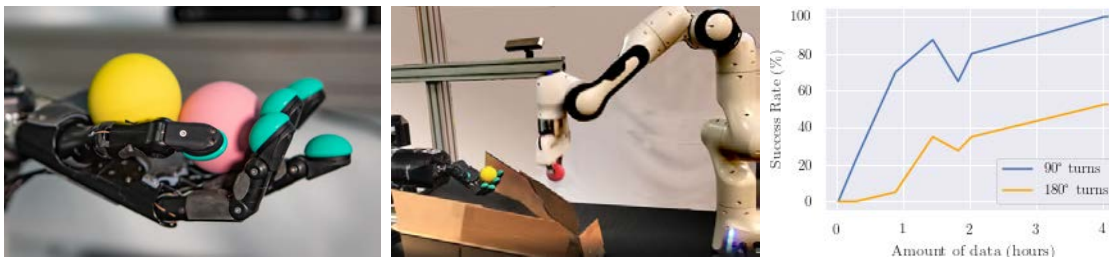
Figure 4.10: Real-world Baoding balls hardware setup with the ShadowHand (left), Franka-Emika arm used for the automated reset mechanism (middle), and the resulting success rates for 90^\circ and 180^\circ turns (right).
