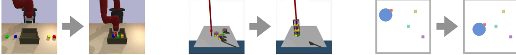
Figure 3: Illustrations of the domains we use for evaluation, in which a policy must (left) control a Sawyer arm to move cubes into and out of a tray (center) attach shelves to a pole using a cursor, and (right) use the blue robot to move objects to different locations. Our tasks requires that the policy ignores objects or move the object based on relative distances, such as moving an object into the tray regardless of the tray’s location.
