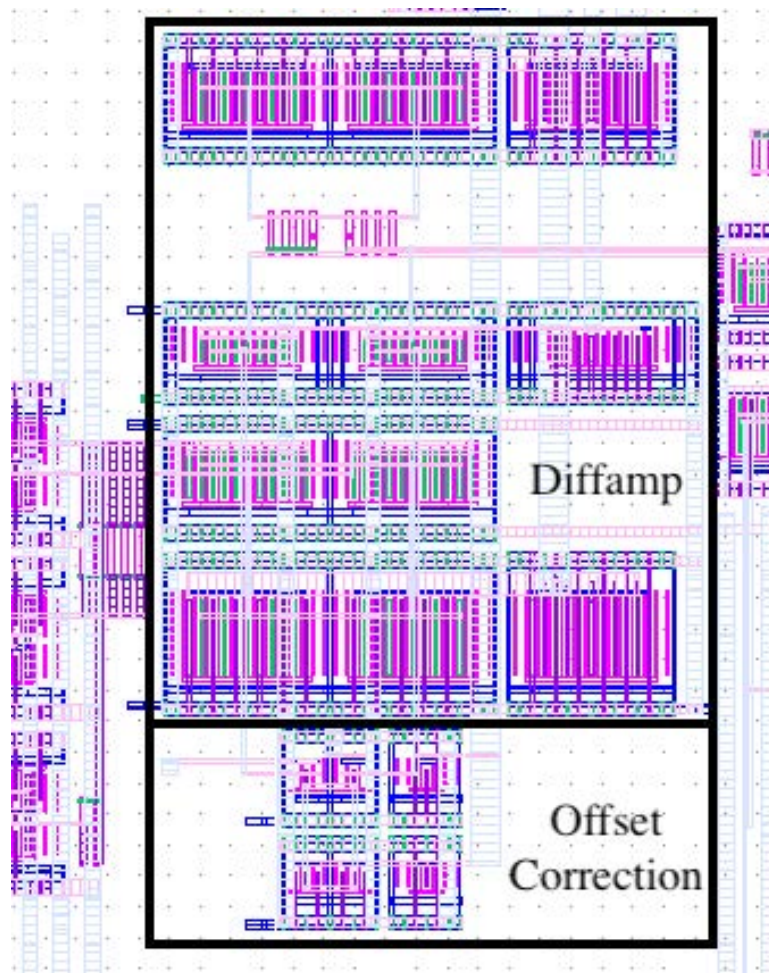
Figure 3.5: Schematic of Pre-Amplifier with Offset Correction
