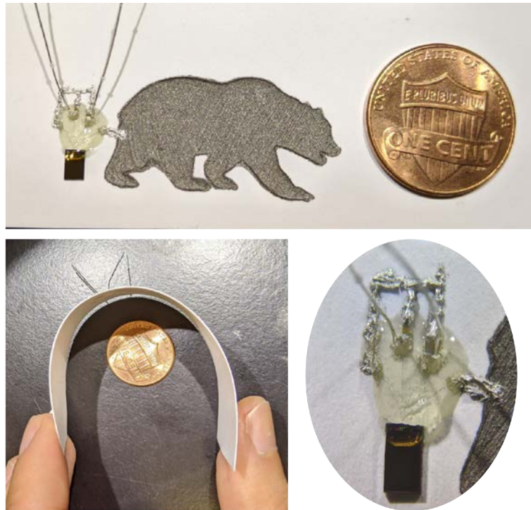
Figure 6.11: Electrostatic energy harvesting system on paper. The ASIC is assembled directly on paper maintaining its flexible and lightweight qualities. The harvesting system continues to work after bending.
