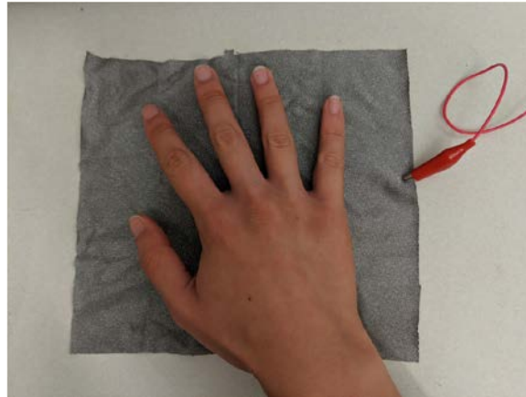
Figure 6.7: Conductive fabric tied to active electrode node on ASIC can operate as a variable capacitor with hand capacitance.
