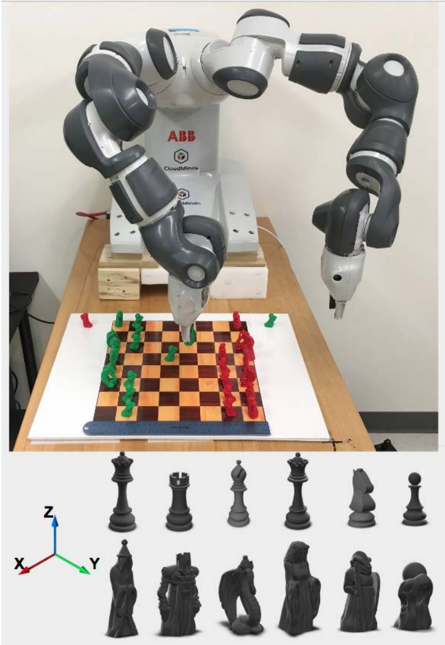
Figure 2.2: Dual-Arm YuMi Robot Playing Non-Standard Chess: (Top) The YuMi robot replaying the classic 1997 chess game where IBM’s Deep Blue defeated world champion Garry Kasparov with asymmetric “wizard” chess pieces (video: https://youtu.be/_LBBX_oxtbA ). (Middle) CAD model of standard chess pieces which can be grasped with hard-coded configurations. (Bottom) CAD model renderings of our non-standard asymmetric chess pieces. The YuMi requires Dex-Net grasp recommendations to manipulate these pieces. The y-axis for each piece points front-to-back, while the x-axis points right-to-left.
