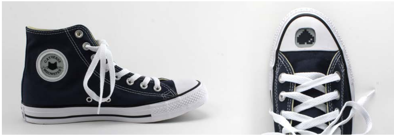
Figure 6.9: Sneaker prototype. Left: Discreet display on the inside heel of the left shoe. Right: Public display on the toe of the right shoe. AlterWear devices are highly contextual. A single artifact can be both personal and public depending on the location of the display.
