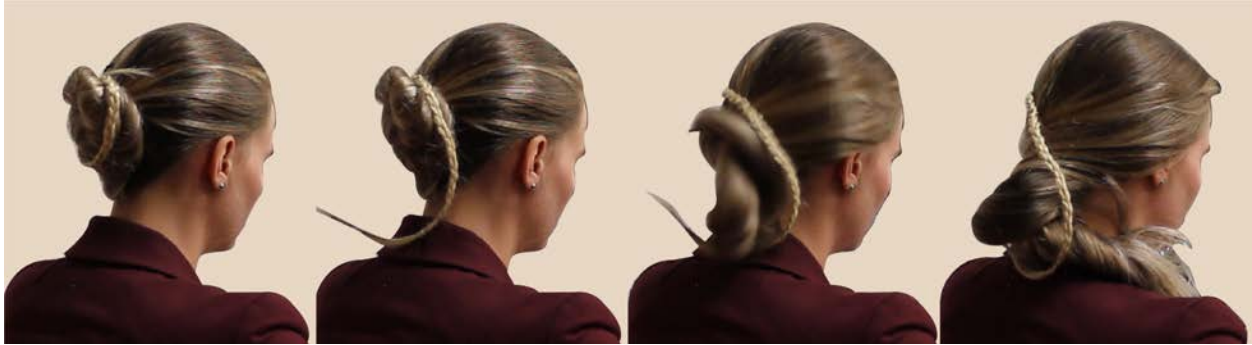
Figure 5.7: Physical implementation of application. H airI  braid is twisted around a bun. Upon actuation, the braid begins to straighten out, unwrapping from the bun and falling on the user’s shoulder. A second wire unravels similarly, and the entire bun falls down. This technique also employs haptics, as the hair movement elicits a tactile sensation.
