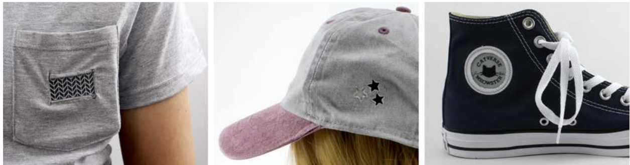
Figure 6.3: Three AlterWear prototypes. Note how well the technology is integrated into the garments. Left: Tee shirt pocket display (i.e., pattern). Middle: Segmented hat display (i.e., stars). Right: Discreet sneaker display (i.e., Catverse logo). AlterWear couples energy harvested from an NFC-enabled device with e-ink displays to afford dynamic interactions and expressions without the need for on-board power.
