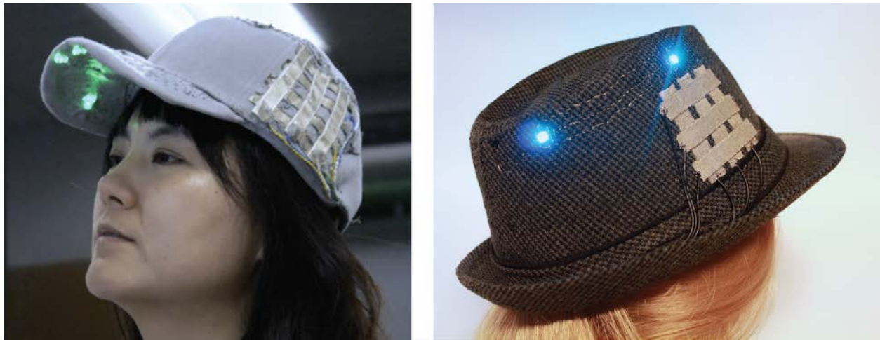
Figure 7.10: The implemented interactive hats included two different classes of ambient displays. Left: personal under-brim display. Right: public crown display.
