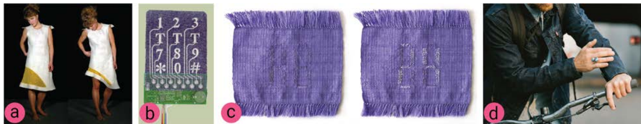
Figure 3.1: E-textiles: (a) Vilkas dress with kinetic nitinol hemline; (b) embroidered fabric keypad with composite image of attached circuit board; (c) Ebb thermochromic textile display; (d) Levi’s ® Commuter X Jacquard By Google trucker jacket 4 .
