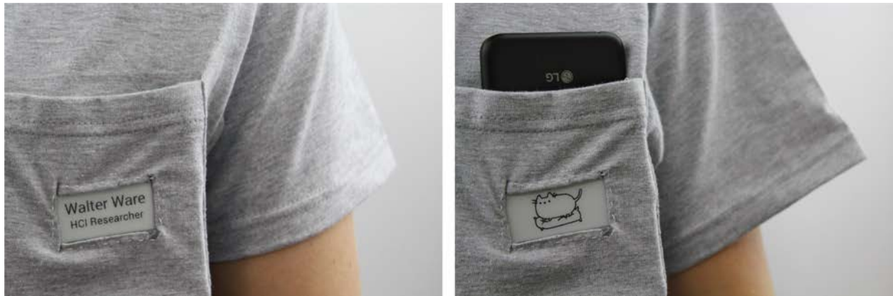
Figure 6.7: Pocket tee prototype. Left: name tag application. Right: when the user places their NFC-enabled phone in their pocket, the phone continuously powers the display, and a simple animation is displayed.
