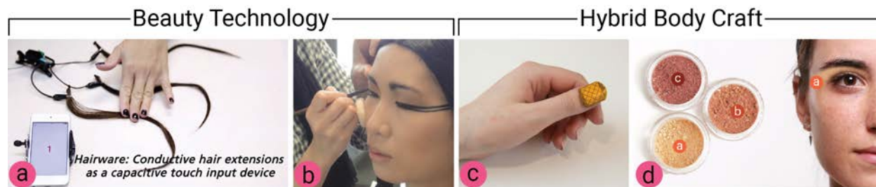
Figure 3.5: Wearable technologies leveraging cosmetic form factors. From left to right: Beauty Technologies in the form of (a) hair extensions and (b) conductive makeups; Hybrid Body Crafts in the form of (c) nail-mounted electronics and (d) cosmetic chemical sensing powders 13 .
