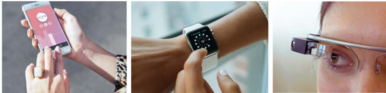
Figure 3.3: Commercially prevalent wearable technologies in the form of accessories. Left: Ringly notification ring; Middle: Apple Watch smartwatch; Right: Google Glass data glasses 10 .
