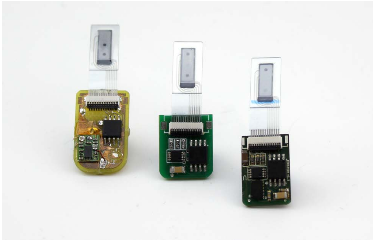
Figure 4.2: Three generations of fingernail devices. All devices are powered wirelessly and feature an e-ink display. From Left to Right: AlterNail, AlterWear, TransformatioNail.
