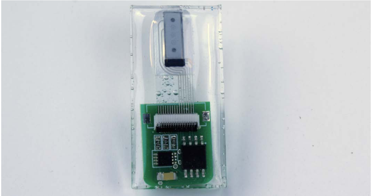
Figure 6.11: To demonstrate durability and longevity of AlterWear devices, the fingernail prototype was completely enclosed in resin. The prototype is durable, waterproof, and still entirely functional.
