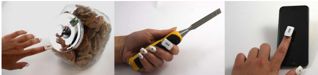
Figure 4.5: Left: Credits and Usage scenario demonstrated with an AlterNail enabled cookie jar. When the user opens the cookie jar, a new dot is added to their AlterNail display. Middle: Object Status scenario demonstrated with an AlterNail enabled chisel. As displayed by the AlterNail, this tool has been used three times today. Right: AlterNail updated through NFC from a smartphone. The user can discreetly check that they have one new email without unlocking and looking at their phone.
