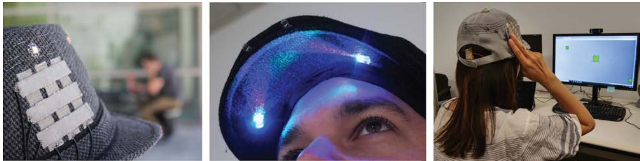
Figure 7.2: Three interactive hat prototypes. Left: touch sensitive region and public crown display of the fedora prototype. Middle: personal under-brim display of the flap cap prototype. Right: user evaluation of the baseball cap prototype.
