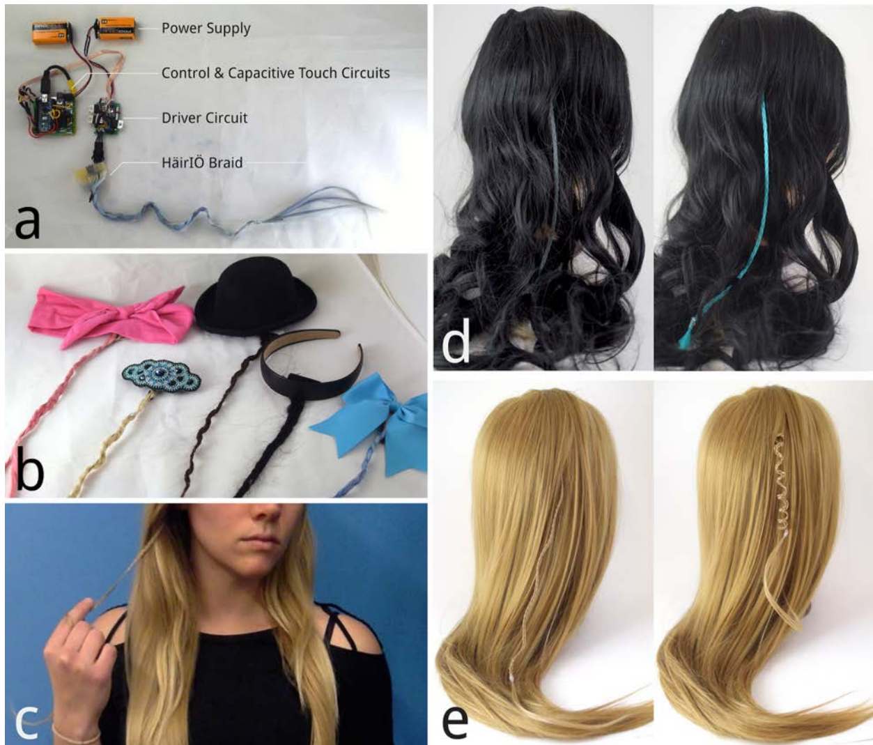
Figure 5.2: A) HäirIÖ prototype prior to miniaturization, B) exemplar HäirIÖ hair accessory form factors, C) HäirIÖ uses Swept Frequency Capacitive Sensing to detect natural hair interactions, D) HäirIÖ color changing properties using thermochromic pigments, and E) shape changing properties using Nitinol wire.
