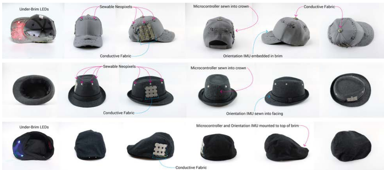
Figure 7.11: Hat prototypes capable of sensing touch and head gestures. The baseball cap (top) has ambient displays under the brim and across the crown; the fedora (middle) has an ambient display across the crown; and the flat cap (bottom) has an ambient display under the brim. In all three prototypes, the battery is tucked into the facing on the inside of the crown.
