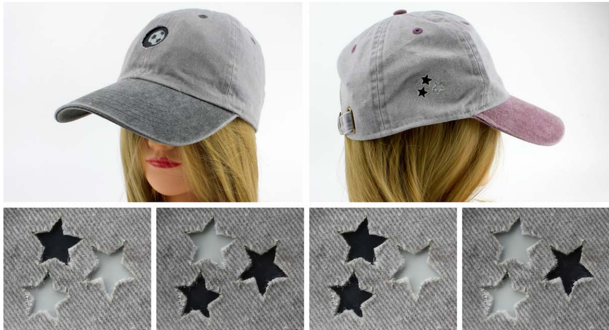
Figure 6.8: Baseball hat prototypes. Left: Hat prototype with AlterWear display on the front panel. Right: Hat prototype with AlterWear display on the side panel. Below: Close up of the side design. This prototype includes a simple animation when updating the display to give the appearance of sparkling or twinkling stars.
