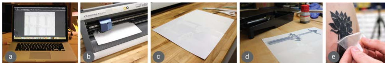
Figure 8.5: The fabrication process for Lotio. a) Design electrode shape and layout interconnects. b) Cut the substrate using commercial vinyl cutter. In this case, the paper tape substrate was applied to waxy paper before cutting. c) Remove excess substrate so that only the design remains. d) Apply electrochromic ink to the cut substrate. e) Transfer resulting design using transfer tape to the skin.
