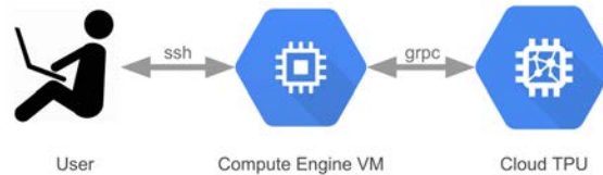
Figure 5.5: This figure illustrates how a regular user can use a cloud TPU. Cloud TPUs are network-attached. Google cloud does not require the user to install any driver. The user can just use the machine images provided by Google cloud.
