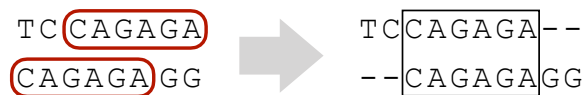
Figure 2.2: The 6-mers shared between two strings on the left are used to seed the alignment of the same two strings on the right.
