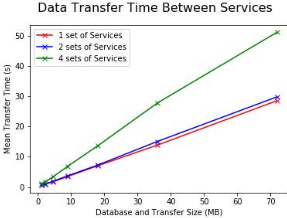
Figure 6.4: Time taken to transfer the entire database contents from a PM to another service in the cluster.
