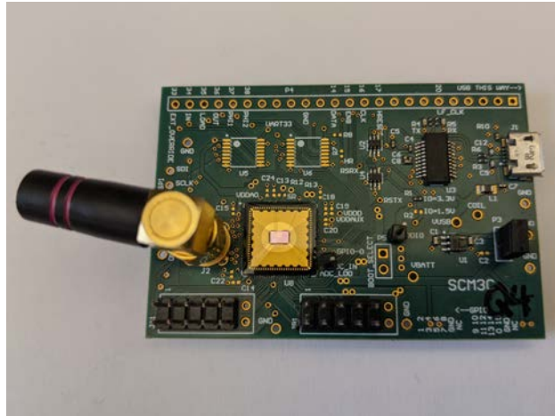
Figure 2.1: Development board Q4 with a wirebonded SC_{\mu}M chip that I used for my experiments.
