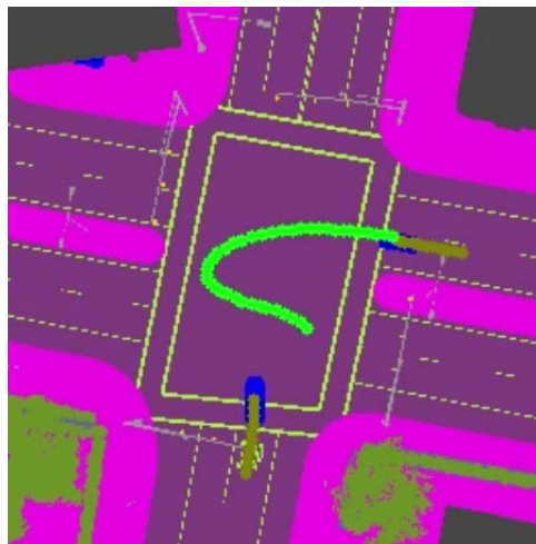
Figure 4.2: Due to our sampling strategy, R2P2 can sometimes be unstable, but this did not affect driving performance as the ego-vehicle has to emergency stop at that distance.
