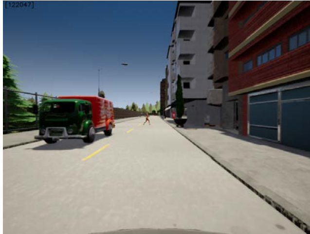
Figure 4.5: The ego-vehicle can choose not to run prediction if no vehicles are physically able to collide with it in the near future, and allocate more time to object detection.
