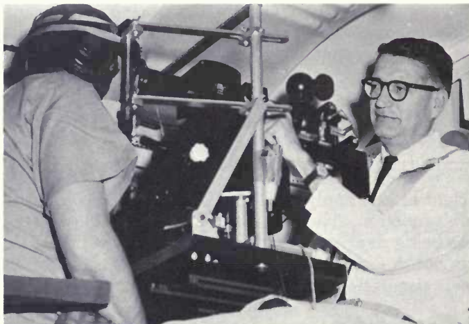
Dr. Duane in the USAF SAM human centrifuge 1968. Zeiss camera modified to photograph the fundus at high Gs.
