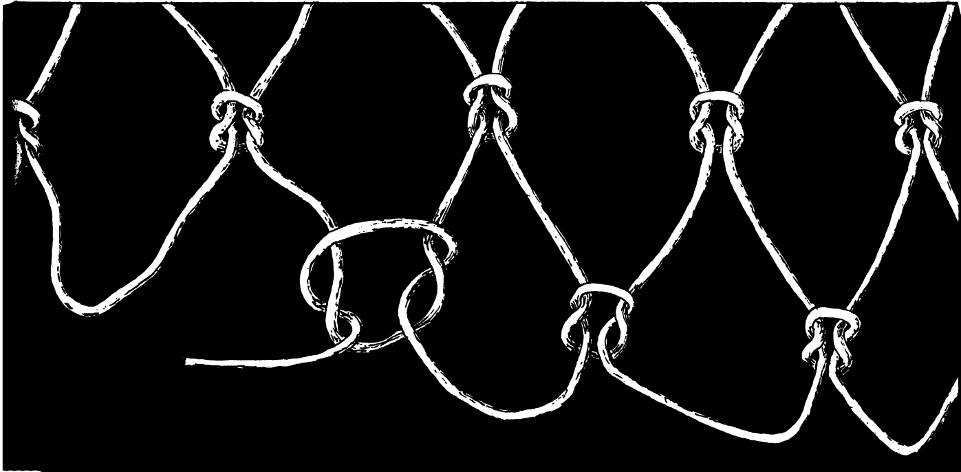
Figure 40. Square-knot netting technique
