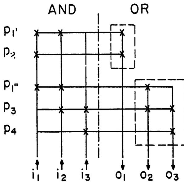
Fig. 4.3c Output-partitioned PLA
