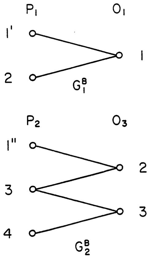
Fig. 4.3b  $G_1^B$  and  $G_2^B$  of the output-partitioned PLA
