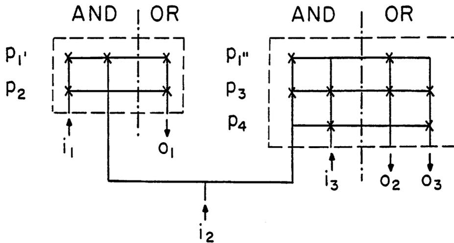
Fig. 4.4b Parallel-partitioned PLA (with product augmentation)
