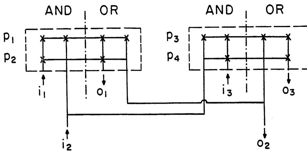
Fig. 4.5b Parallel-partitioned PLA (without product augmentation)
