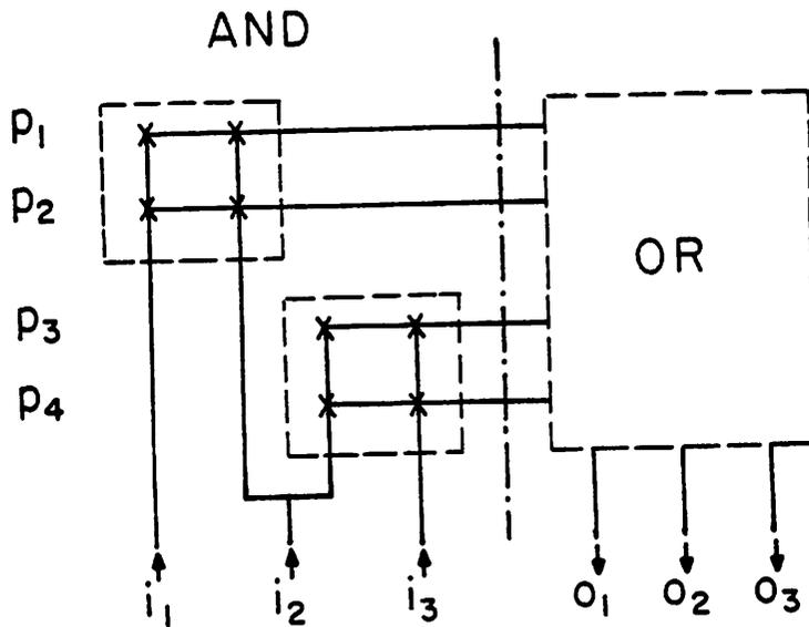
Fig. 4.2c Input-partitioned PLA
