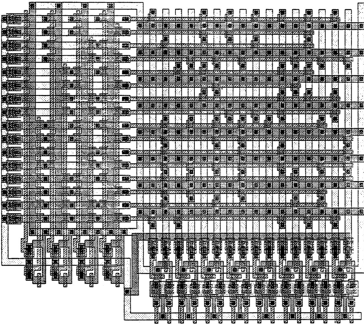
Fig. 6.2a Checkplot of a benchmark PLA (PLA 2) before partitioning
