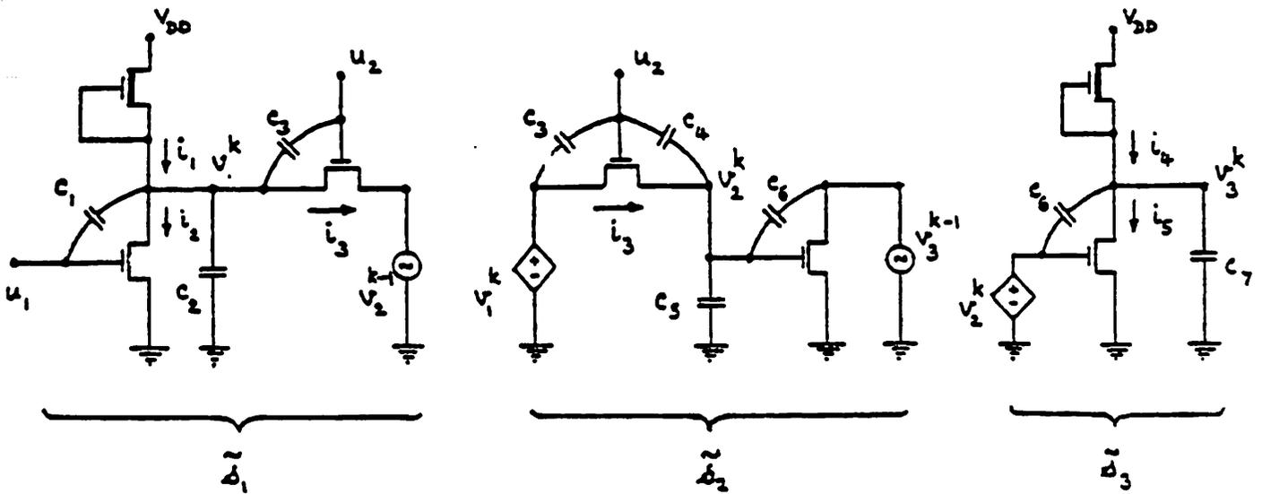
Fig. 2.2 The resulting decomposition of the circuit in Fig. 2.1 at the k-th iteration of the WRM procedure.
