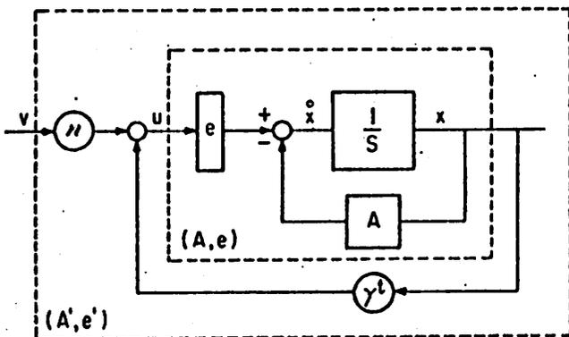
Figure 1. Feedback equivalence of  $(A, e)$  and  $(A', e')$ .
