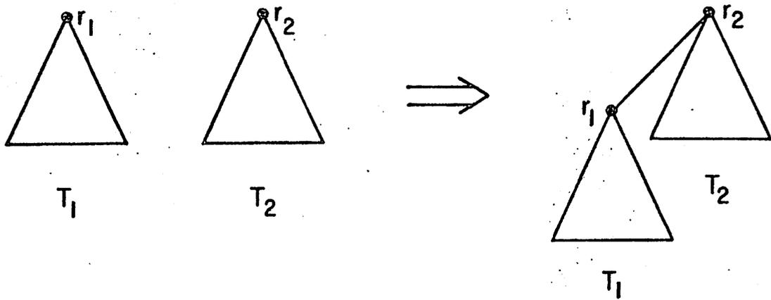
Figure 2: Union of two trees. Root  $r_1$  of  $T_1$  has  $a$  descendants; root  $r_2$  of  $T_2$  has  $b$  descendants. Root of new tree has  $a + b$  descendants.
