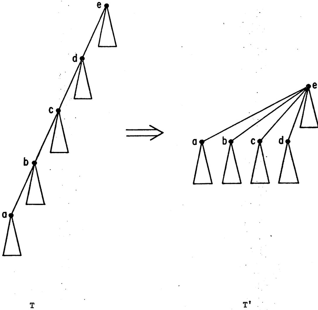
Figure 1: A FIND on element a, with collapsing. Triangles denote subtrees. Collapsing converts tree T into tree T'.
