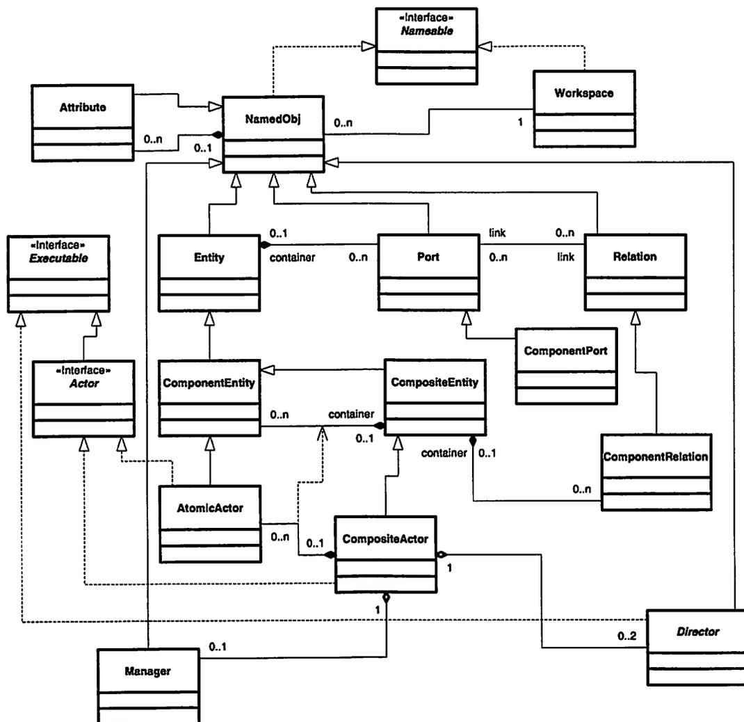
FIGURE 3. Some of the key classes in Ptolemy II. These are defined in the *kernel*, *kernel.util*, and *actor* packages.
