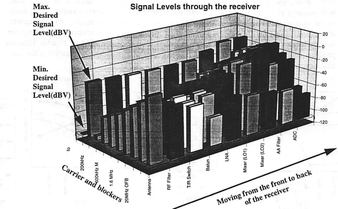
FIGURE 34. All the GSM signal levels in the receiver chain including both inband and out-of-band blockers.
