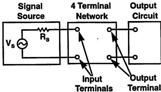
FIGURE 14. Simple Four terminal Network
