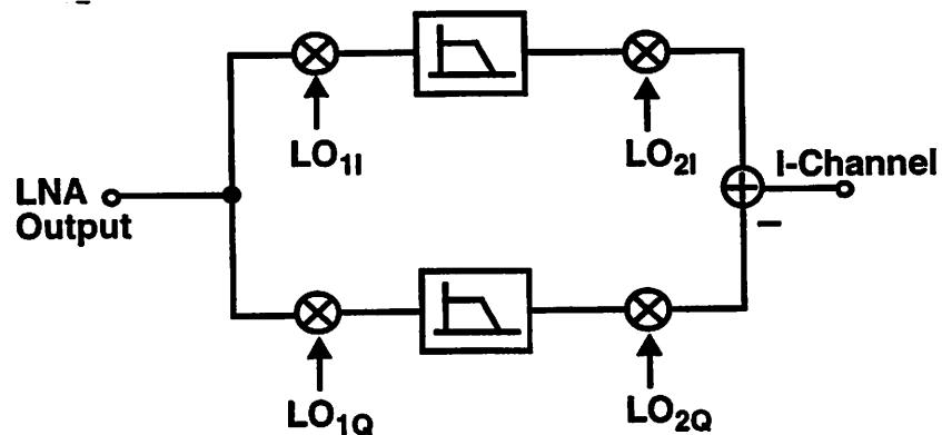
FIGURE 25. Single channel IR-Mixer used by the wideband IF receiver
