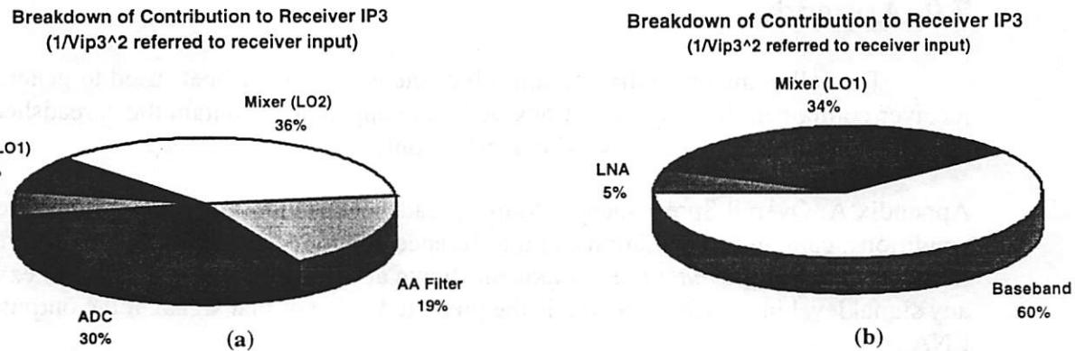
FIGURE 38. Individual contribution of each block to the overall receiver's input referred IP3. The breakdown is with respect to each receiver block's  $V_{IP3}$  referred to the receiver input, (a) Wideband IF (b) Low-IF w/ single conversion
