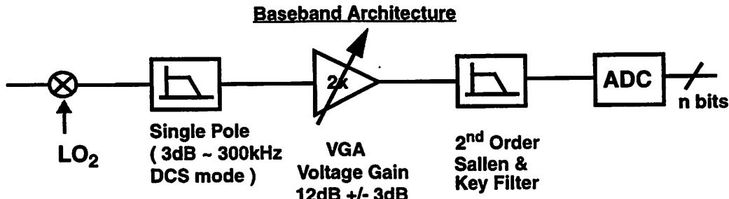
**FIGURE 29.** Baseband filter and ADC configuration.
