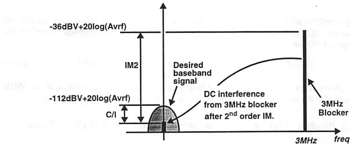
FIGURE 20. Signal spectrum after the second mixer in the wideband IF receiver during the GSM 3MHz blocking test. An interferer is created within the signal band by the 3MHz blocker passing through the baseband 2<sup>nd</sup> order nonlinearities.
