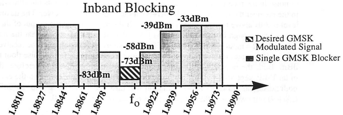
FIGURE 7. DECT Inband blocking requirements
