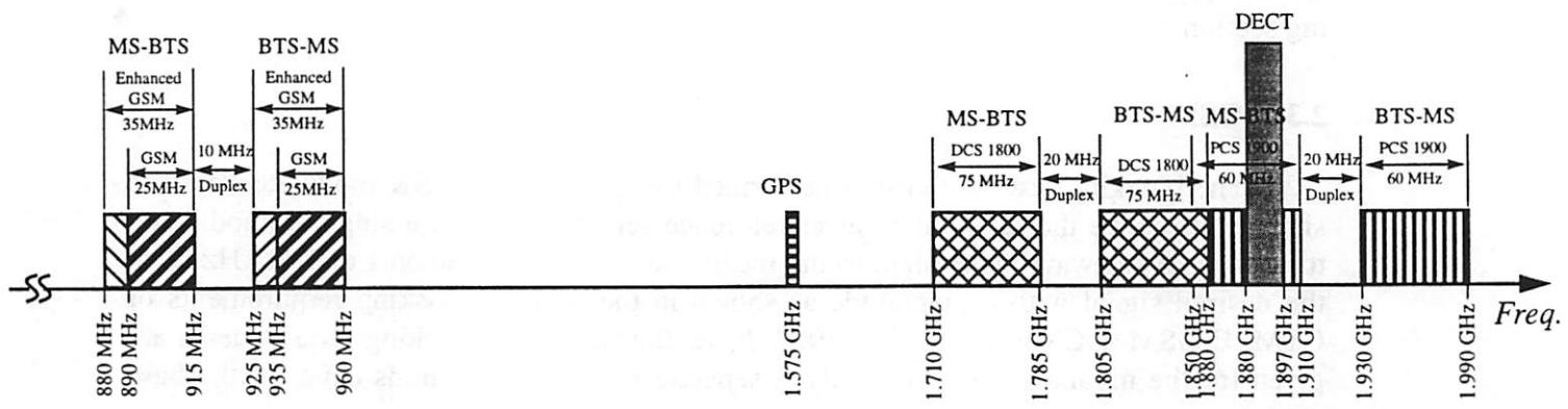
**FIGURE 1. Frequency Bands of interest for the (GSM / DECT / GPS) Receiver.**
