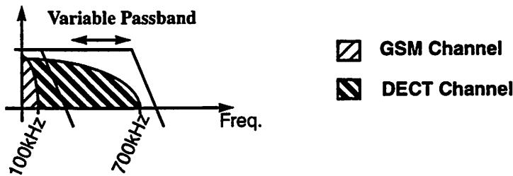
FIGURE 28. Bandwidth channel filtering requirements for dual-standard operation. Both the DECT and GSM channel are frequency translated to baseband.
