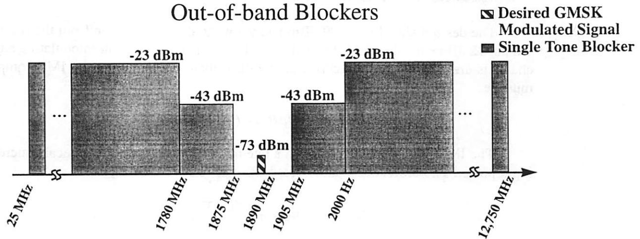
FIGURE 9. Out-of-Band DECT blocking requirements.
