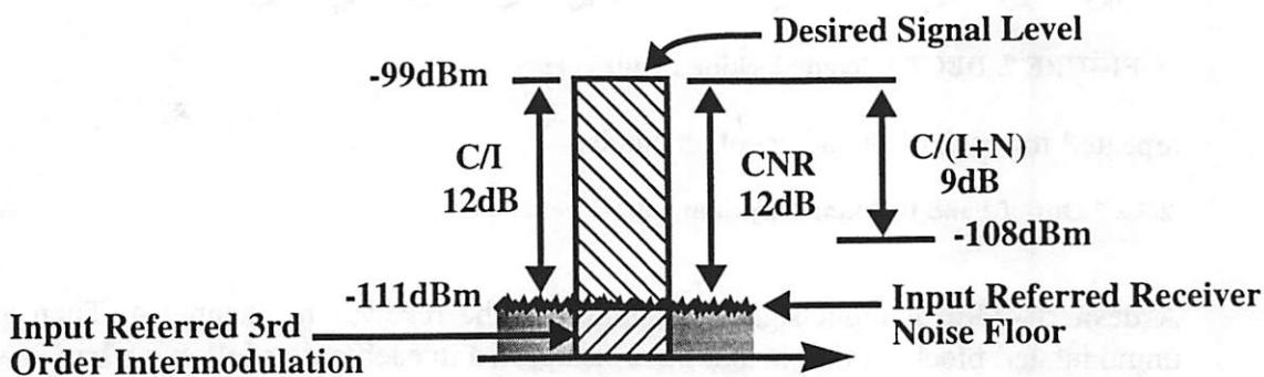
FIGURE 10. Maximum allowable input referred noise and distortion floors under the intermodulation test for GSM, PCS 1900.
