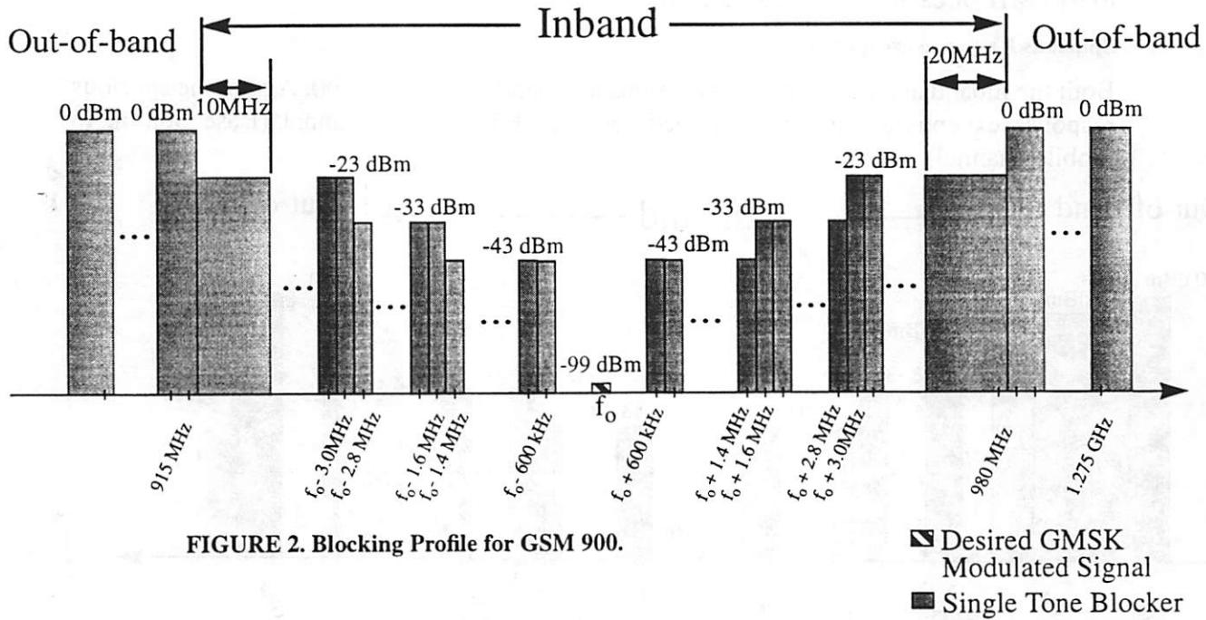
FIGURE 2. Blocking Profile for GSM 900.
