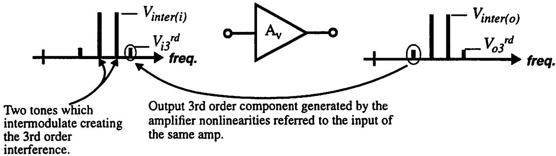
**FIGURE 18. Representation of the adjacent channel interferers and the intermodulated 3rd order component which is created.**
