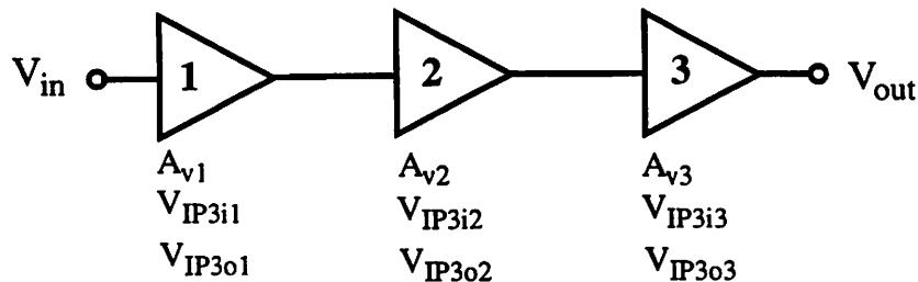
**FIGURE 19. Intermodulation in a set of cascaded blocks.**
