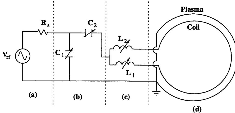
Figure 2: The circuit schematic of the system, with the tuning network shown to launch a traveling wave along the antenna coil.  $L_1$  and  $L_2$  are two identical variable inductors. (a) RF power generator; (b) matching network; (c) tuning network; (d) antenna coil.
