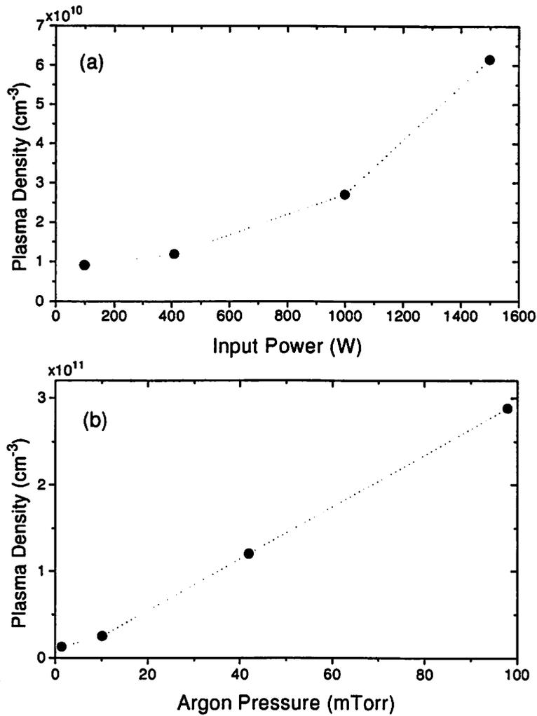
Figure 4: Langmuir probe measurement of (a) plasma density vs. input power at 1.4 mTorr argon pressure and (b) plasma density vs. argon pressure at 500 W input power.
