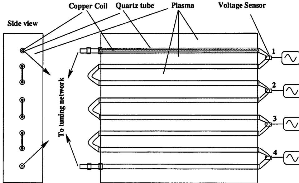
**Figure 1: Antenna coil system. The coil is made of a series of copper tubes, each surrounded by a quartz tube embedded in the plasma. Four voltage sensors are equally spaced along the antenna coil to monitor the voltage distribution.**
