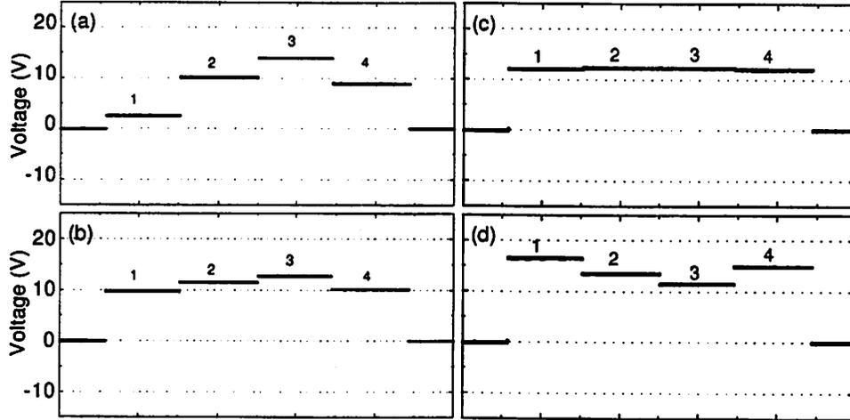
Figure 3: Oscilloscope traces showing the voltages on the four sensors. Each segment of the signal comes from one voltage sensor. (a) Voltages from the four sensors are very different, indicating a high standing wave ratio along the coil; (b) as the tuning network is adjusted, the voltage signals become comparable; (c) voltages from the four sensors are equal, indicating that a traveling wave has been launched; (d) over tuned condition.
