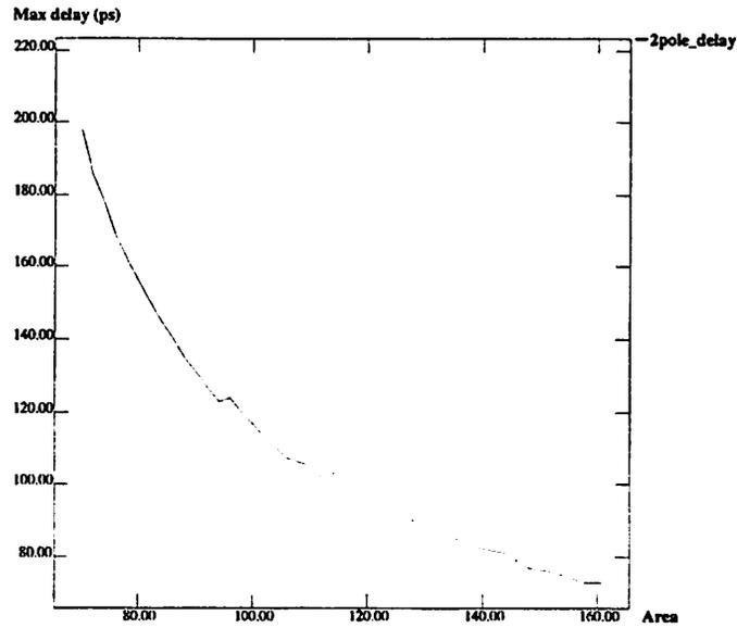
Figure 3.8: Maximum Delay vs. Routing Area
