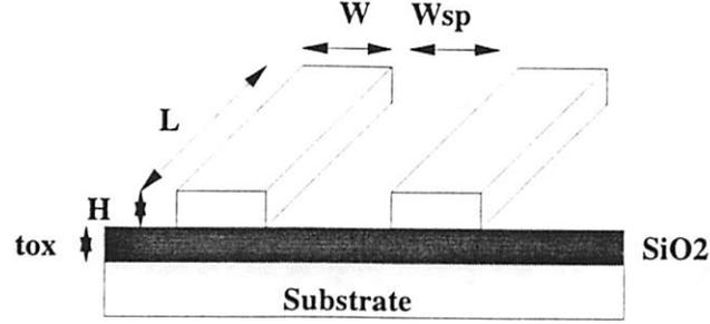
Figure 1.3: Modeling of Interconnects on the Chip
