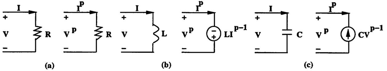
Figure 3.1: Moment Models of Lumped Circuit Elements
