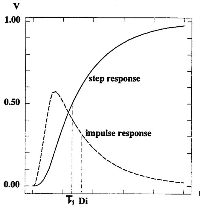
Figure 2.5: Step and Impulse Response at Node  $i$
