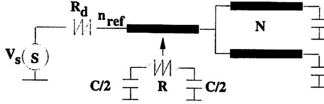
Figure 2.4: Formulation of Distributed RC Line Network  $N$
