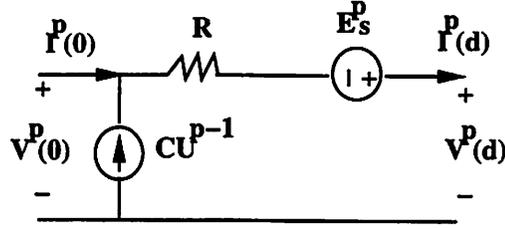
Figure 3.2: Moment Model of Lossy Transmission Line
