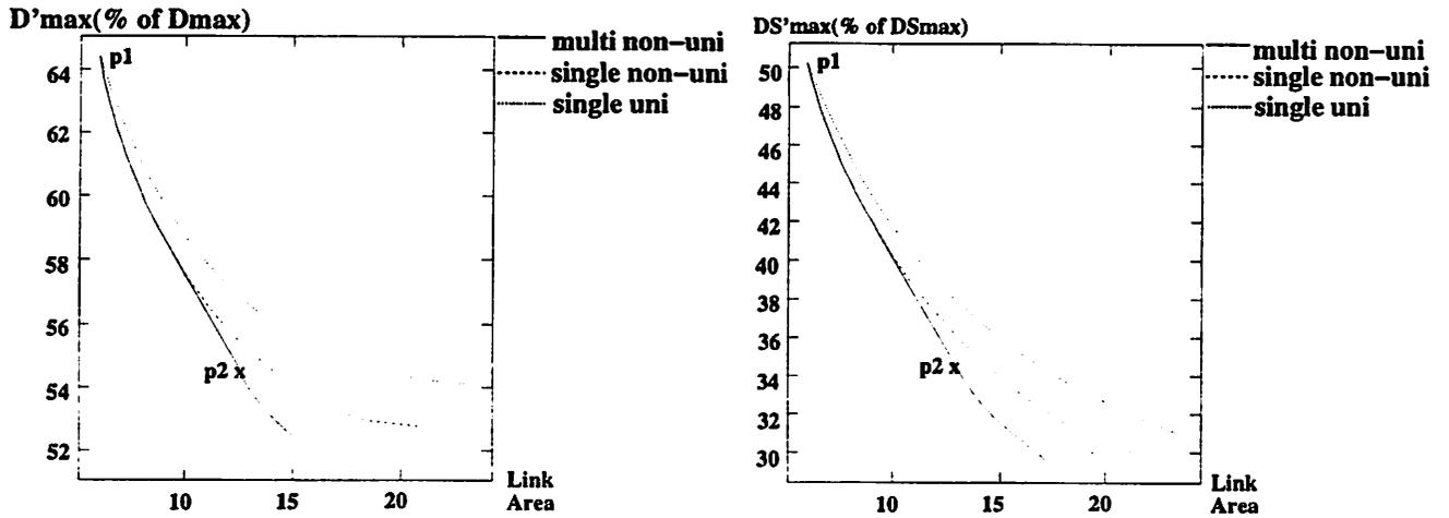
Figure 2.13: (a) Maximum delay vs. Link area (b) Maximum skew vs. Link area
