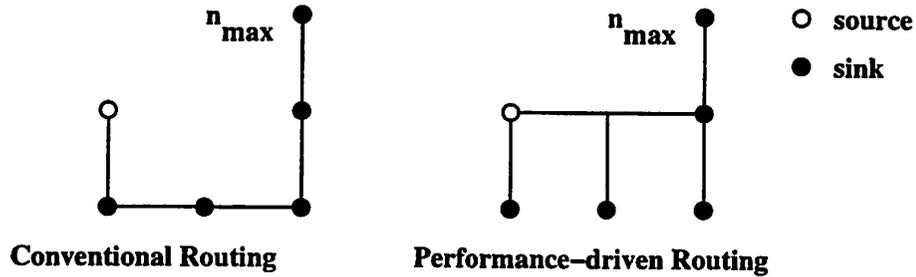
Figure 1.4: Conventional vs. Performance-driven Routing
