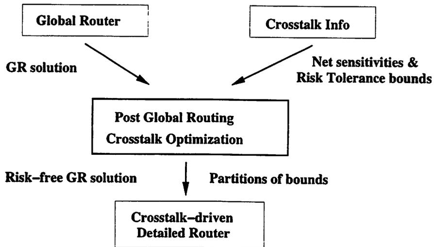
Figure 4.3: Post Global Routing Crosstalk Estimation and Reduction
