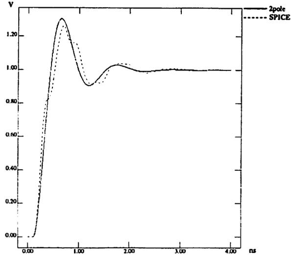
Figure 3.5: Waveforms at Maximum Delay Node Before Optimization
