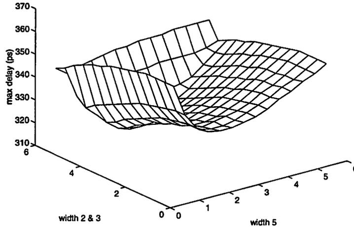
Figure 3.3: Example: Maximum Delay vs. Wire Widths
