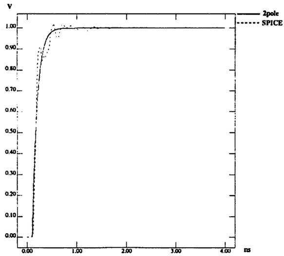
Figure 3.6: Waveforms at Maximum Delay Node After Optimization
