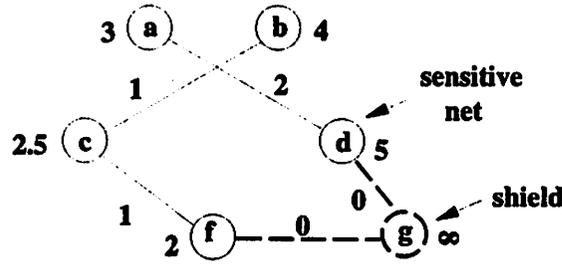
Figure 4.8: Construction of Hamiltonian path using shield
