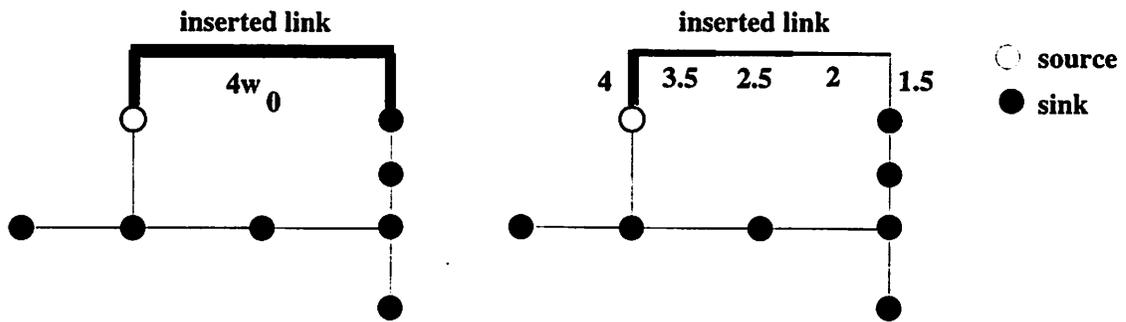
Figure 2.11: Single link: (a) Uniform Sizing (b) Non-Uniform sizing
