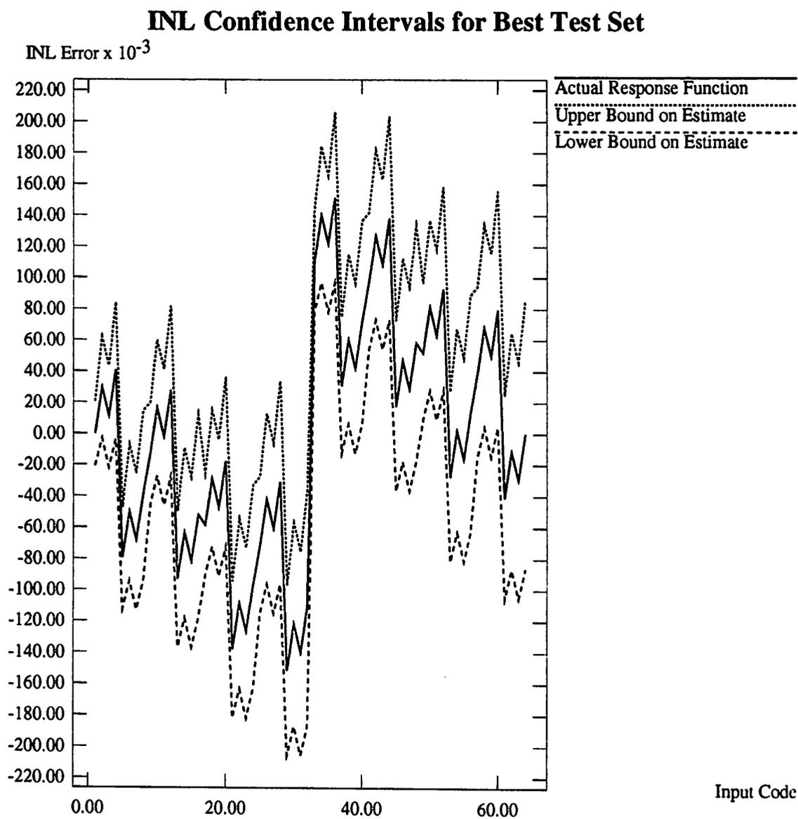
Figure 3.5: Upper and lower bounds on INL error from seven test vectors.
