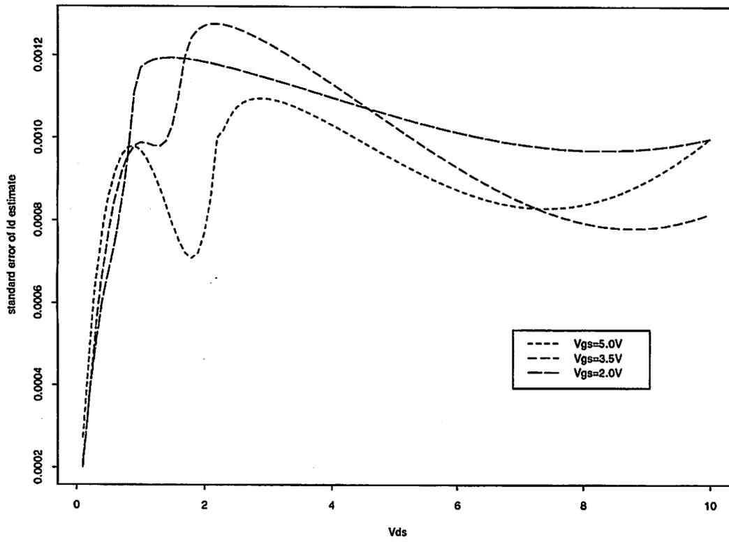
Figure 4.8: Standard error of estimated response for MOS transistor.
