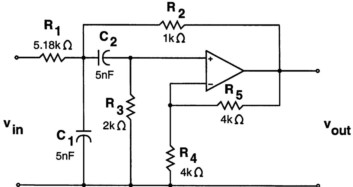
Figure 4.2: Bandpass filter with center frequency at 24.5 kHz.
