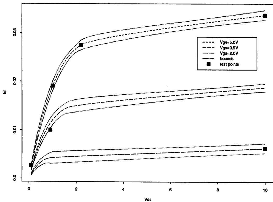
Figure 4.7: Estimated response and confidence intervals for MOS transistor from 6 test points.
