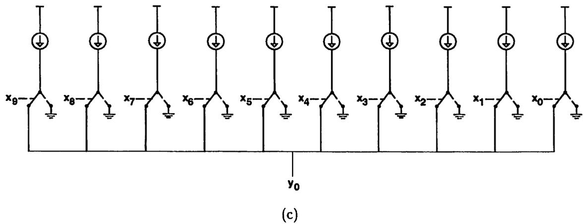
Figure 5.2: (a) Proposed test structure for Circuit 1. (b) Proposed test structure for Circuit 2. (c) Proposed test structure for Circuit 3.
