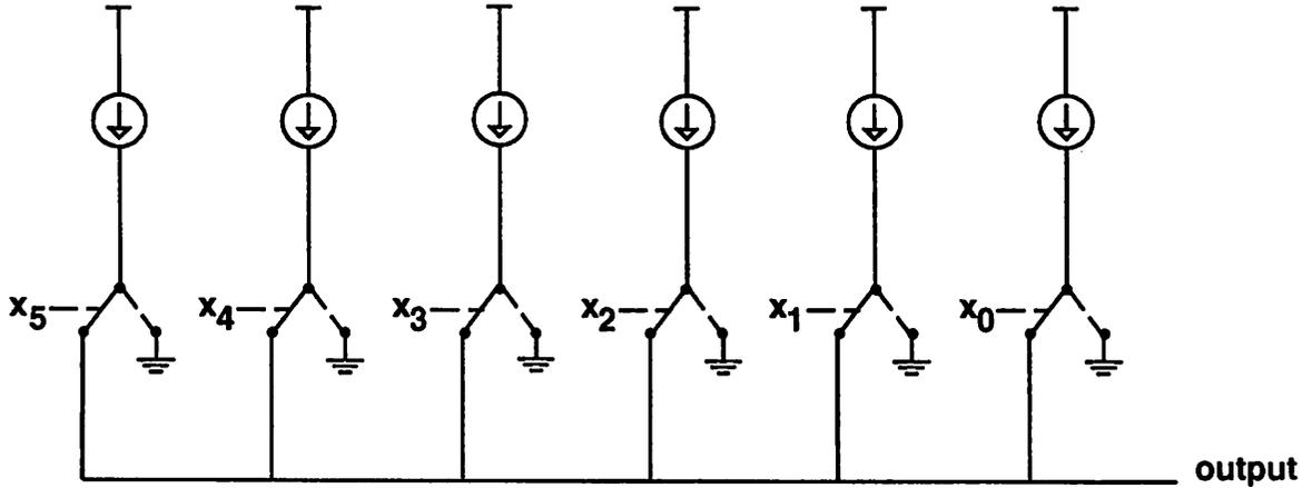
Figure 3.1: Six switchable current sources connected in parallel.
