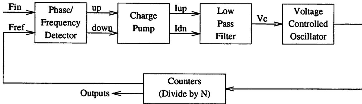
Figure 6.5: Block diagram of PLL.
