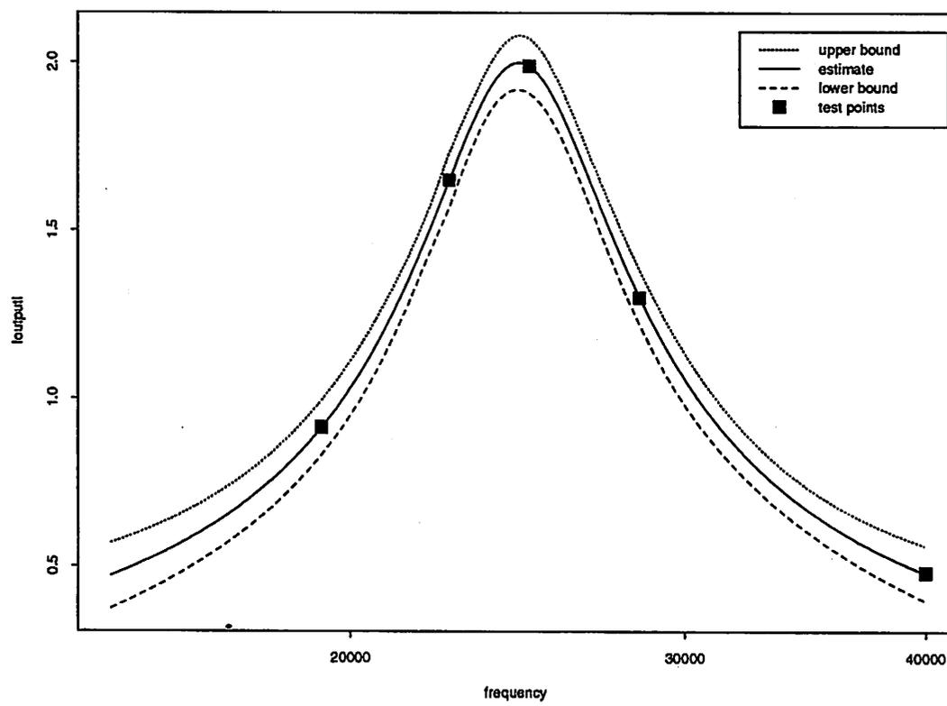
Figure 4.4: Estimated output and 99% confidence intervals for bandpass filter.
