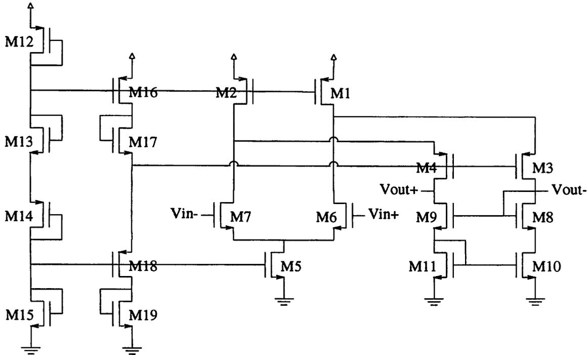
Figure 6.4: Transistor-level schematic of operational amplifier circuit.
