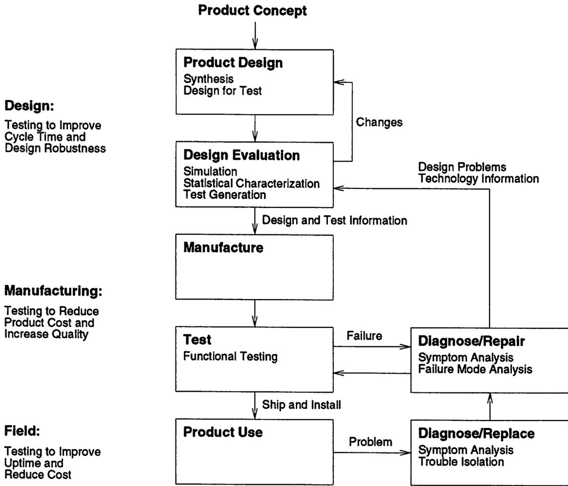
Figure 1.1: Overview of testing within typical product design cycle.
