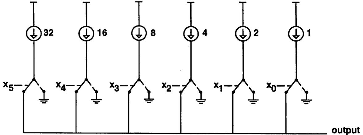
Figure 3.4: 6-bit binary-weighted current source D/A converter.
