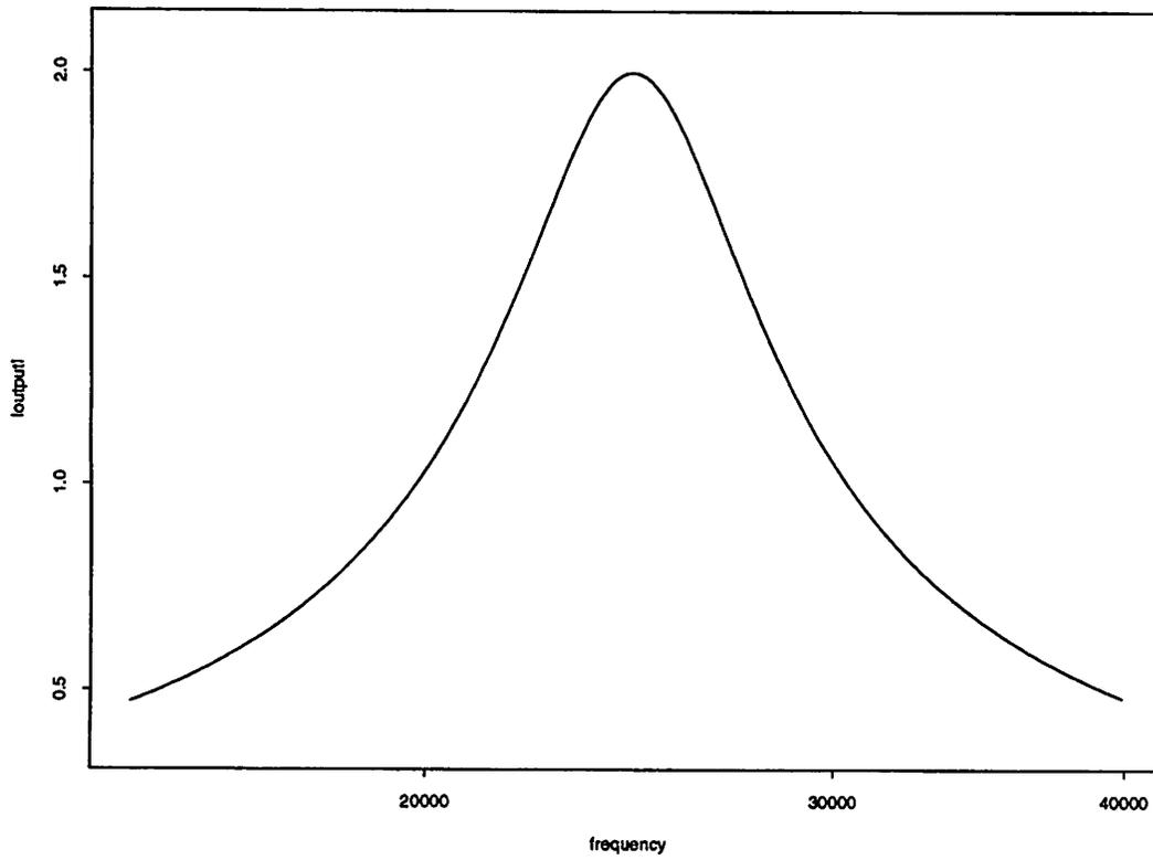
Figure 4.3: Nominal frequency response of bandpass filter.
