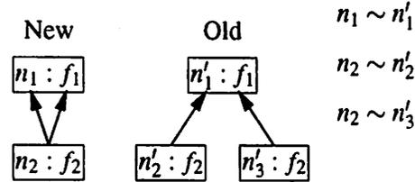
Figure 7: A candidate pair ( $n_1 \sim n'_1$ ) with no consistent matching.
