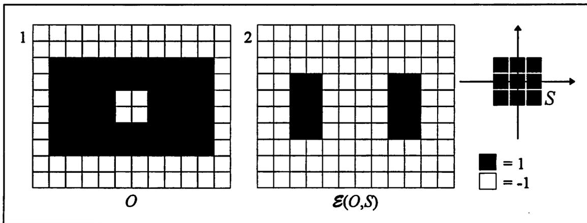
Figure 8. Binary erosion  $\mathcal{E}(O,S)$  of an image  $O$  by a square structuring element  $S$ . Picture 1 shows the original image  $O$ . Picture 2 depicts the result of the binary erosion of
