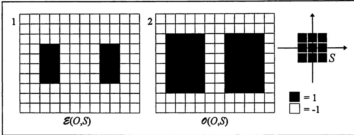
Figure 9. Binary opening  $\theta(O,S)$  of an image  $O$  by a square structuring element  $S$ . Picture 1 shows the eroded original image  $\mathcal{E}(O,S)$ . Picture 2 illustrates the result of the binary dilation of  $\mathcal{E}(O,S)$  by  $S$  which equals the binary opening  $\theta(O,S)$ .
