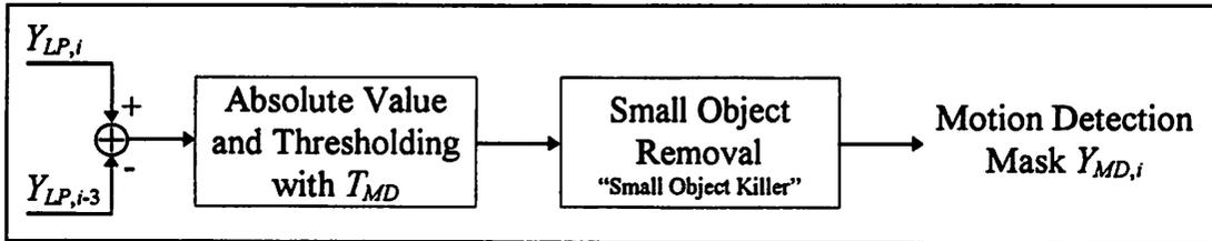
Figure 5. *Motion Detection* is done by computing the pixelwise difference of two incoming frames. The significant motion is extracted by a thresholding operation and an elimination of small detected moving areas that are mostly due to noise influences. The output is a binary mask where moving parts are marked in black.
