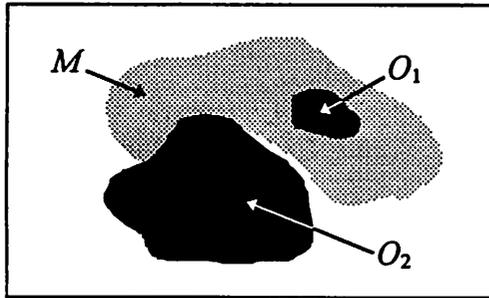
Figure 13. The marker  $M$  (for presentation purposes given in gray) marks only object  $O_1$  but not object  $O_2$ . This results from the simple observation that  $O_1$  is completely contained in  $M$ , while parts of  $O_2$  do not coincide with  $M$ . In terms of mathematical set theory this means that  $O_1 \in M$ , but  $O_2 \notin M$ .
