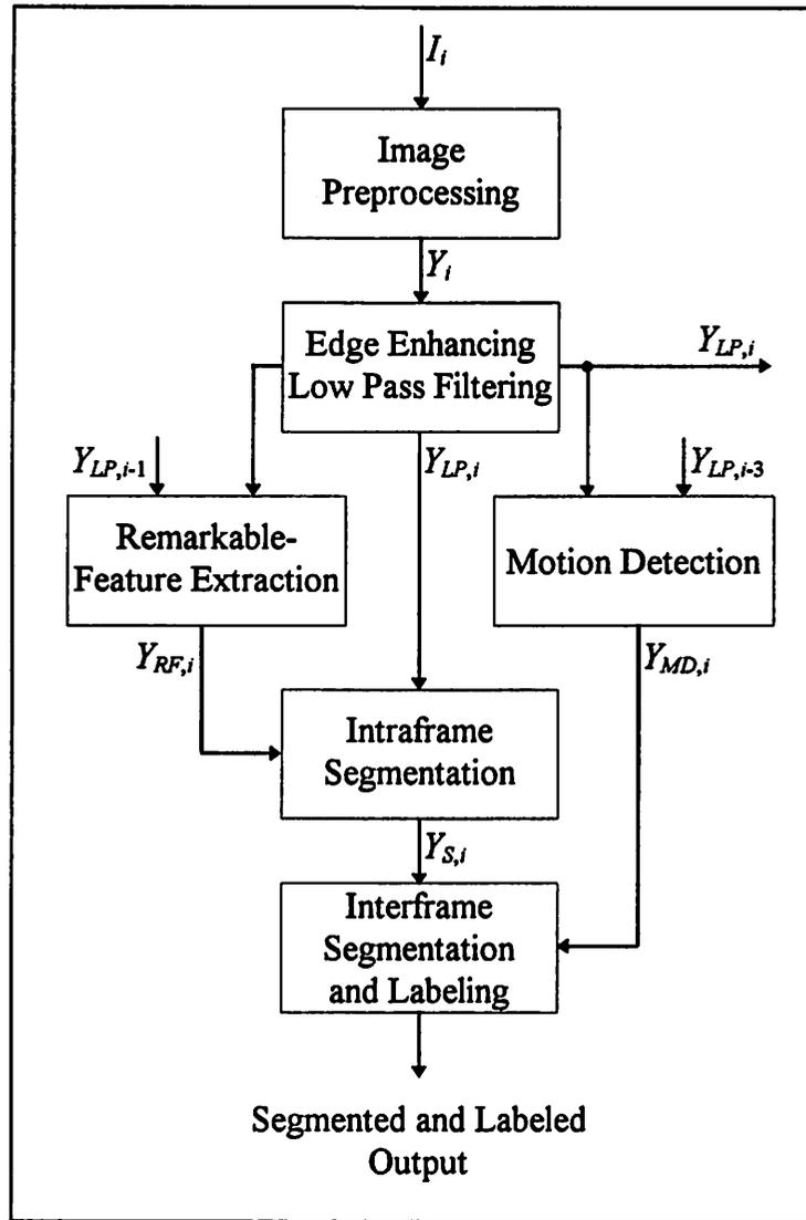
Figure 2. Block diagram illustrating the structure of the *Segmentation and Object Labeling* algorithm. This is the first block of the image analysis described in Figure 1. One can imagine the same architecture for the processing of all image frames. At certain levels these architectures interact mutually and exchange their low pass filtered intermediate results, this is  $Y_{LP,i}$ ,  $Y_{LP,i-1}$ , and  $Y_{LP,i-3}$ , as it is demonstrated in this figure.
