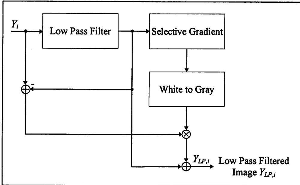
Figure 4. The *Edge Enhancing Low Pass Filtering* stage is intended to reduce the incoming image's noise with a special low pass filter operation. In order to maintain the sharpness of the scene's contours, an additional edge enhancement restores the most important features, this is the moving contours.
