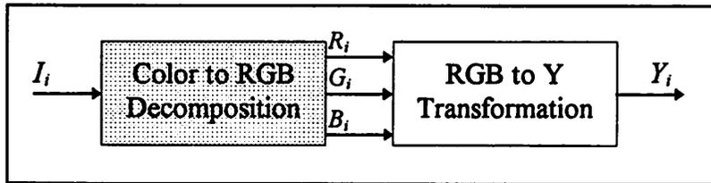
Figure 3. *Image Preprocessing* decomposes the color frames into the YIQ system and extracts the  $Y$  channel. The incoming image is first split off into a red  $R_i$ , green  $G_i$ , and blue  $B_i$  channel, commonly reported as the RGB system. This decomposition is usually
