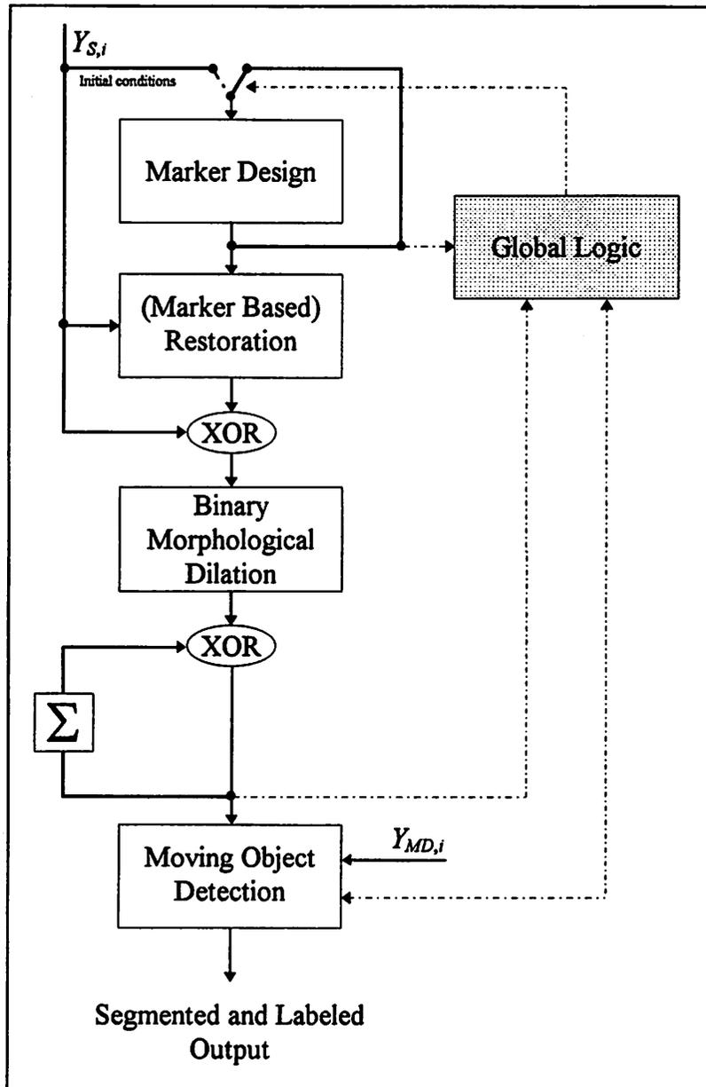
Figure 12. The *Interframe Segmentation and Object Labeling* operation sorts the fragments detected by the *Intraframe Segmentation* by size and transmits only those, which are also part of the motion detection mask  $Y_{MD,i}$ . This algorithm is based on *markers*, which are areas pointing out the location of segmented image objects. An external logic controls the data flow, such as switching the input of the *Marker Design* block after the initial conditions have been downloaded.
