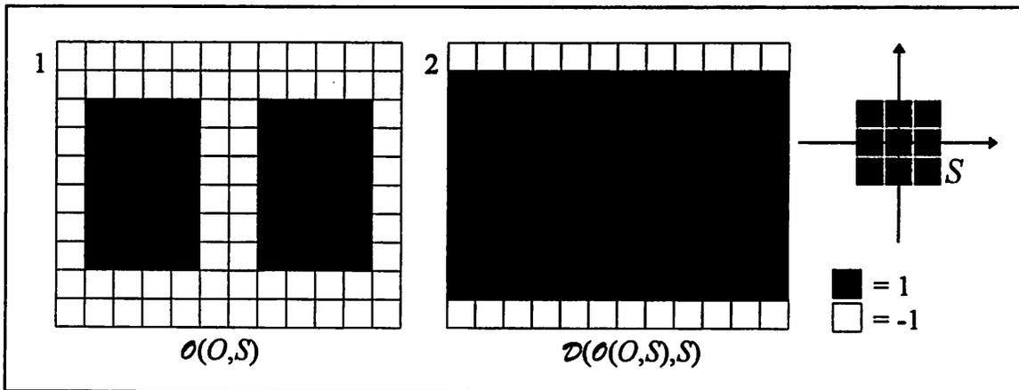
Figure 10. A second binary dilation  $\mathcal{D}(\theta(O,S),S)$  of the opening  $\theta(O,S)$  by a square structuring element  $S$ . Picture 1 shows the original image  $\theta(O,S)$ . Picture 2 depicts the result of the binary dilation of  $\theta(O,S)$  by  $S$ . One can see how a dilation is able to join different features of an image and to fill cracks within an object.
