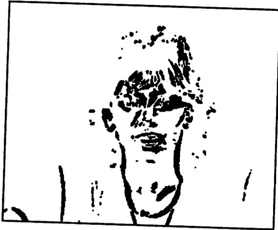
Figure 26. Thresholded abs.  $Y_{LP,i} - Y_{LP,i+1}$  diff..
