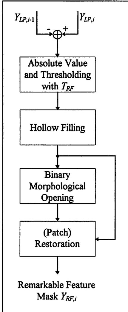
Figure 6. The aim of the *Remarkable-Feature Extraction* function is the detection of image parts fulfilling certain size and motion criteria at the same time. This result is computed by taking the difference of two directly succeeding frames, whose absolute pixel values are then compared to a relatively high threshold. The *Hollow Filling* intends to merge very small objects, such as the eye balls or the teeth, with the surrounding object.
