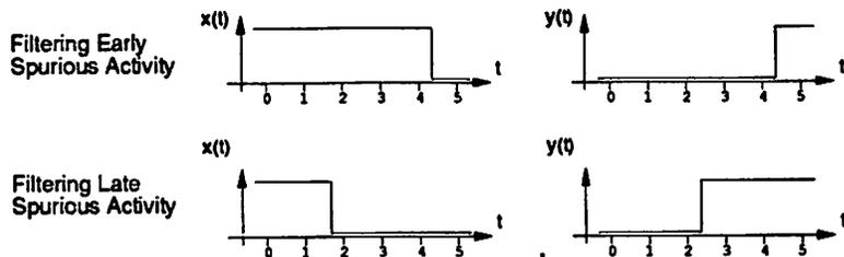
Figure 1.5: Inertial Delay and the Limitations of Timing Model Accuracy
