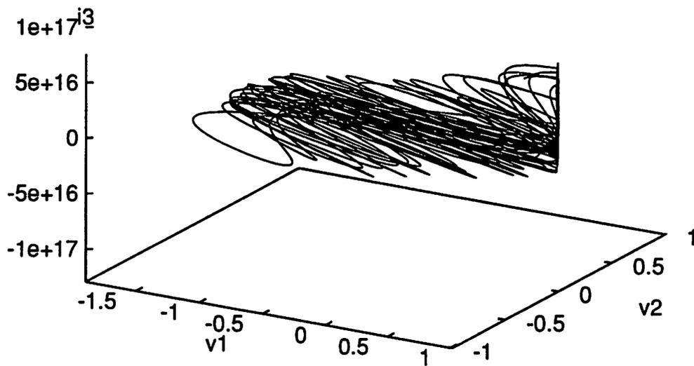
Figure 5: Attractor from the 4-dimensional Chua's oscillator which is topologically conjugate to the system in Eq. (52) with parameters  $\gamma_L = 0.5$ ,  $\gamma_C = 0.5$ ,  $\alpha = 0.18$ ,  $\epsilon = 0.005$ . The attractor is projected onto the  $v_1$ - $v_2$ - $i_3$  plane.
