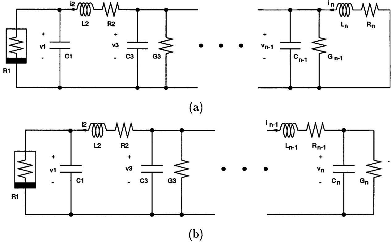
Figure 14:  $n$ -dimensional circuit given in [Kocarev *et al.*, 1993]. (a)  $n$  is even. (b)  $n$  is odd.
