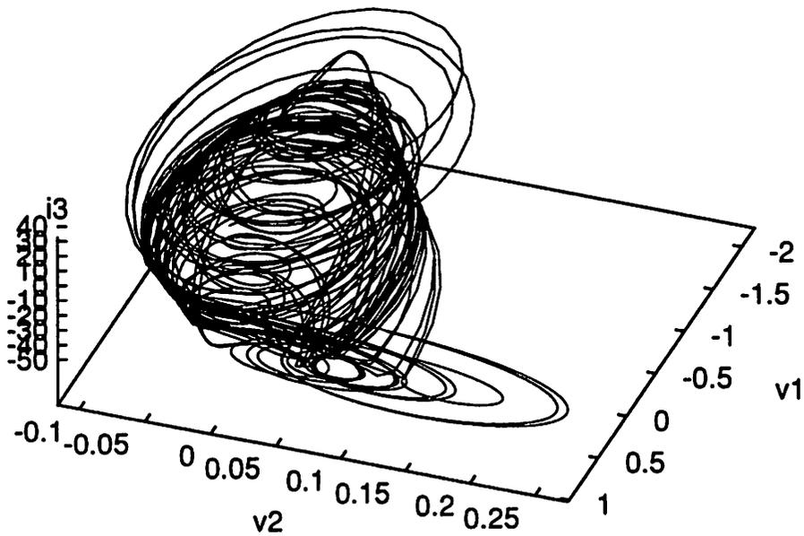
Figure 6: Attractor from the 4-dimensional Chua's oscillator which is topologically conjugate to the system in Eq. (53) with parameters  $\gamma_L = 1$ ,  $\gamma_C = 1.545$ ,  $\alpha = 0.26$ ,  $\epsilon = 0.005$ . The attractor is projected onto the  $v_1$ - $v_2$ - $i_3$  plane.
