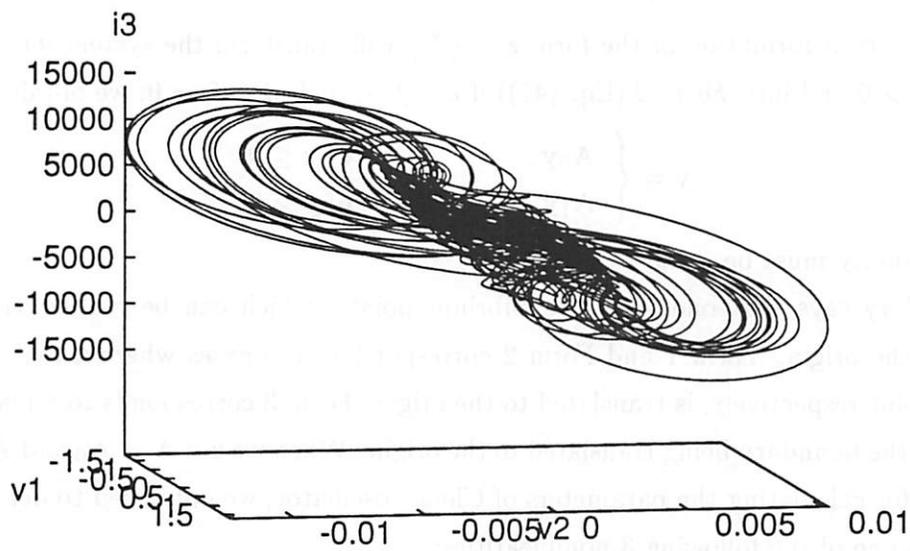
Figure 4: Attractor from the 4-dimensional Chua's oscillator which is topologically conjugate to the system in Eq. (44) with parameters  $C_1 = \frac{1}{2}$ ,  $C_2 = \frac{1}{20}$ ,  $L_3 = 1$ ,  $L_4 = \frac{2}{3}$ ,  $R = 1$ ,  $m_0 = -0.2$  and  $m_1 = 3$ . The attractor is projected onto the  $v_1$ - $v_2$ - $i_3$  plane.
