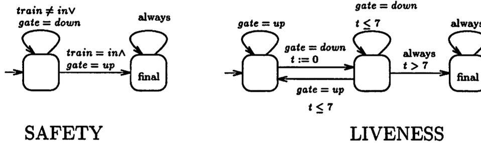
Figure 4.2: Properties for the railroad crossing example.
