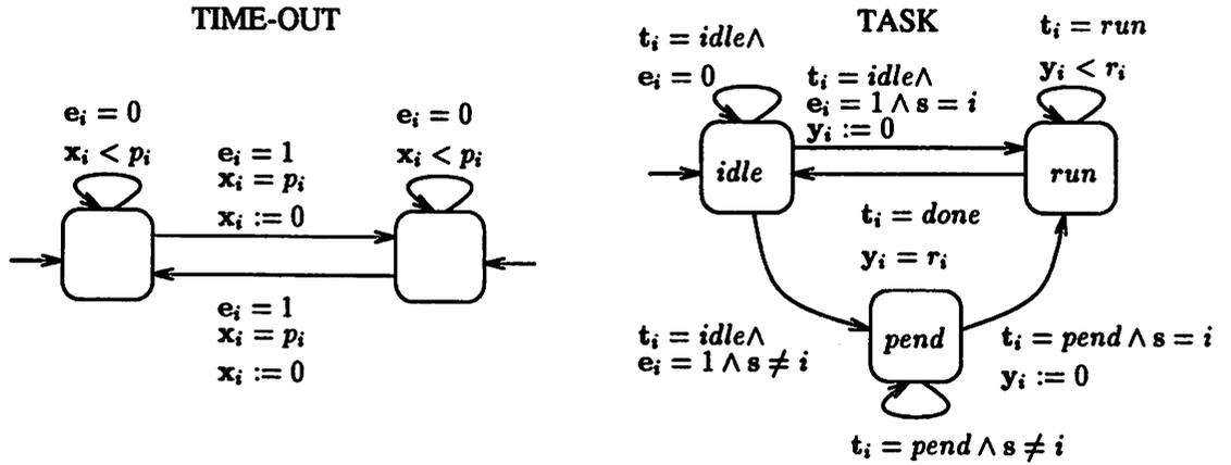
Figure 5.1: Simple models of a time-out and a task.
