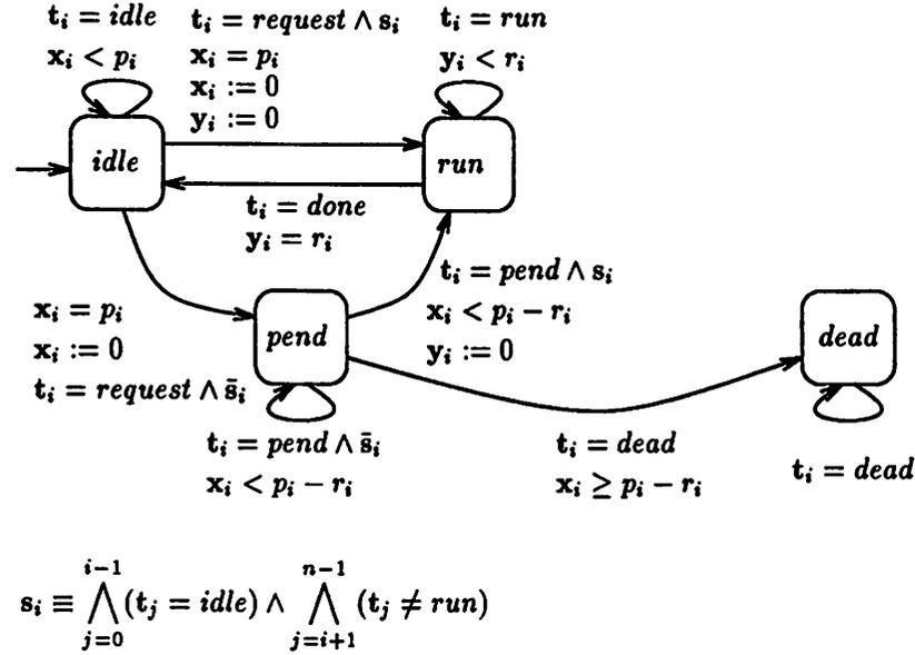
Figure 5.2: An optimized model of a task.
