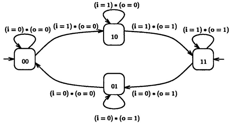
Figure 2.1: A model of a buffer.
