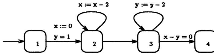
Figure 6.4: An automaton for which the extended TLE algorithm does not terminate.
