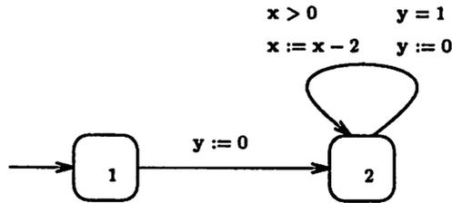
Figure 6.5: An automaton with no infinite sequences admitting consistent timing.
