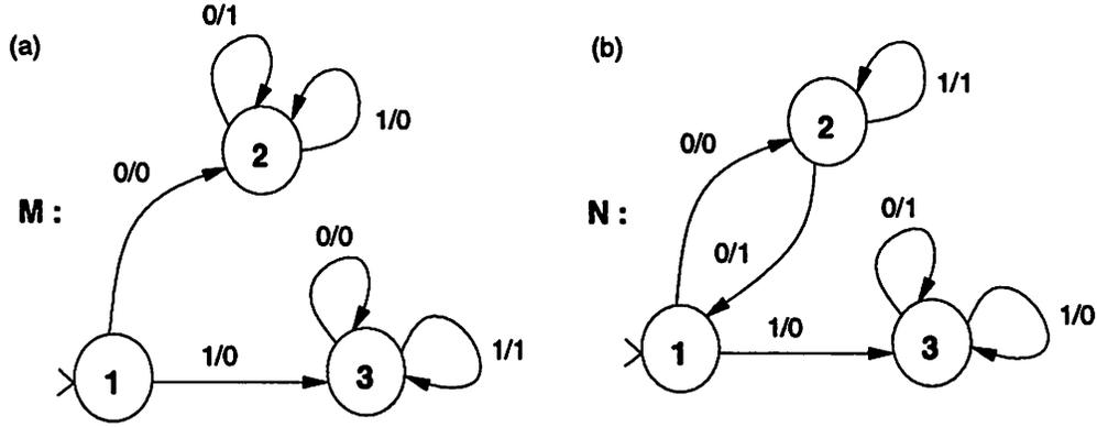
Figure 4: (a) An information lossless and state-minimal machine. (b) A lossy and state-minimal machine.
