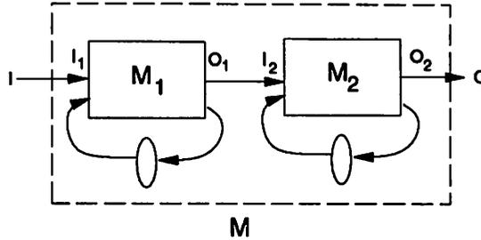
Figure 1: A cascade circuit of two FSM's.
