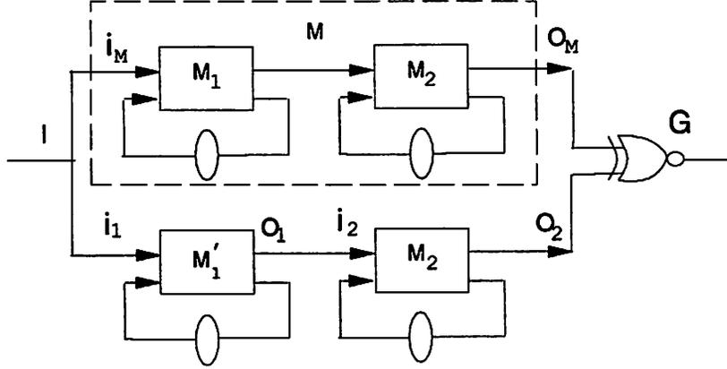
Figure 6: Feasibility testing using FSM equivalence checking.
