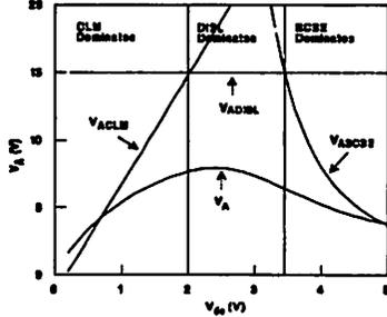
In order to have a smooth transition from triode region to saturation region, the Early voltage ( $V_{Asat}$ ) at  $V_{ds} = V_{dsat}$  is introduced, which can be determined in triode region. If eq. 5 is used in the triode region  $V_{Asat} = E_{sat}L + V_{dsat}$ . The total Early voltage is
