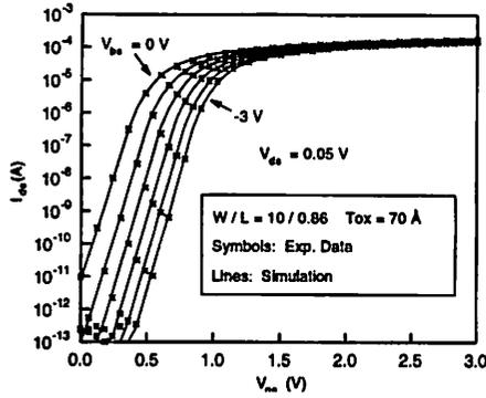
Fig. 9. Drain current vs. gate voltage.  $W/L=10/0.86$
