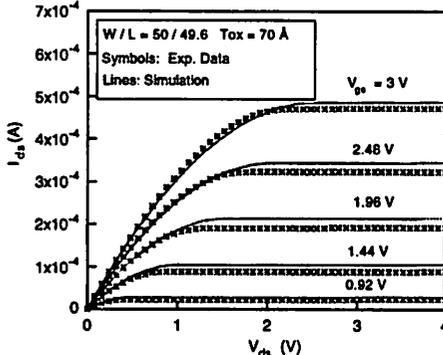
Fig. 12. Drain current vs. drain voltage.  $W/L=50/49.6$ .
