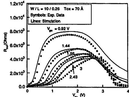
Fig. 8. Output resistance versus drain voltage. W/L=10/0.26
