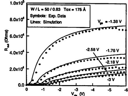
Fig. 14. Output resistance vs. drain voltage. PMOS,  $W/L=50/0.83$
