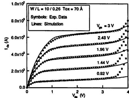
Fig. 7. Drain current versus drain voltage. W/L=10/0.26
