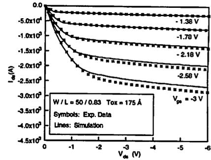
Fig. 13. Drain current vs. drain voltage. PMOS,  $W/L=50/0.83$
