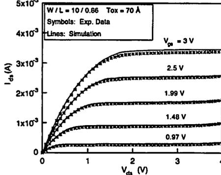
Fig. 10. Drain current vs. drain voltage.  $W/L=10/0.86$
