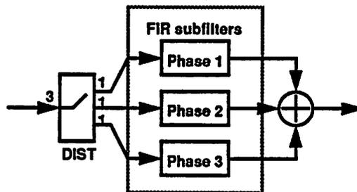
Figure 21. A 1D-SDF specification of a polyphase decimating FIR filter. This description does not expose all the parallelism and has the decimation ratio graphically hard-wired into it.
