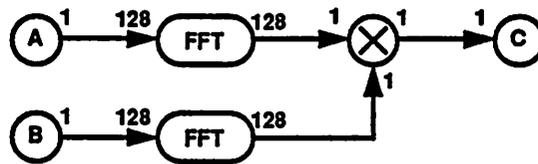
Figure 5. Application of SDF to vector operations.
