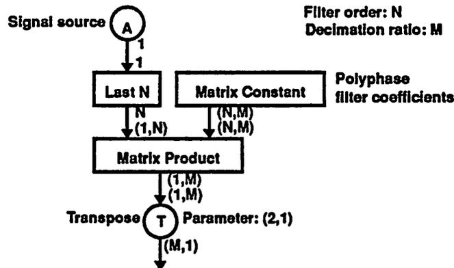
Figure 26. A polyphase interpolating FIR filter expressed using the MD-SDF model. All the parallelism in the algorithm can be automatically exploited.
