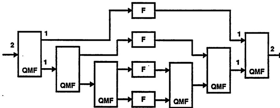
**Figure 8.** An analysis/synthesis filter bank under the SDF model. The depth of the filter bank, however, is hard-wired into the representation.
