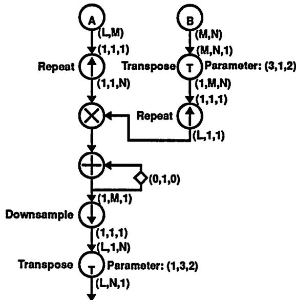
Figure 24. Matrix multiplication in MD-SDF.
