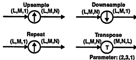
Figure 25. Some key MD-SDF actors that affect the flow of control.
