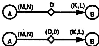
Figure 20. Rule for augmenting the dimensionality of a delay.
