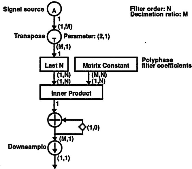
Figure 22. A polyphase decimating FIR filter expressed using MD-SDF. This representation exposes all the parallelism in the algorithm.
