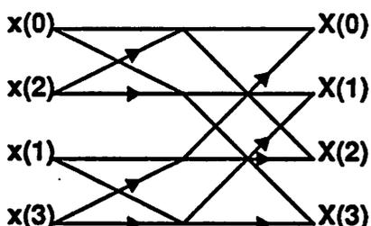
Figure 10. A fourth-order decimation-in-time FFT shown graphically. The order of the FFT, however, is hard-wired into the representation.
