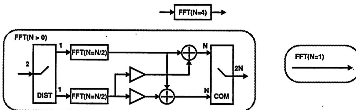
Figure 11. A recursive-iterator representation of the decimation-in-time FFT. This representation is scalable.
