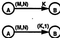
Figure 19. Rule for augmenting the dimensionality of a producer or consumer.
