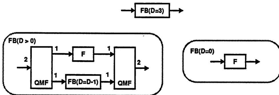
Figure 9. A "recursive iterator" representation of the filter bank application. This representation is scalable.
