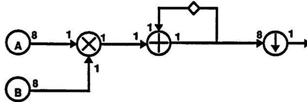
Figure 16. An attempt to use 1D-SDF to repeatedly compute inner products.
