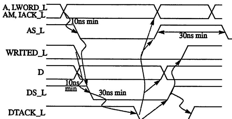
Figure 3-4 : Asynchronous I/O Protocol (VMEbus)
