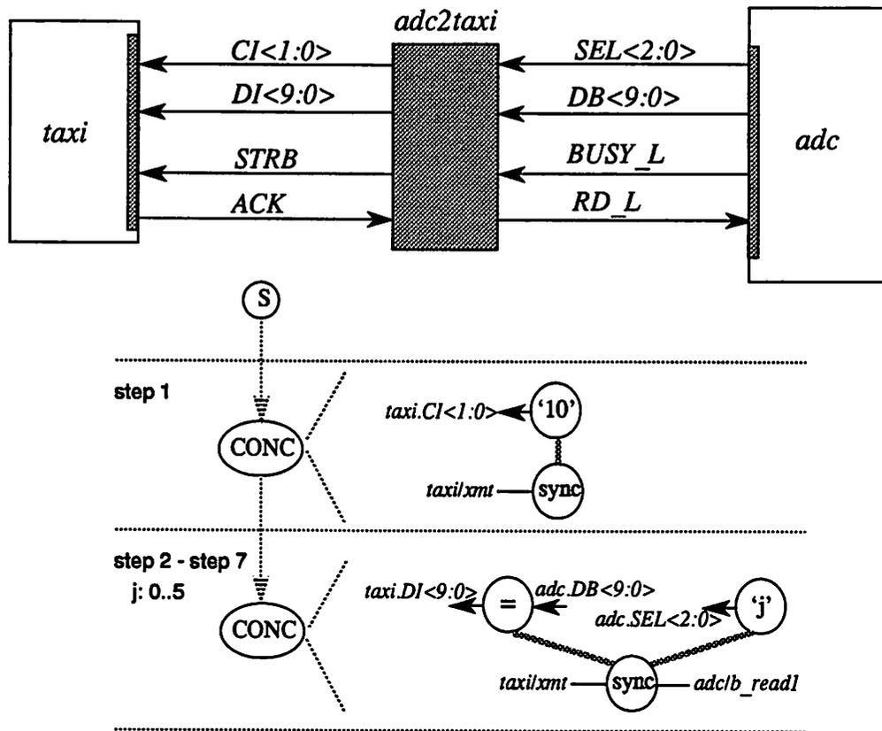
Figure 6-13 : Schedule for A/D Module to Optical Link Interface
