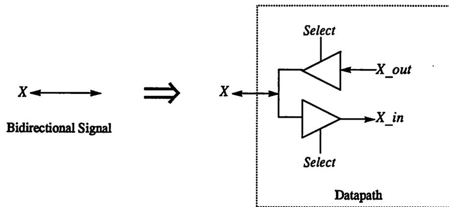
Figure 8-5 : Bidirectional Signal Implementation
