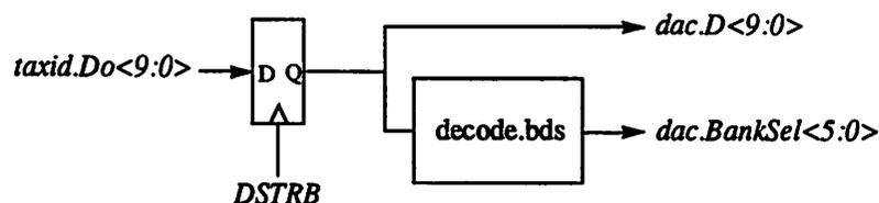
Figure 8-6 : Datapath for the Optical Link to D/A Interface
