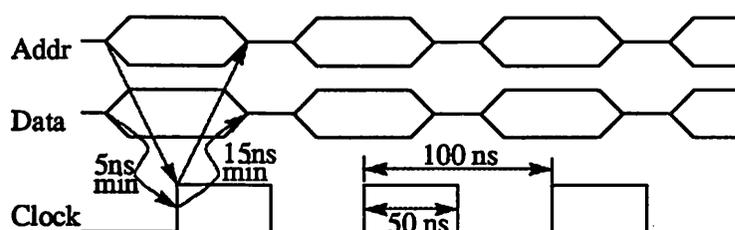
Figure 3-3 : Synchronous I/O Protocol (ASIC)
