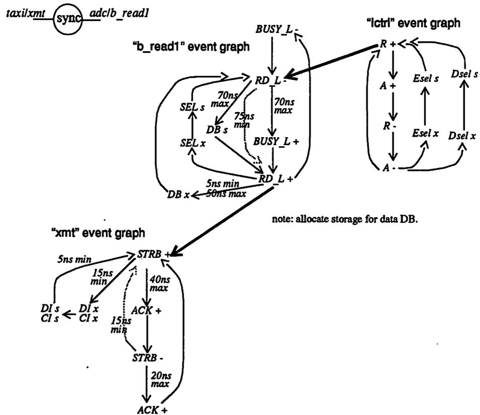
Figure 7-16 : Interlocked Event Graphs for A/D Module to Optical Link Interface
