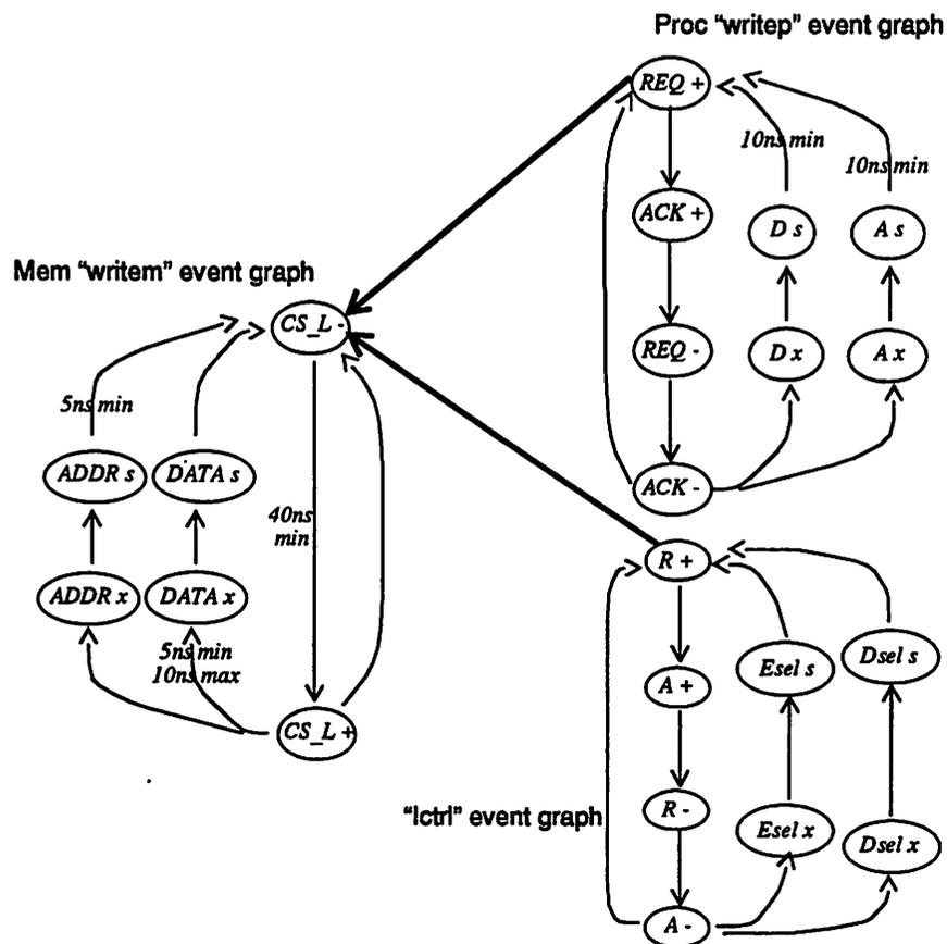
Figure 7-7 : Interlocked Event Graph with Ictrl Handshake
