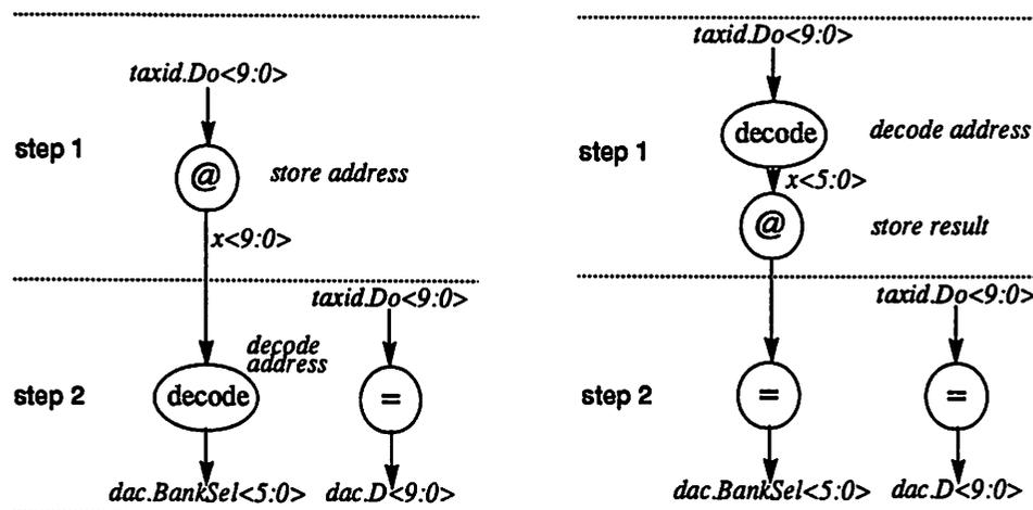
Figure 6-3 : Steps in Flow Graph for Demultiplexed Transfers
