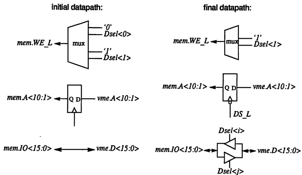
Figure 8-3 : Generating a Register-Transfer Level Datapath
