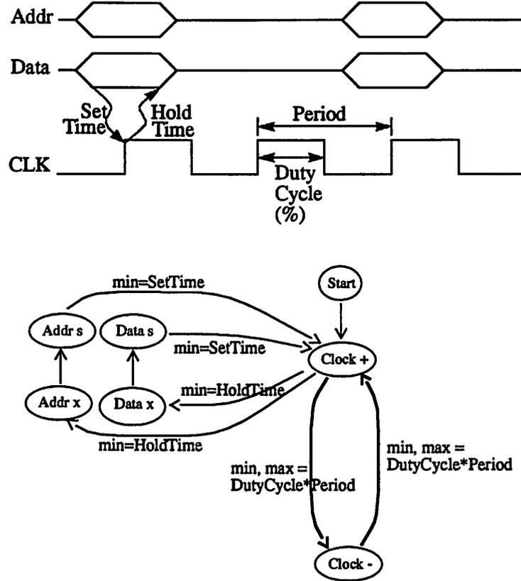
Figure 3-11 : Template for a Synchronous I/O Protocol
