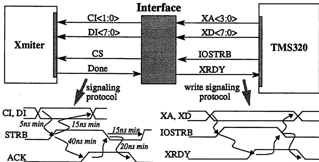
Figure 1-3 : Interface for TMS320 Signal Processor to TAXI Optical Transmitter
