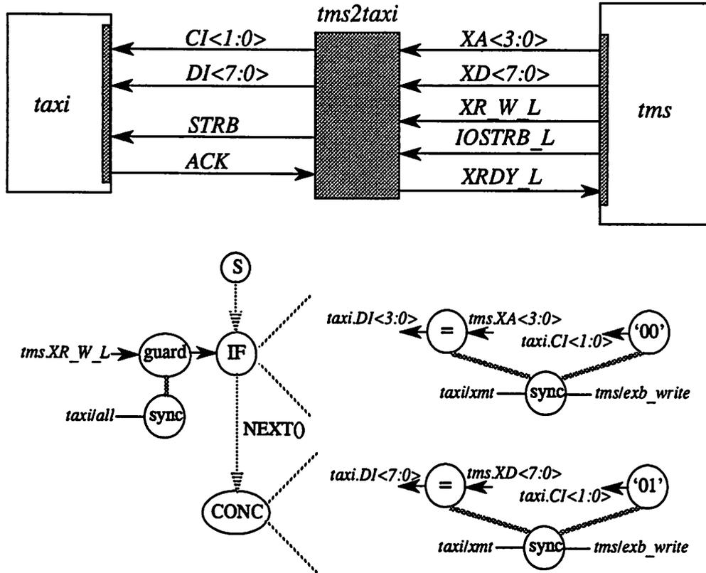
Figure 5-11 : Flow Graph for TMS320 to Optical Link Interface
