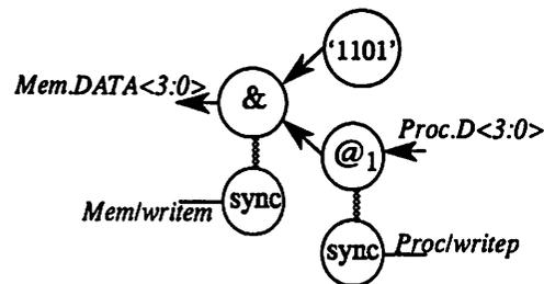
Figure 5-3 : Data Flow Graph with a Complex Operation
