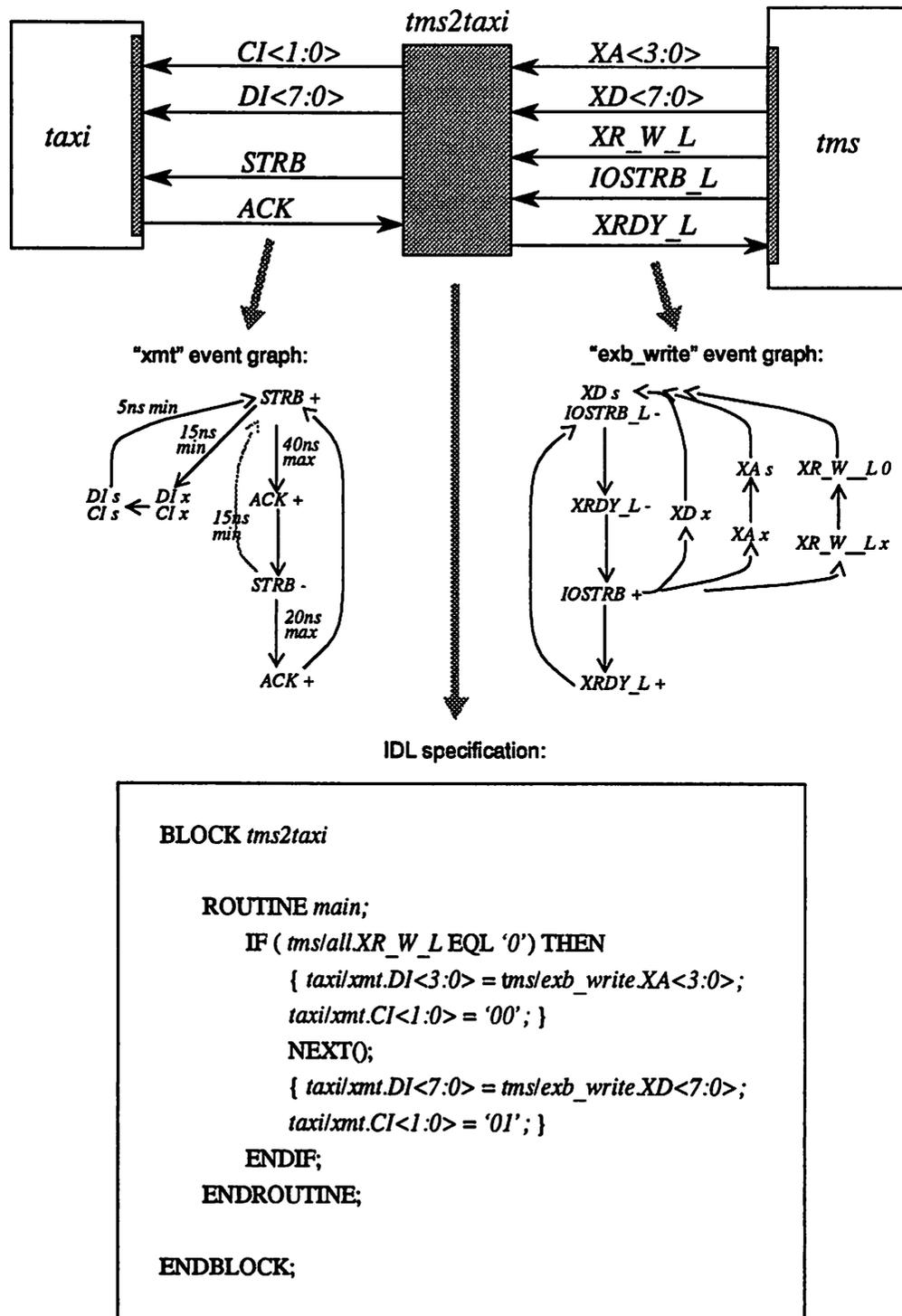
Figure 4-8 : IDL Description for TMS320 to Optical Link Interface
