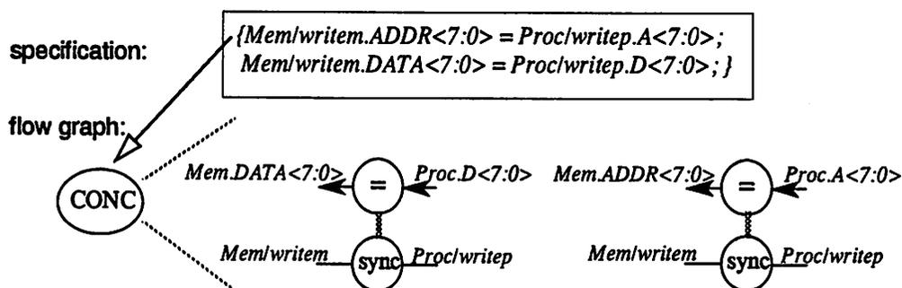
Figure 5-6 : Flow Graph with Concurrent Control Node
