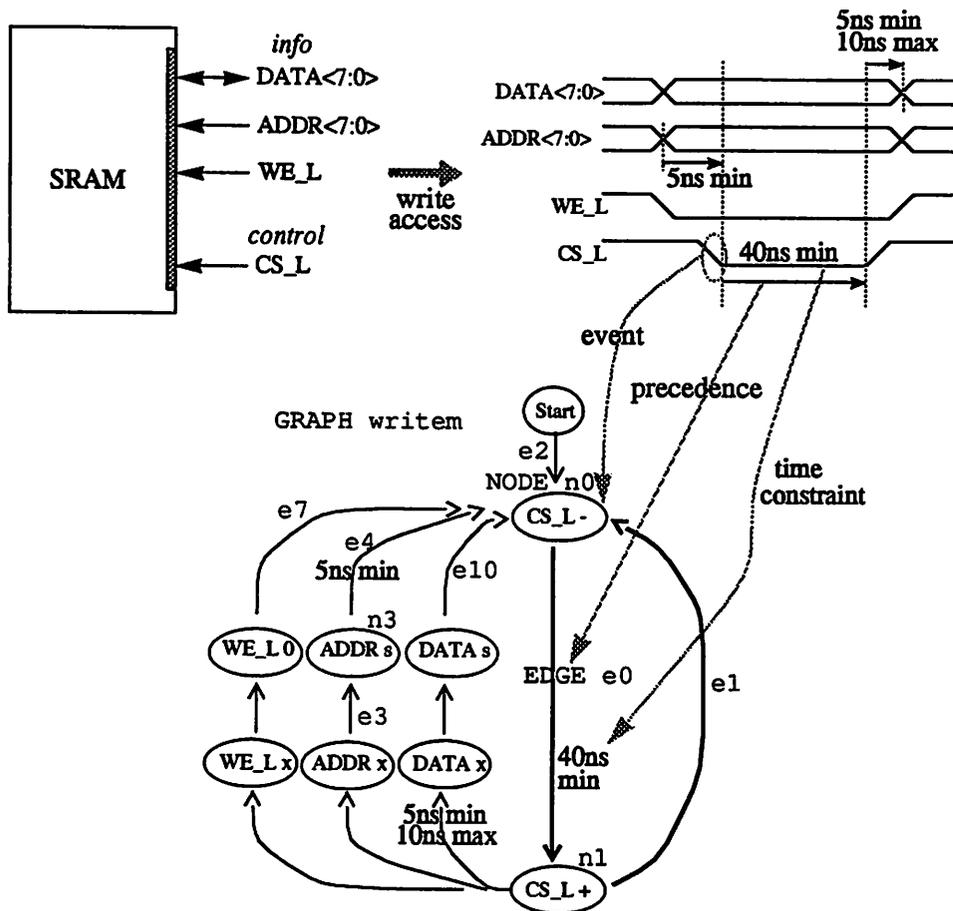
Figure 3-5 : I/O Protocol and Event Graph for SRAM Write Access
