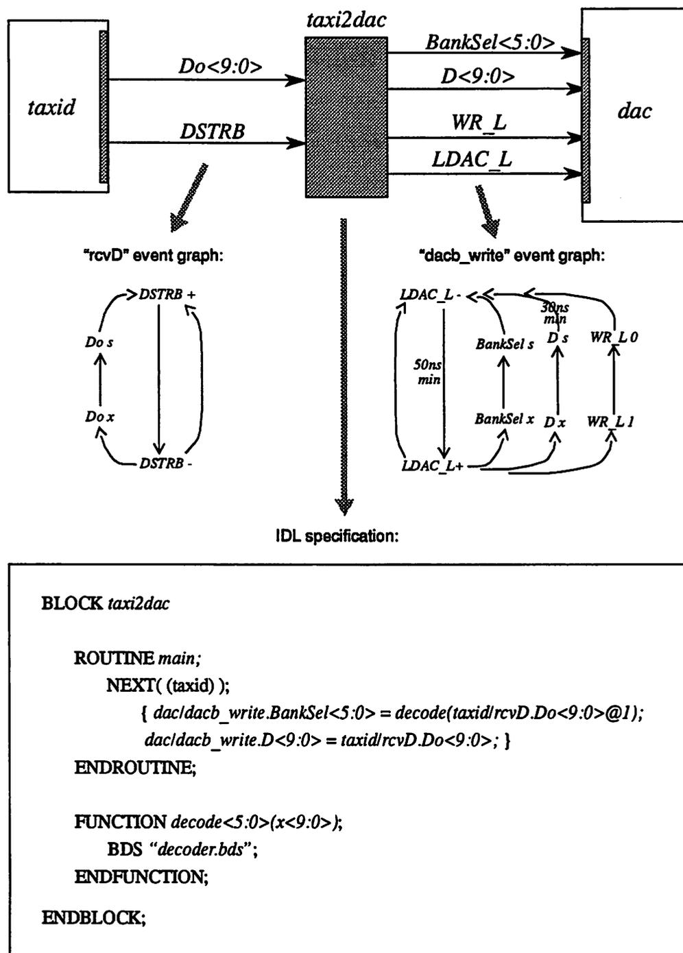
Figure 4-10 : IDL Description for Optical Link to D/A Interface
