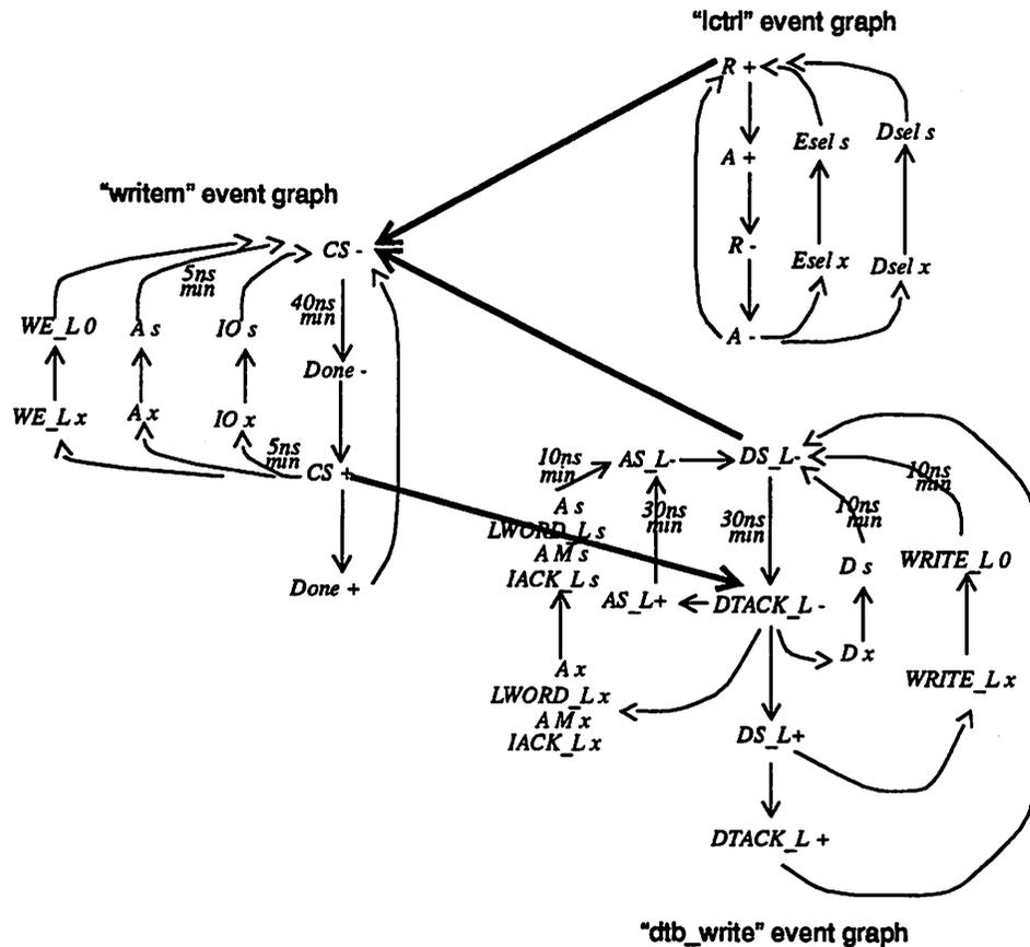
Figure 7-13 : Interlocked Event Graph for VMEbus Write Access
