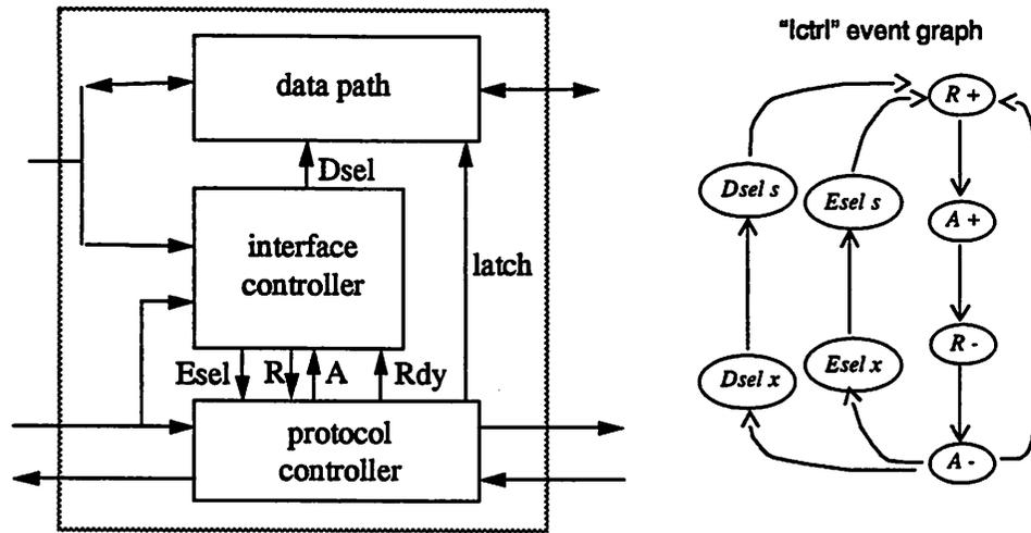
Figure 7-6 : Interface Controller and the Ictrl Handshake
