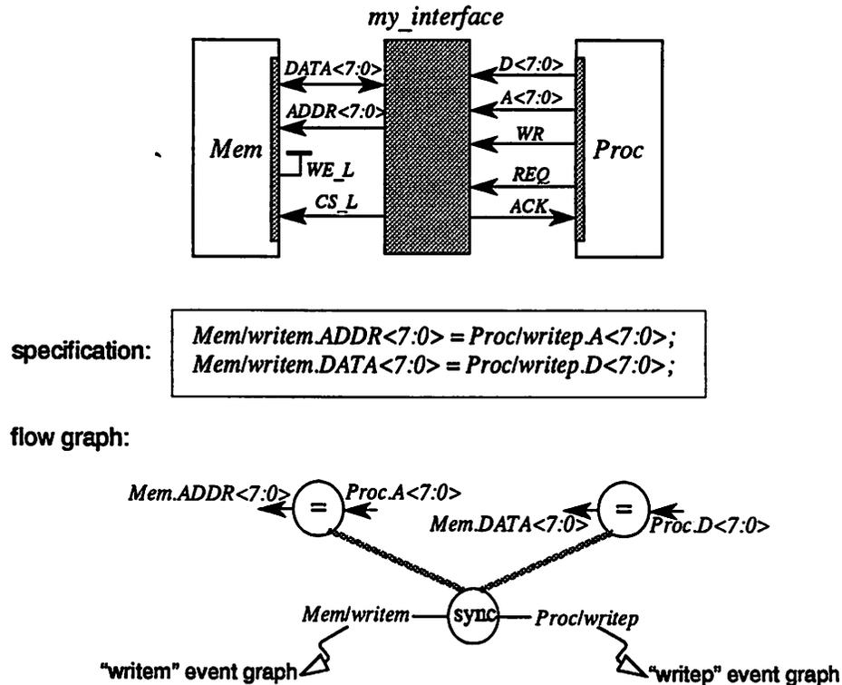
Figure 7-2 : Flow Graph for Processor to Memory Interface
