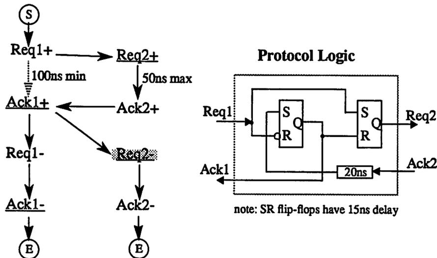
Figure 2-3 : Event Graph for a Handshake Communication
