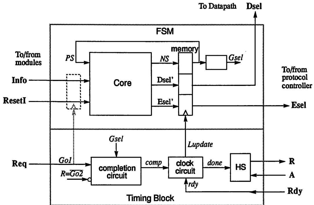
Figure 8-23 : Internal Structure of the Interface Controller
