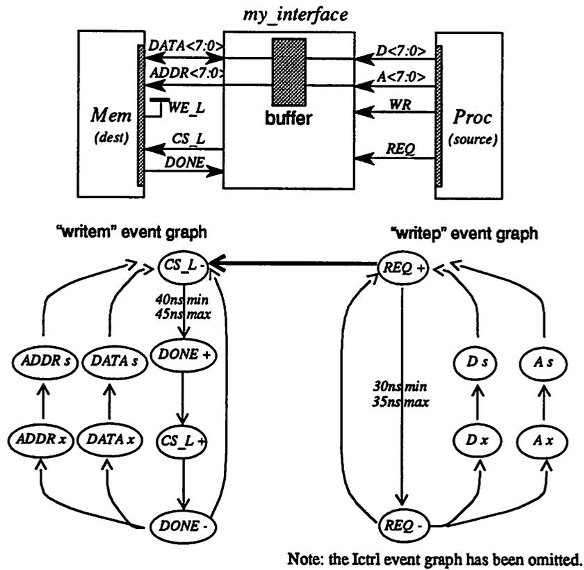
Figure 7-9 : Transfer Synchronization Using a Buffer
