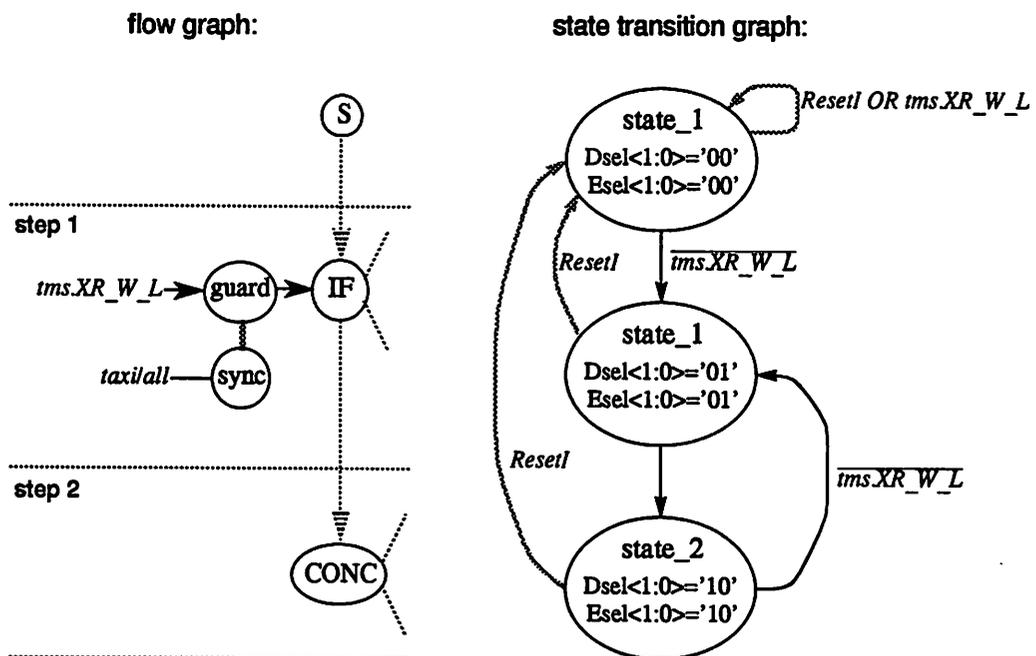
Figure 8-30 : Interface Controller for TMS320 to Optical Link Interface
