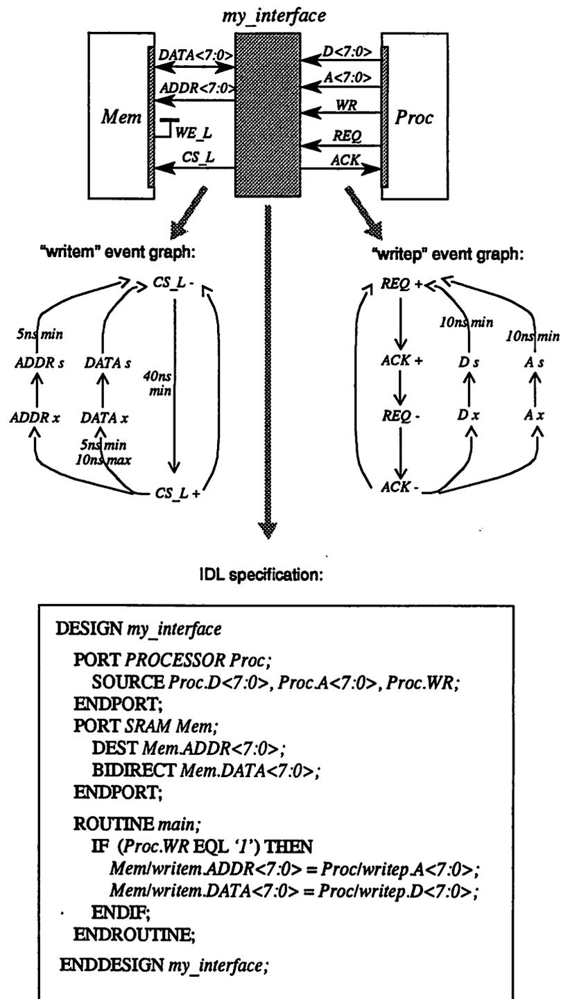
Figure 4-3 : IDL Specification for a Processor to Memory Write Interface
