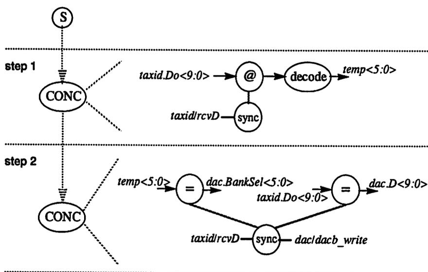
Figure 6-10 : Schedule for the Optical Link to D/A Interface
