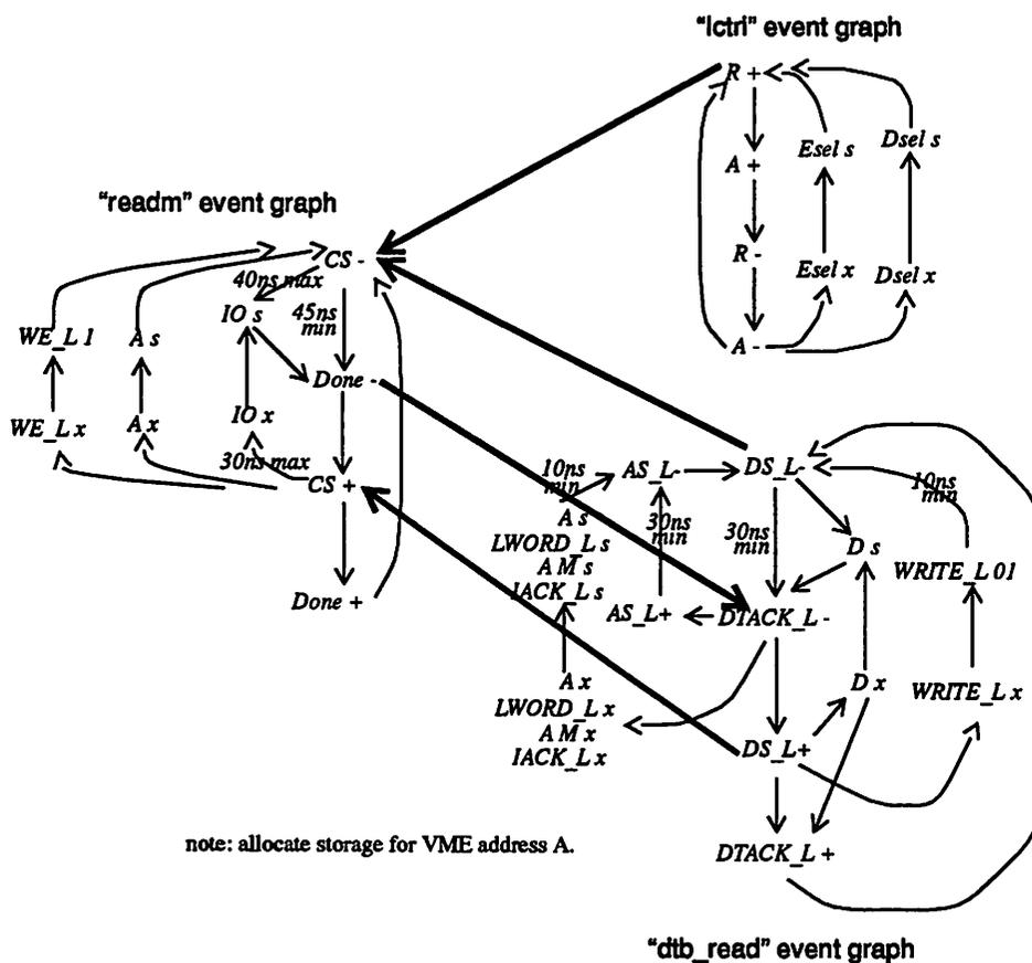
Figure 7-14 : Interlocked Event Graph for VMEbus Read Access
