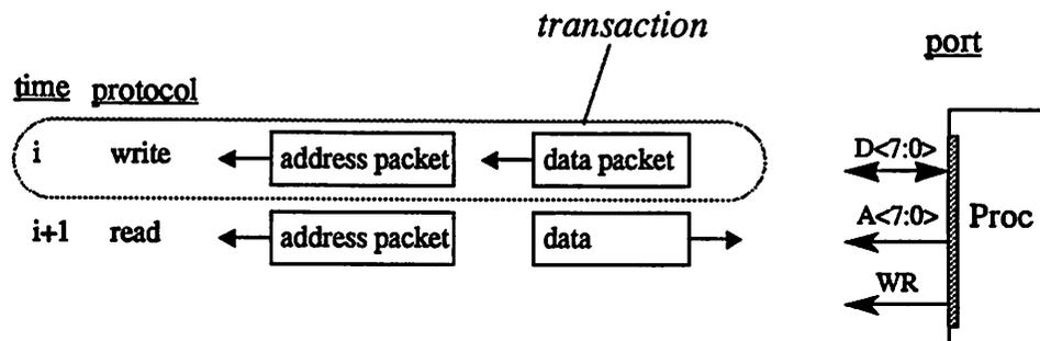
Figure 4-1 : Processor I/O Transactions
