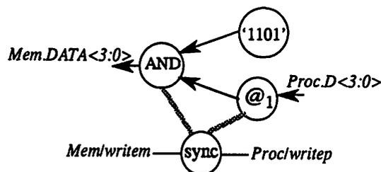
Figure 5-9 : Clustering Data Flow Nodes Into a Complex Operation
