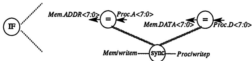
Figure 5-8 : Clustered Flow Graph for Processor to Memory Interface
