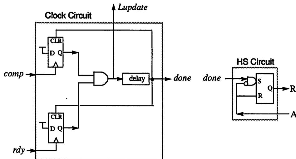
Figure 8-25 : Clock and Handshake Circuit Implementations
