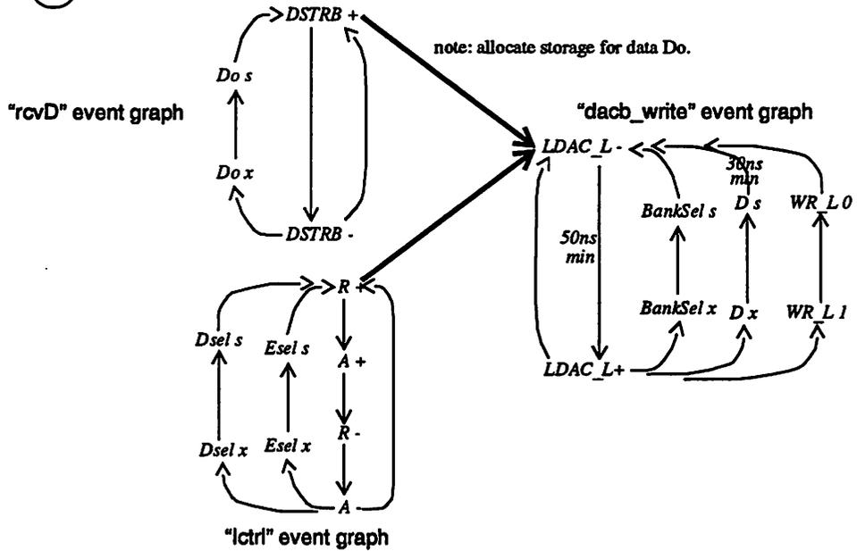
Figure 7-12 : Interlocked Event Graphs for Optical Link to D/A Interface
