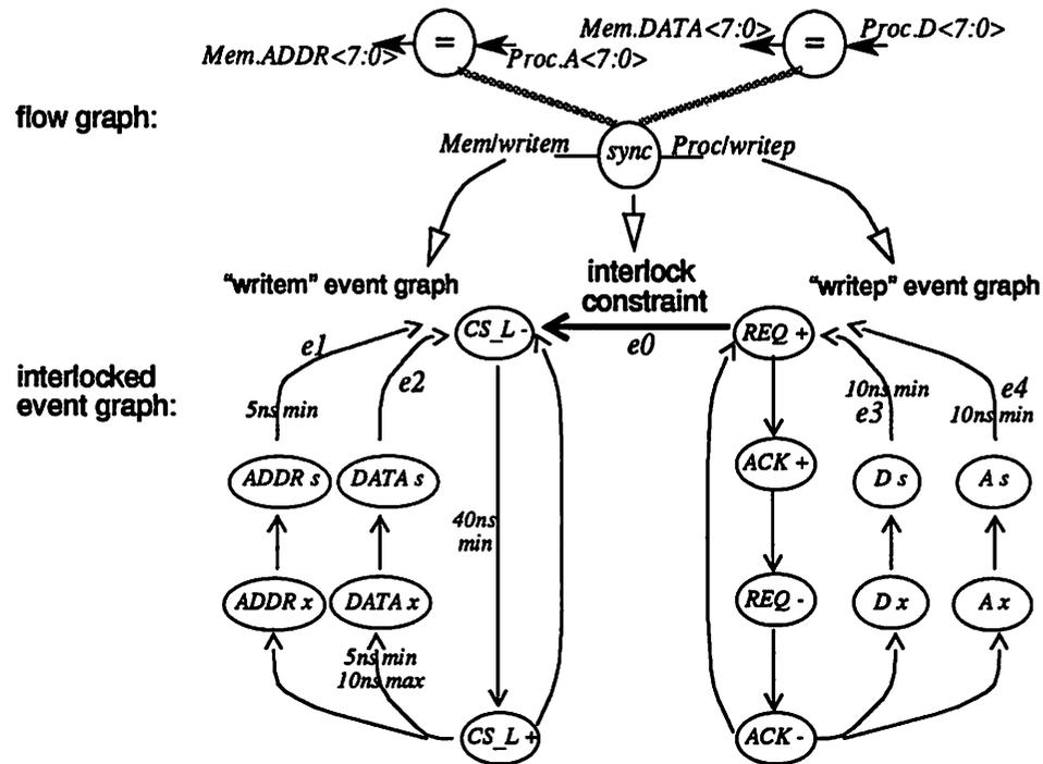
Figure 7-3 : Interlocked Event Graph for Processor to Memory Interface
