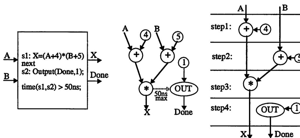
Figure 2-4 : Example of a Flow Graph and Scheduling
