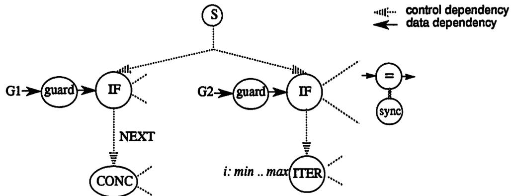
Figure 5-13 : Example of Control and Data Flow Hierarchy
