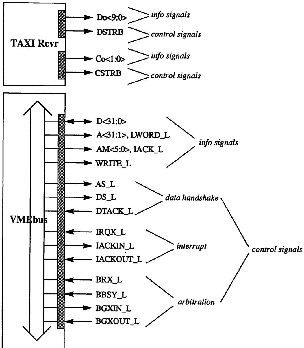
Figure 3-2 : I/O Structure of the TAXI Receiver and the VMEbus
