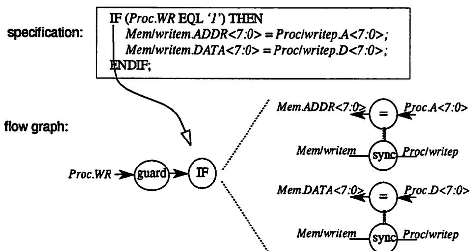
Figure 5-4 : Control/Data Flow Graph for Processor to Memory Interface
