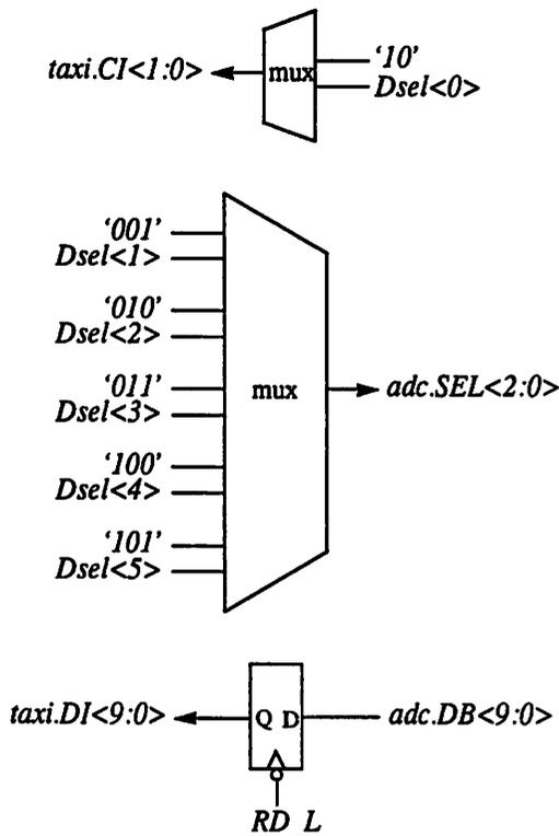
Figure 8-9 : Datapath for A/D Module to Optical Link Interface
