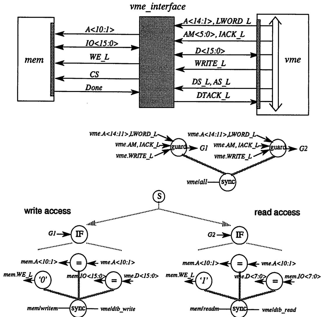
Figure 5-10 : Flow Graph for VMEbus Interface
