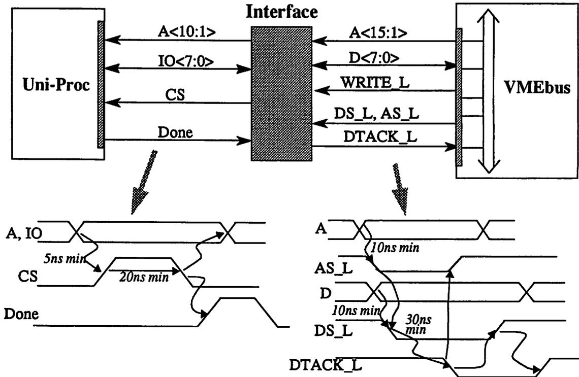
Figure 1-2 : Interface for VMEbus and Uni-processor
