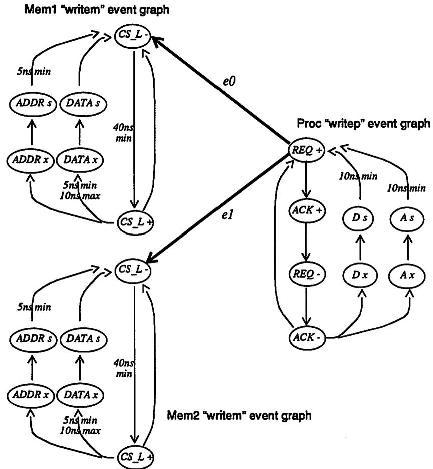
Figure 7-5 : Interlocked Event Graph for a Source and Two Destinations
