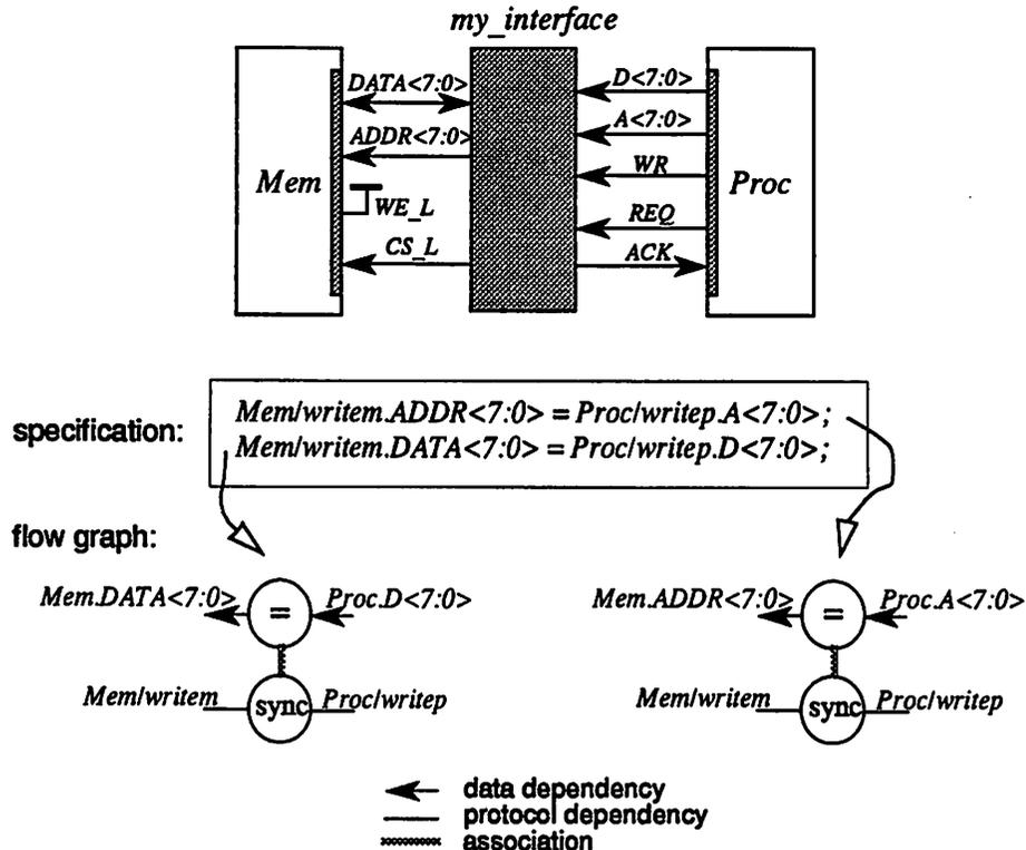
Figure 5-2 : Data Flow Graph for a Processor to Memory Write Interface
