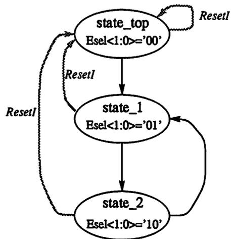
**Figure 8-26 : Interface Controller for the Optical Link to D/A Interface**
