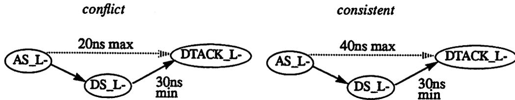
Figure 3-9 : Time Constraint Consistency
