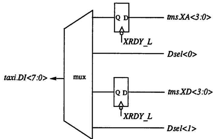
Figure 8-8 : Datapath for TMS320 to Optical Link Interface
