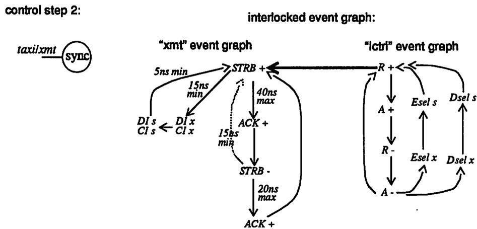
Figure 7-15 : Interlocked Event Graphs for TMS320 to Optical Link Interface
