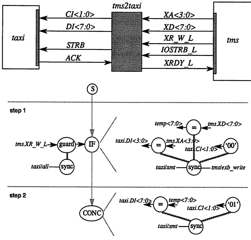
Figure 6-12 : Schedule for TMS320 to Optical Link Interface
