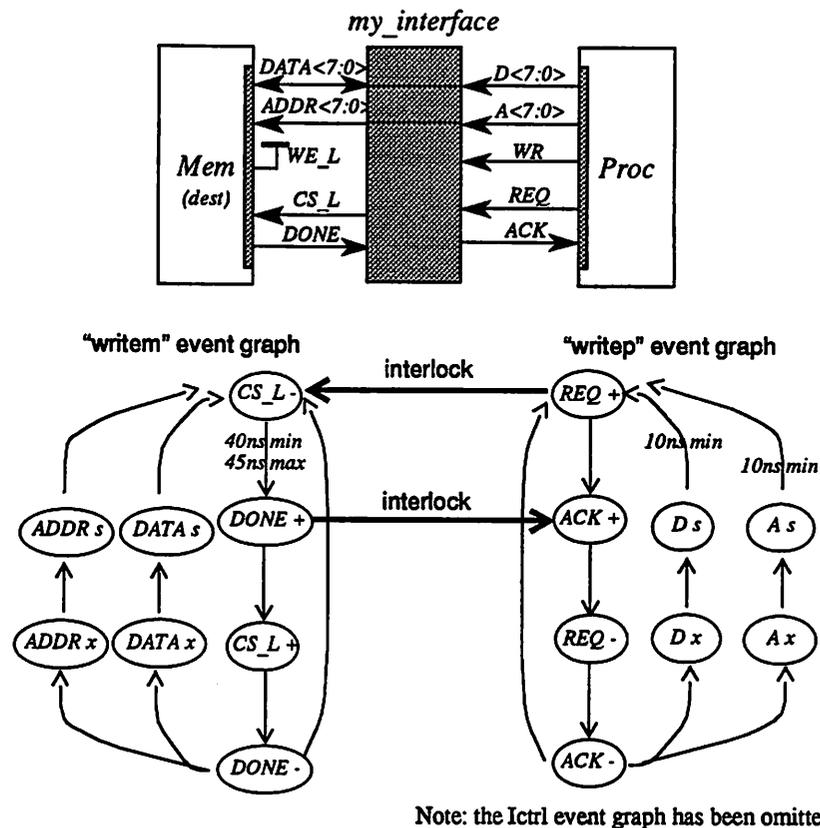
**Figure 7-10 : Interlocked Event Graph for Unbuffered Transfer**
