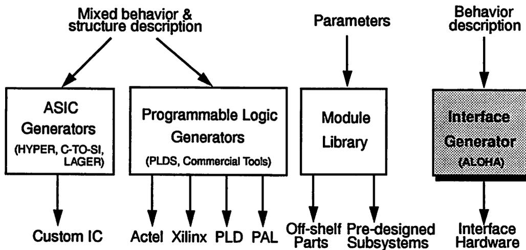
Figure 1-5 : Hardware Module Generation in SIERA
