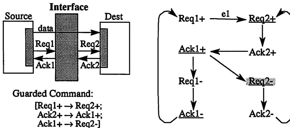
Figure 2-1 : Signal Transition Graph for a Handshake Communication
