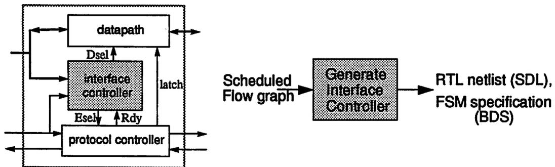
Figure 8-21 : Interface Controller Generation and Output Formats from Synthesis
