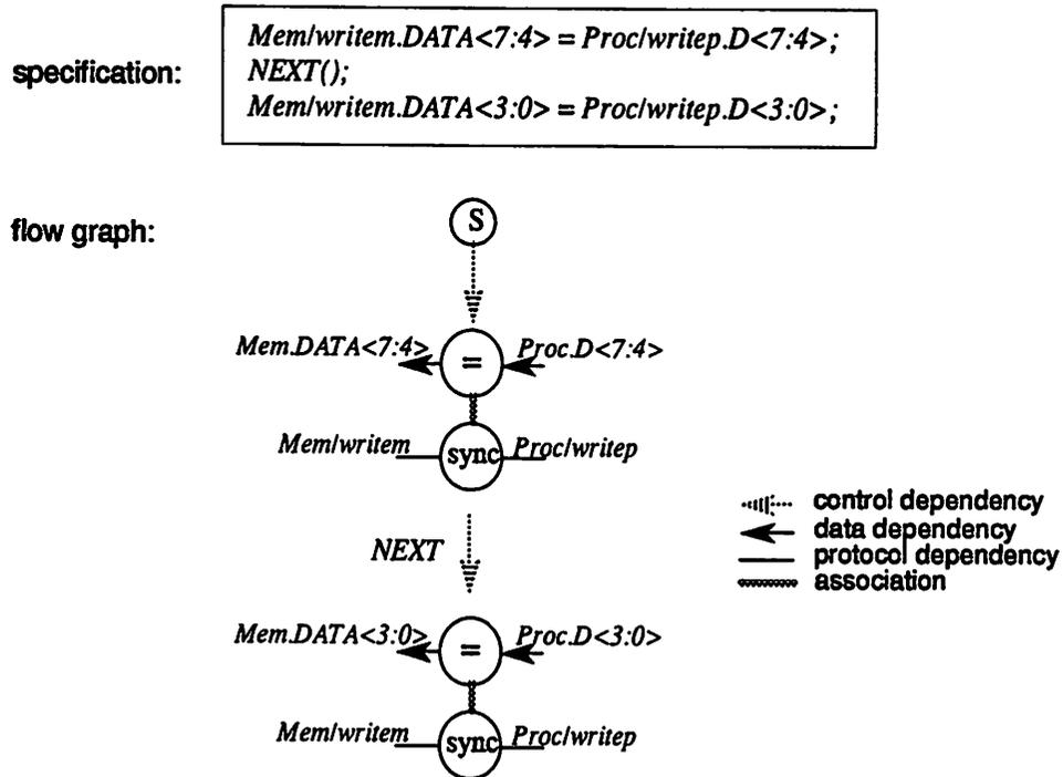
Figure 5-7 : Flow Graph with Control Precedence Edge
