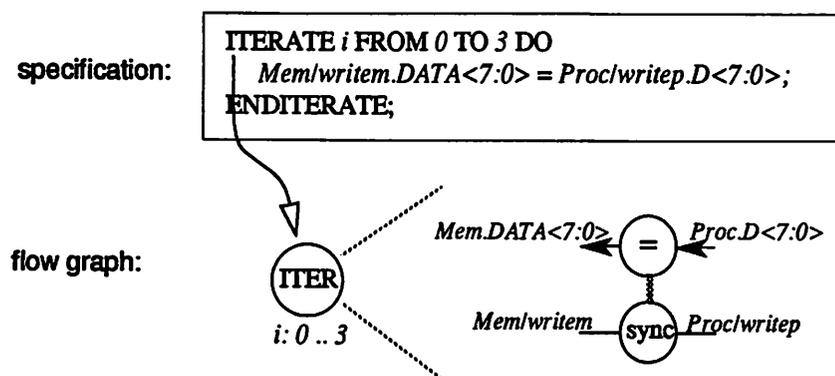
Figure 5-5 : Flow Graph with Iterate Control Node
