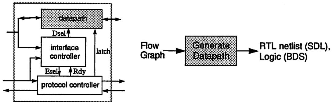
Figure 8-2 : Datapath Generation and Output Formats from Synthesis
