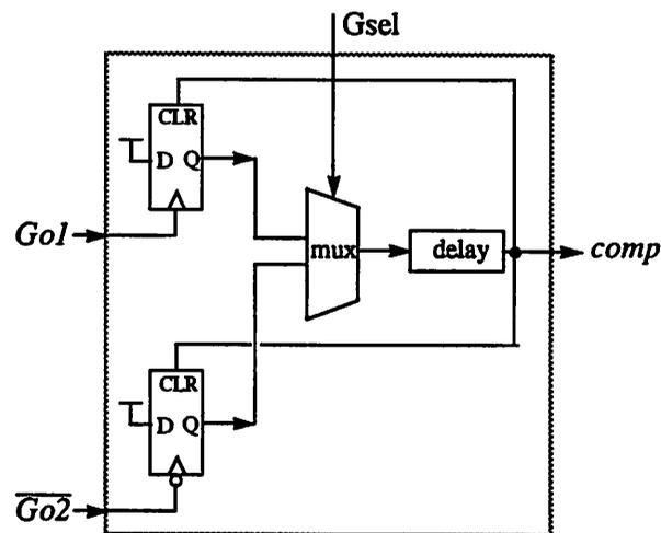
Figure 8-24 : Completion Circuit Implementation
