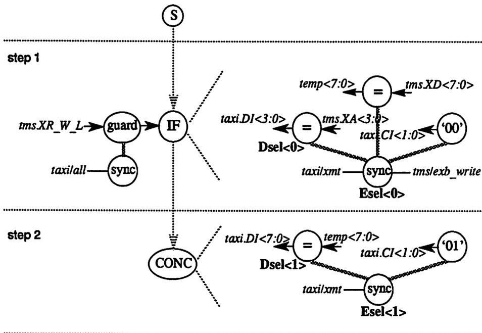
Figure 8-11 : Annotating A Flow Graph with Assigned Dsel and Esel Bits
