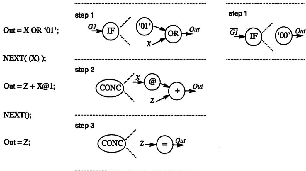
Figure 6-6 : Scheduling of Control and Data Flow Operations
