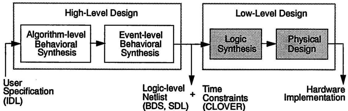
Figure 9-1 : Design Flow for Interface Generation
