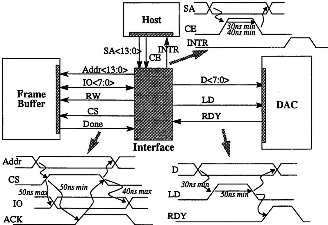
Figure 1-4 : Interface for DMA control of a Video Frame Buffer
