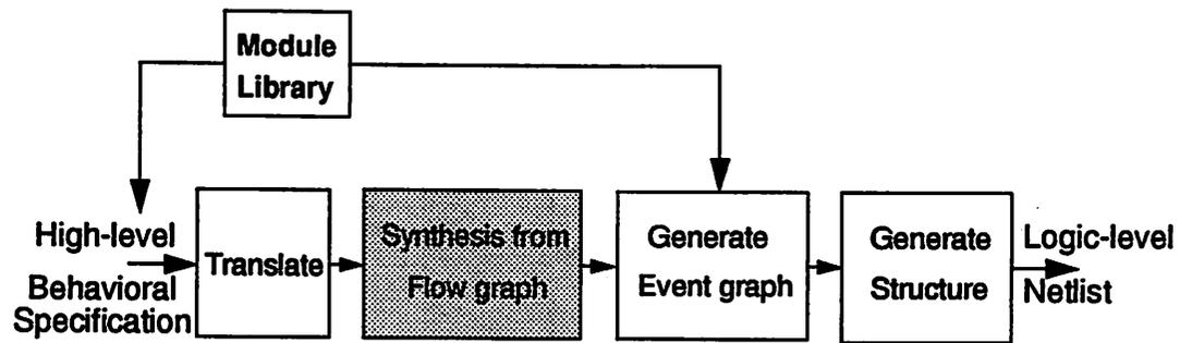
Figure 6-1 : Synthesis from Flow Graph and Interface Generation
