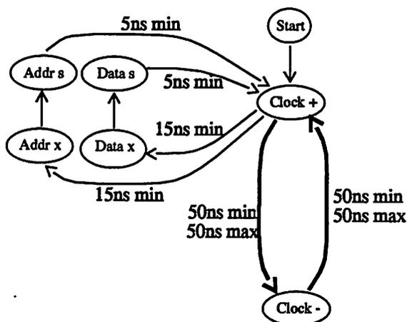
Figure 3-7 : Event Graph for a Synchronous ASIC Protocol
