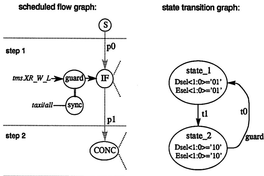
Figure 8-22 : Deriving the State Transition Graph from the Flow Graph
