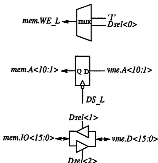
Figure 8-7 : Datapath for VMEbus Interface
