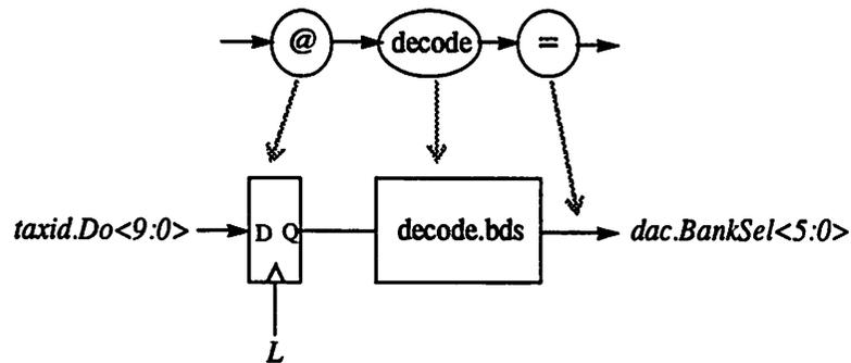
Figure 8-4 : Generating Functional and Storage Units
