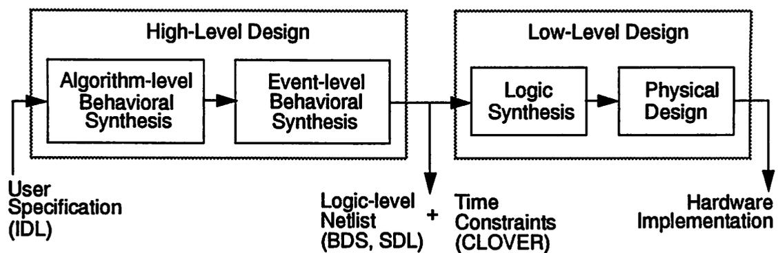
Figure 1-6 : Design Flow for Interface Generation
