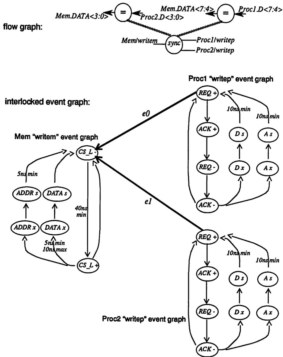
Figure 7-4 : Interlocked Event Graph for Two Sources and a Destination
