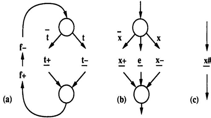
Figure 3: Input choices (a) STG requiring controlled-choice of input signal (b) Common controlled-choice configuration (c) The *hatch* notation for (b)
