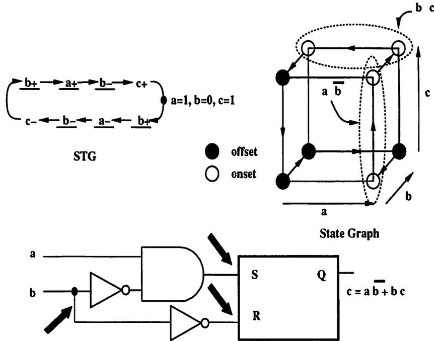
Figure 7: Problem with two-level logic and SR latch implementation
