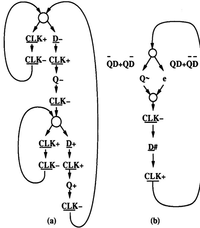
Figure 4: D-latch examples (a) STG using only multiple occurrences of transitions (b) STG using new extensions
