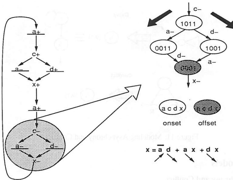
Figure 10: An implementation which is not hazard-free under MIC condition
