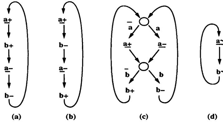
Figure 5: Transition Signaling. (a) Buffer STG. (b) Inverter STG. (c) Using controlled-choice. (d) Using toggles notation.
