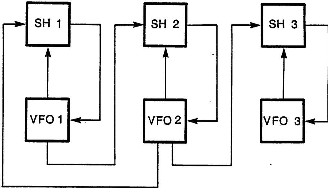
Fig. 7. Communication system consisting of three coupled DPLL's.
