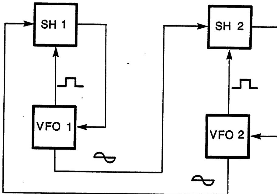
Fig. 2. Two coupled self-synchronizing DPLL's.
