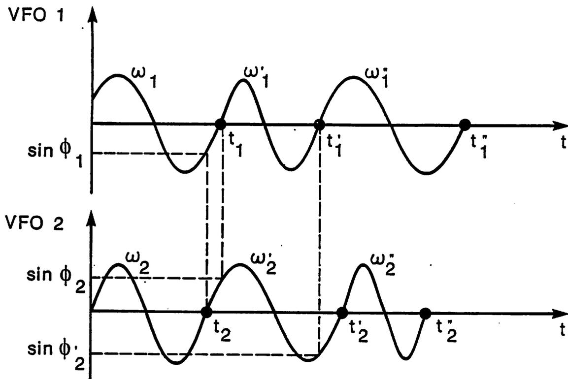
Fig. 3. Schematic representation of the dynamics of the two coupled DPLL's.
