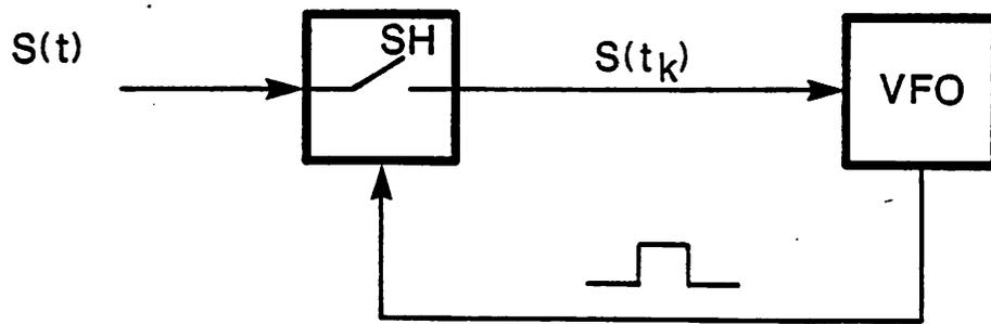
Fig. 1. Schematic representation of a single DPLL.
