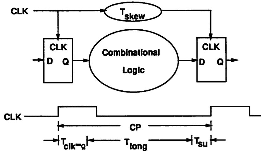
Figure 2.4: Figure illustrating clocking constraints
