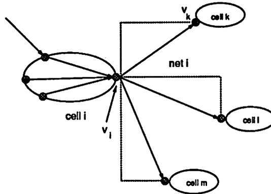
Figure 5.1: Example of a star connected net
