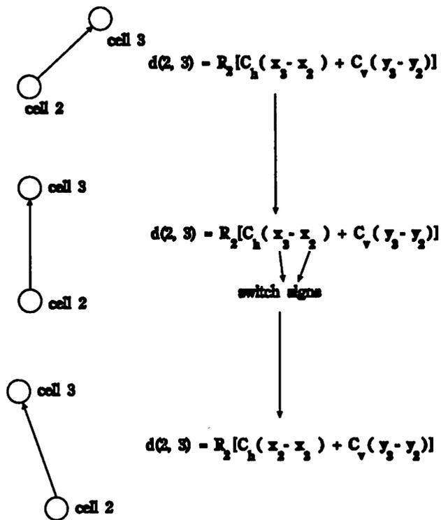
Figure 5.3: Linearizing absolute valued constraints
