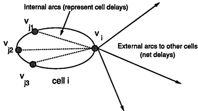
Figure 2.6: Internal and external arcs of a cell
