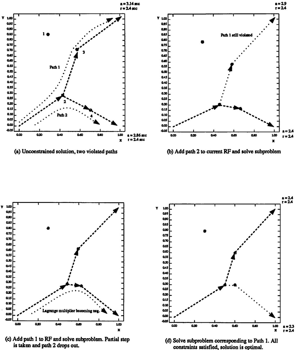
Figure 4.1: Steps of Dual algorithm on example
