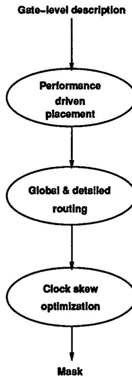
Figure 7.1: Figure showing the role of clock skew optimization
