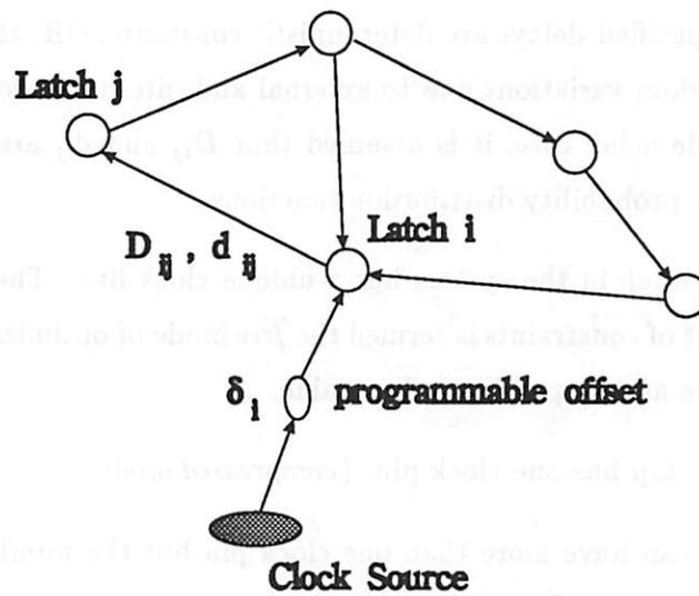
Figure 7.3: A synchronous communication graph
