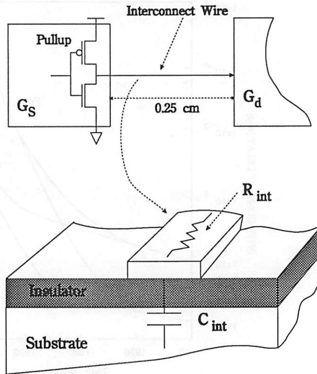
Figure 1.4: Example to quantify the contribution of wire delay
