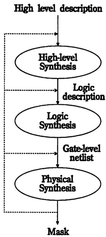
Figure 1.1: The flow of a typical IC design
