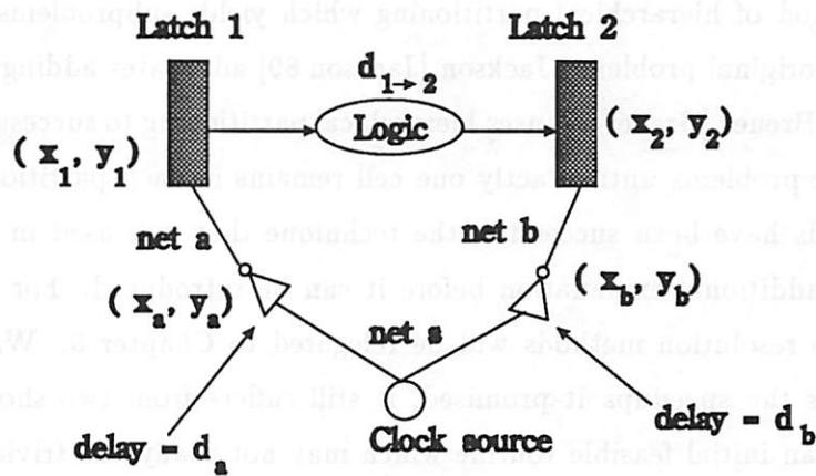
Figure 3.7: Clock tree placement example
