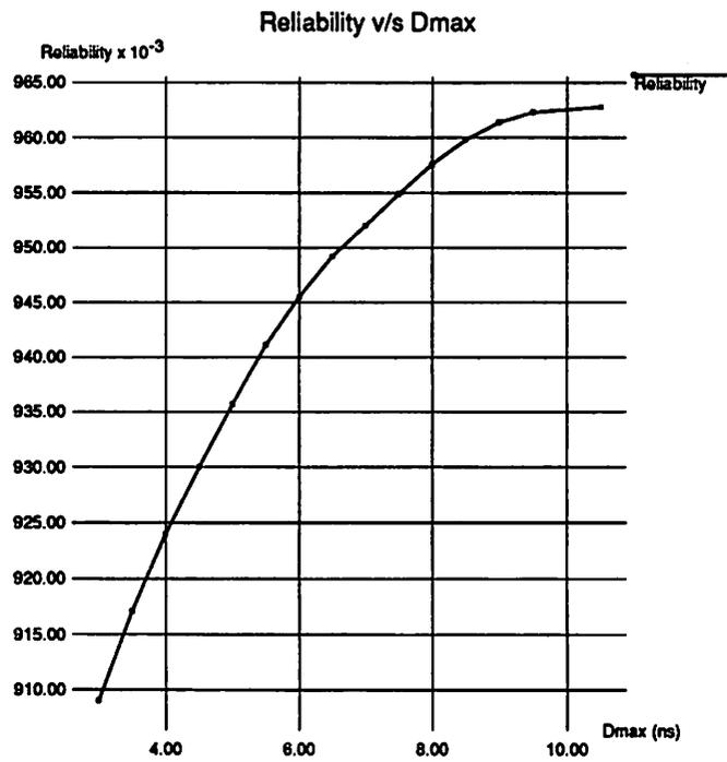
Figure 7.8: Reliability v/s  $\Delta_{max}$ , normal distribution,  $T_0 = 30ns$
