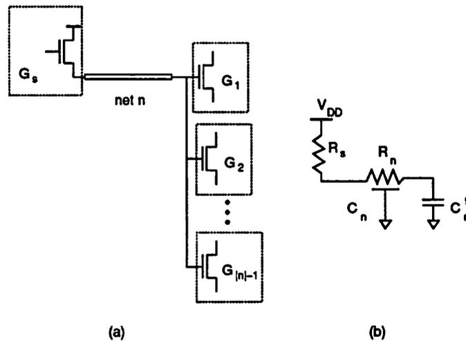
Figure 2.7: A net (a), and associated interconnect delay model (b)
