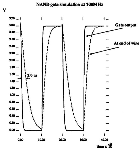
Figure 1.5: Simulated waveforms to illustrate wire delay
