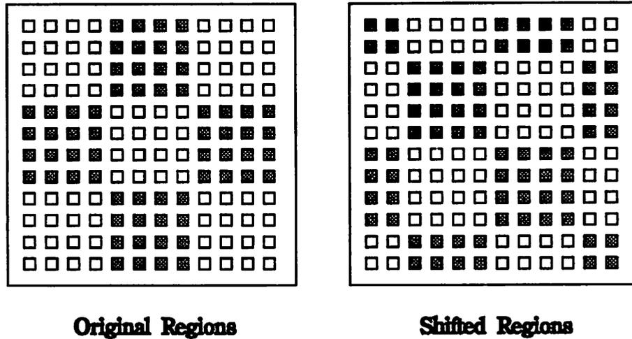
Figure 5.6: Regions of optimization are shifted at alternate iterations
