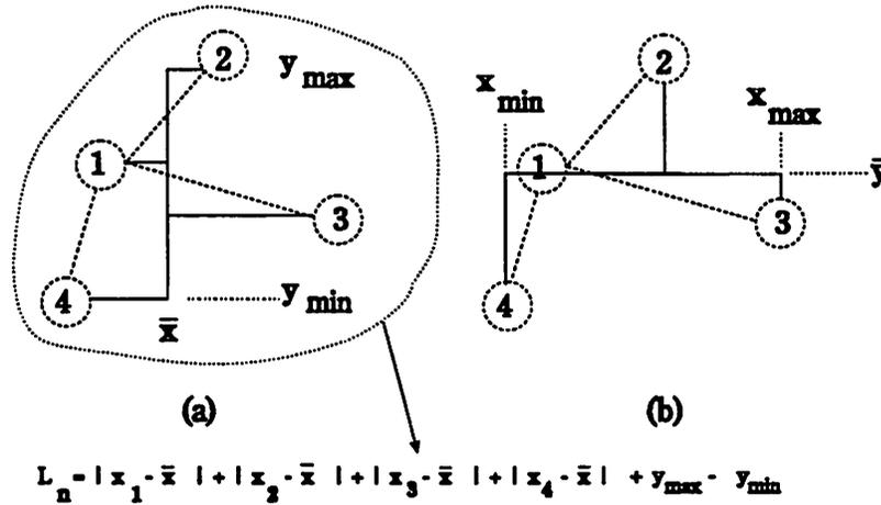
Figure 2.3: Single-trunk Steiner tree wirelength model
