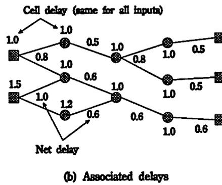
Figure 3.1: An example of a netlist, its vertex numbering and delays
