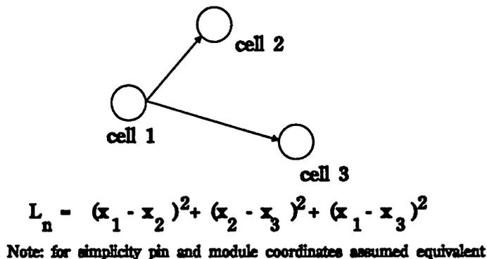
Figure 2.1: The Quadratic wirelength model
