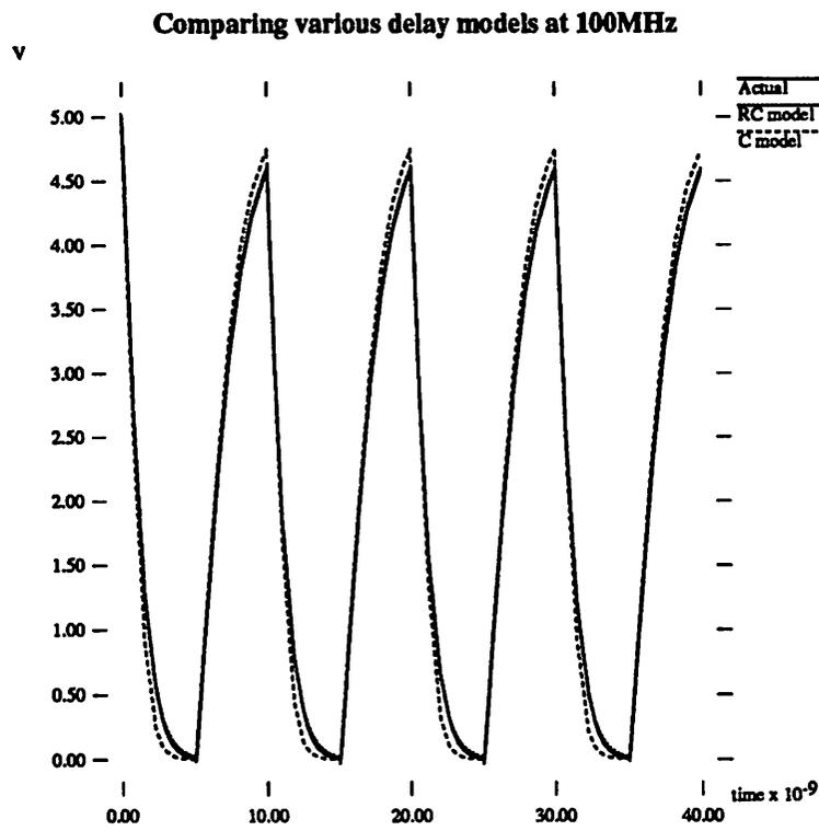
Figure 2.8: Simulation to compare various delay models
