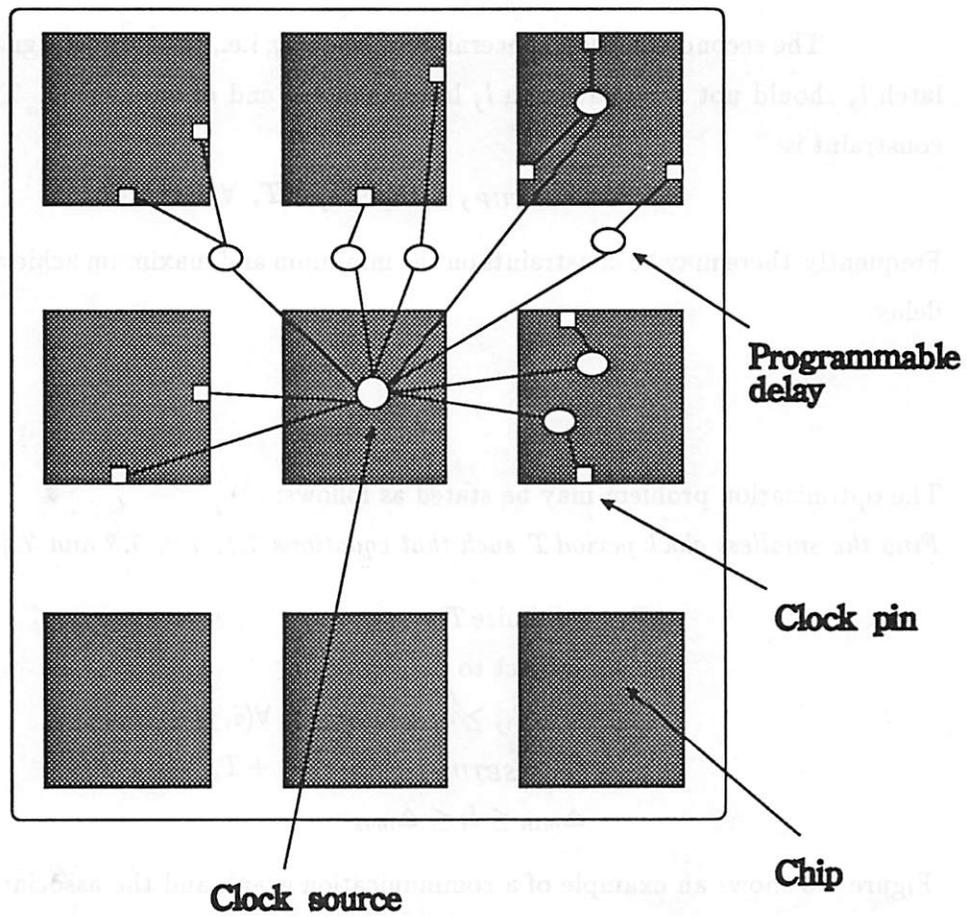
Figure 7.2: An example of a clock distribution network on a MCM
