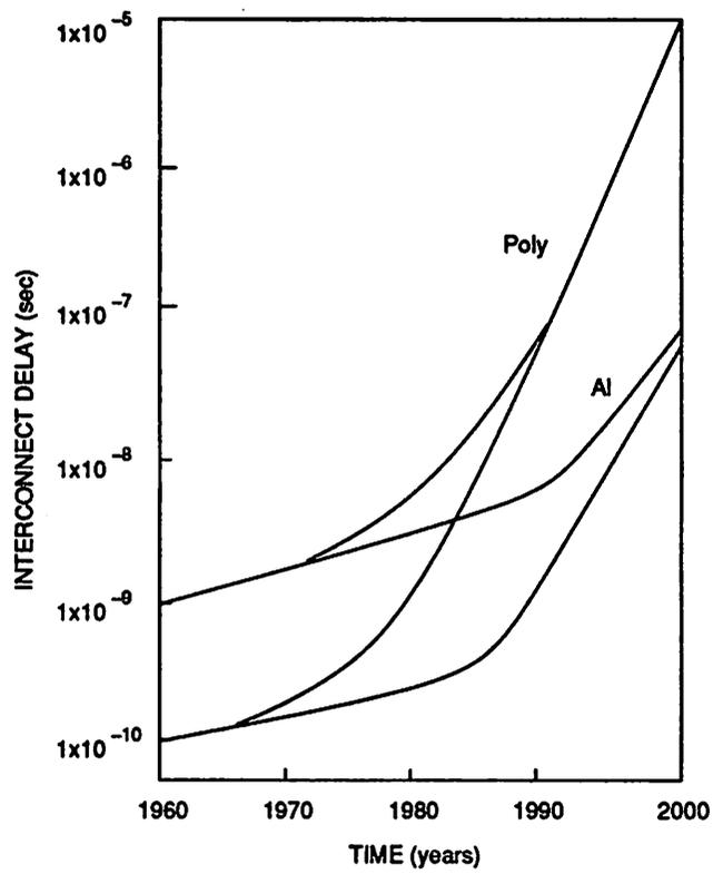
Figure 1.3: Graph illustrating the increase of global interconnect delays with time
