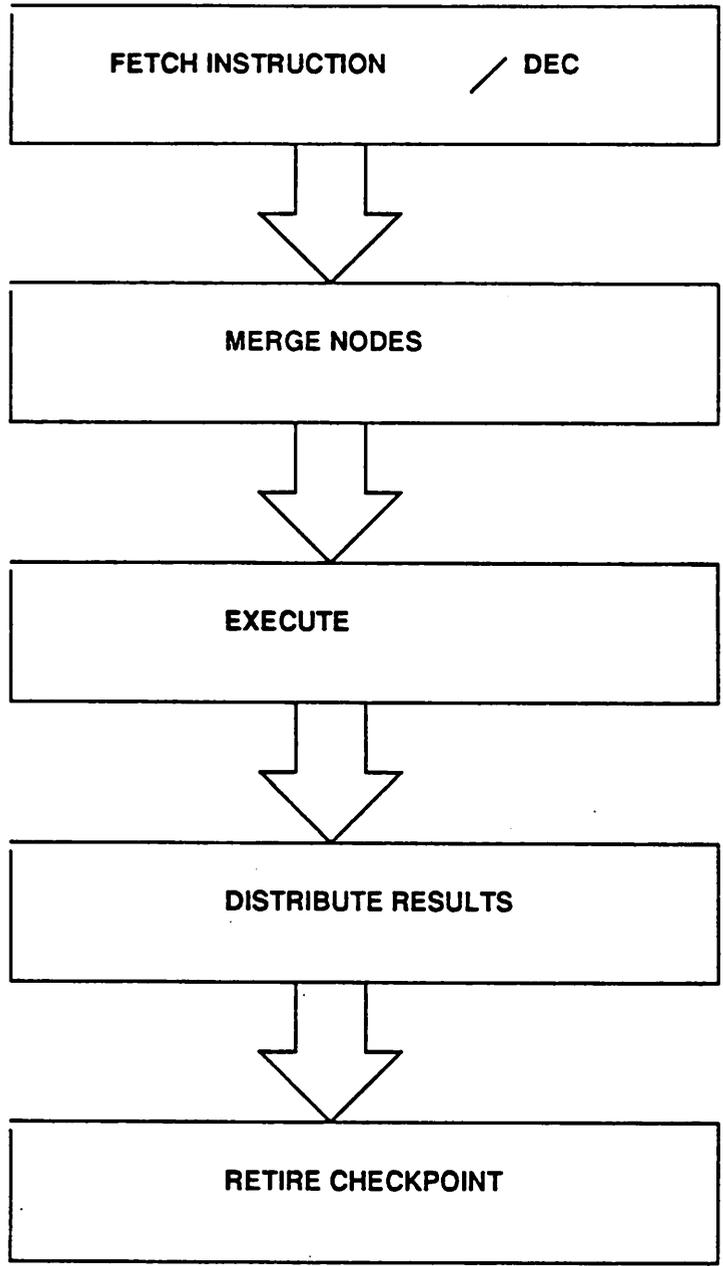
**Fig. 3: HPSm Simplified Pipeline**
