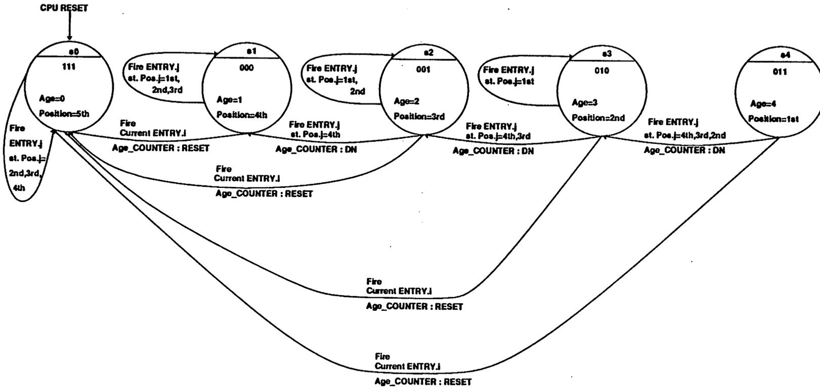
Fig. 9b. ENTRY.I AGE State Transition Diagram for FIRing
