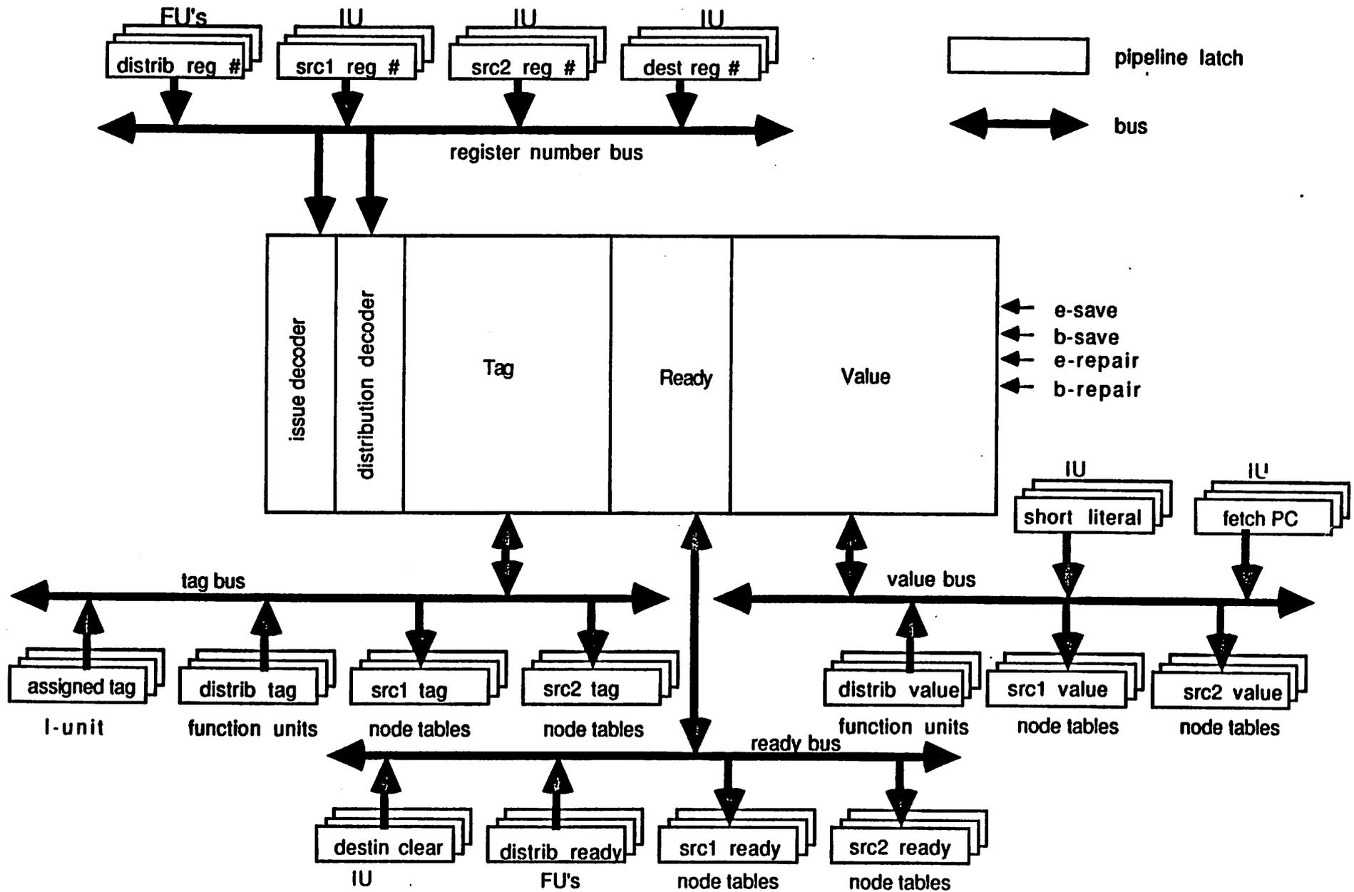
**Fig. 2 : RAT with Global Busses and Signals**
