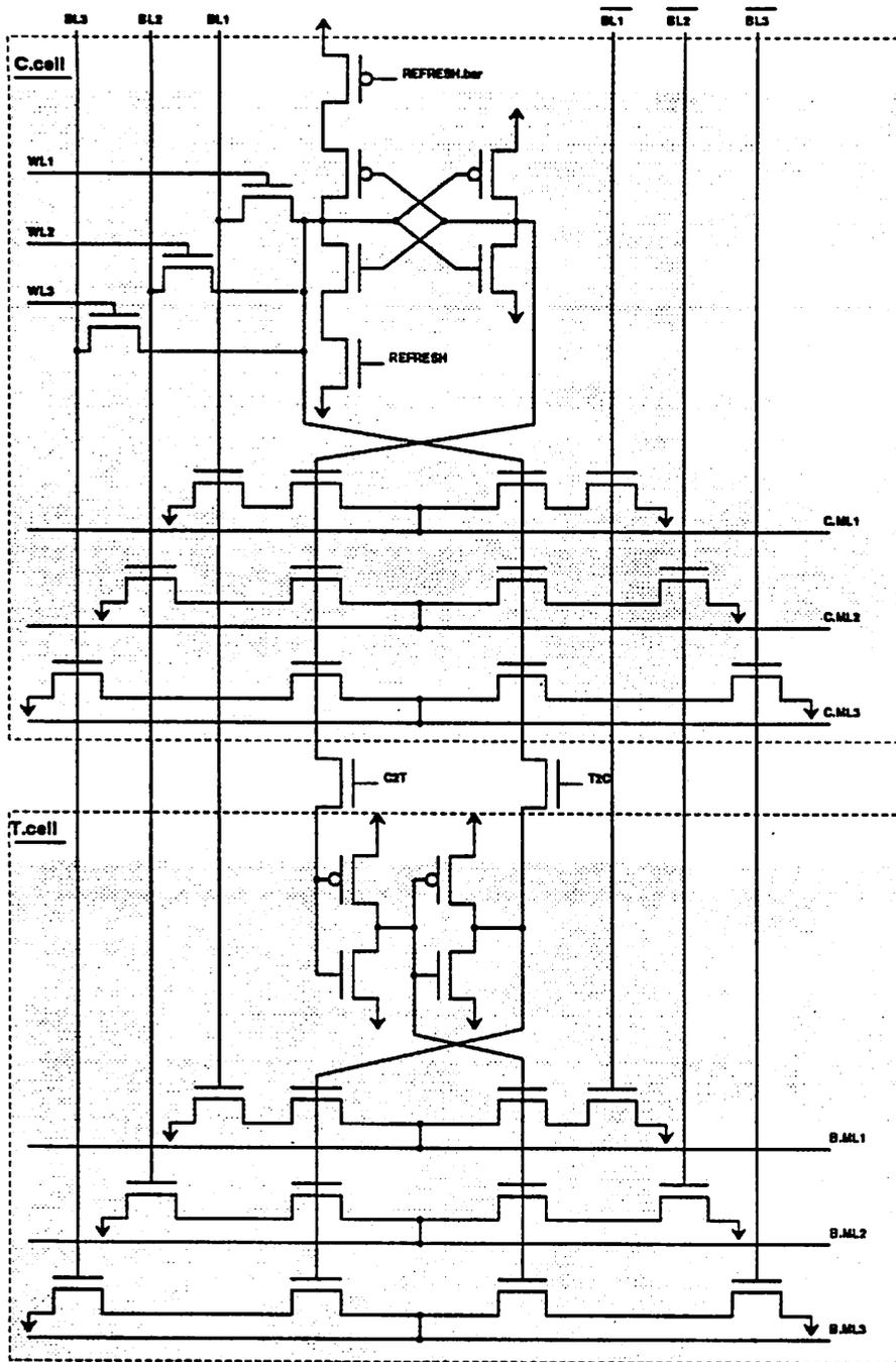
**Fig. 7: Tag "Double-CAM" Cell Schematic**
