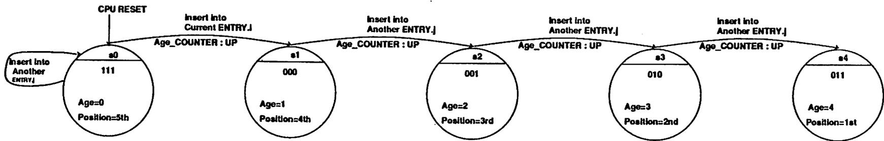
Fig. 8b. ENTRY.i AGE State Transition Diagram for INSERTion
