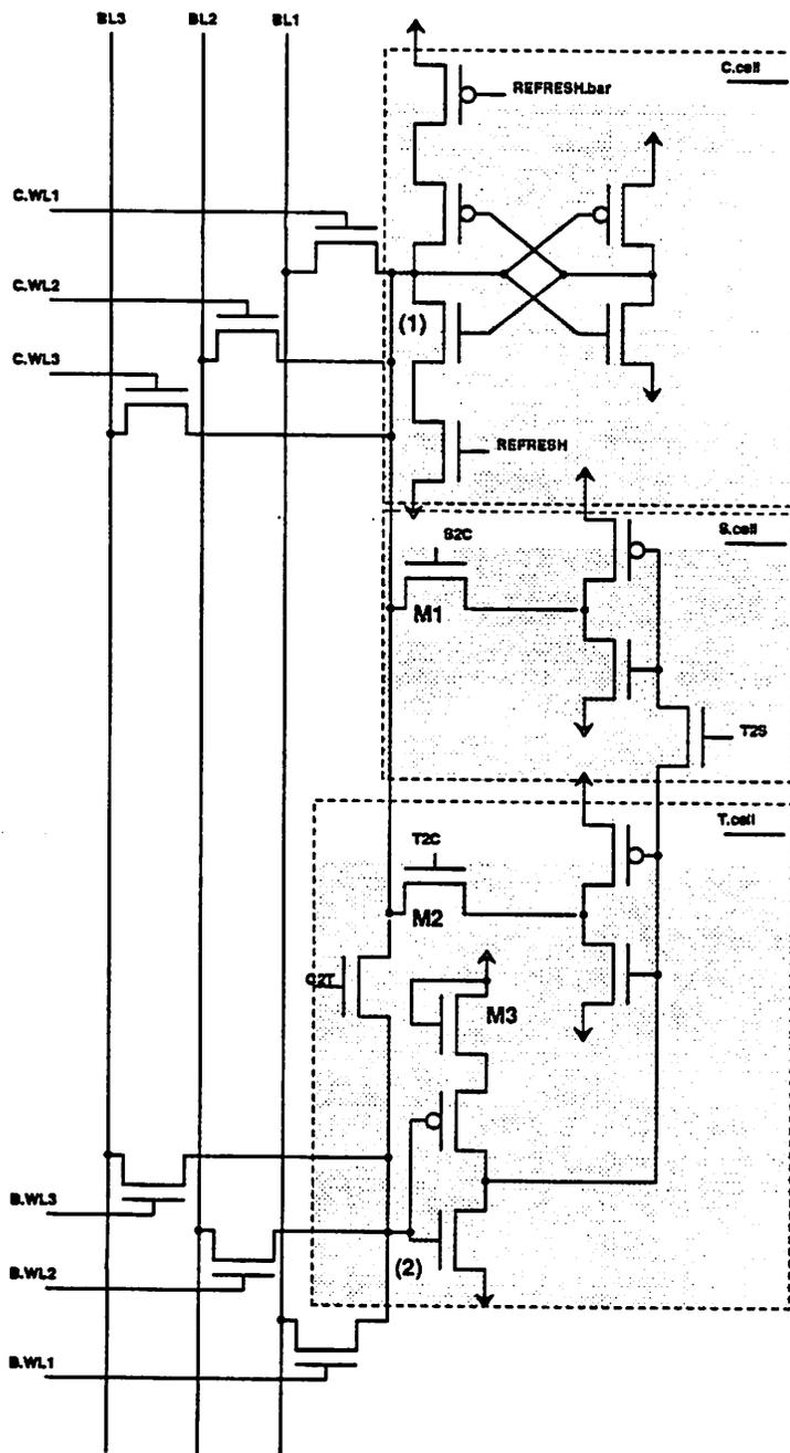
**Fig. 5: Value "Triple-Cell" Schematic**
