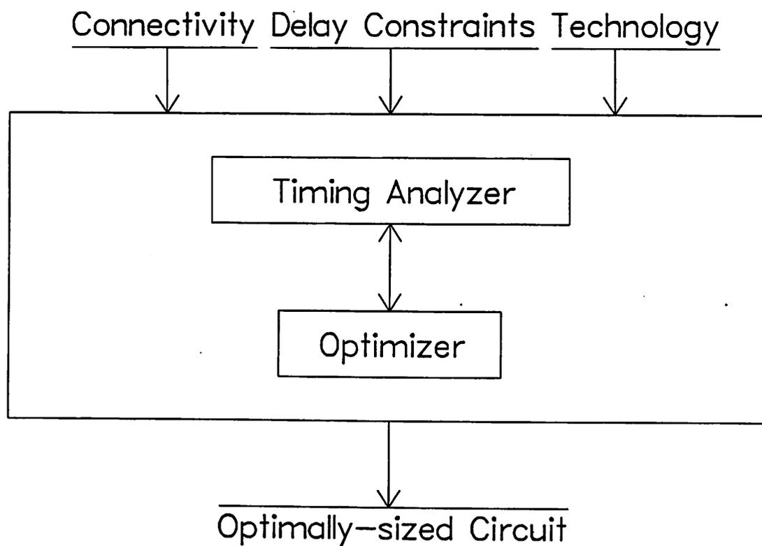
Figure 5.1: Block Diagram of the Transistor Sizer
