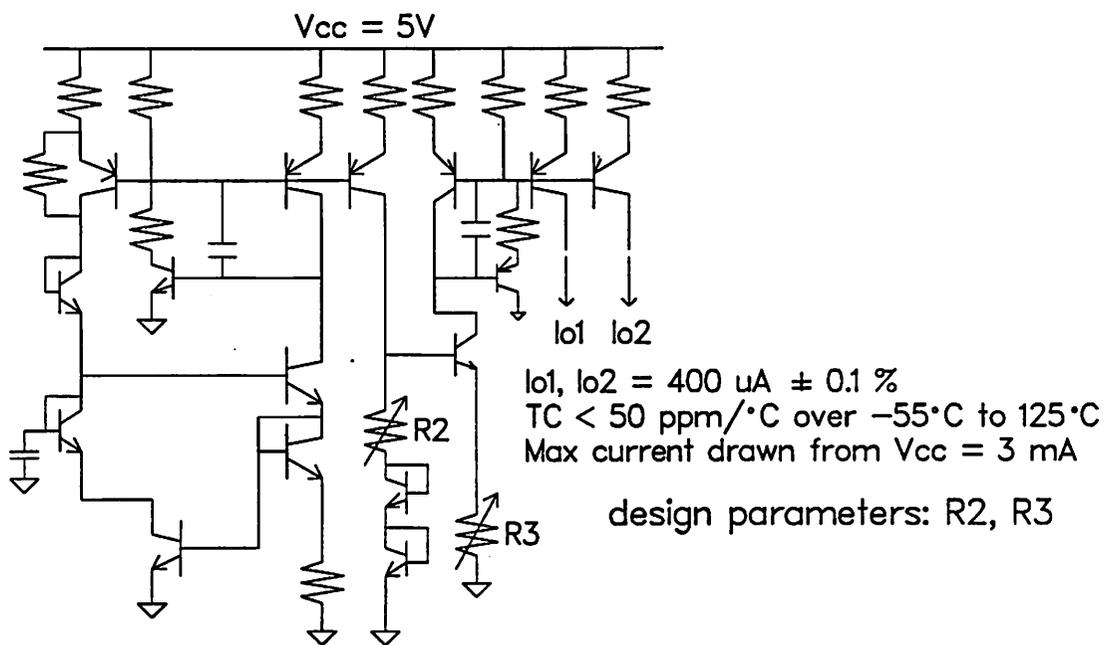
Figure 4.13: Bipolar Current Source
