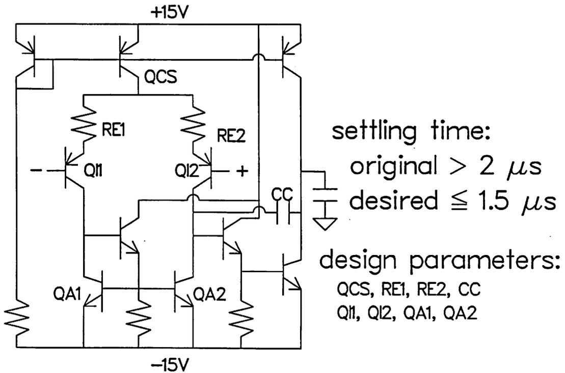
Figure 4.15: Bipolar Operational Amplifier Circuit
