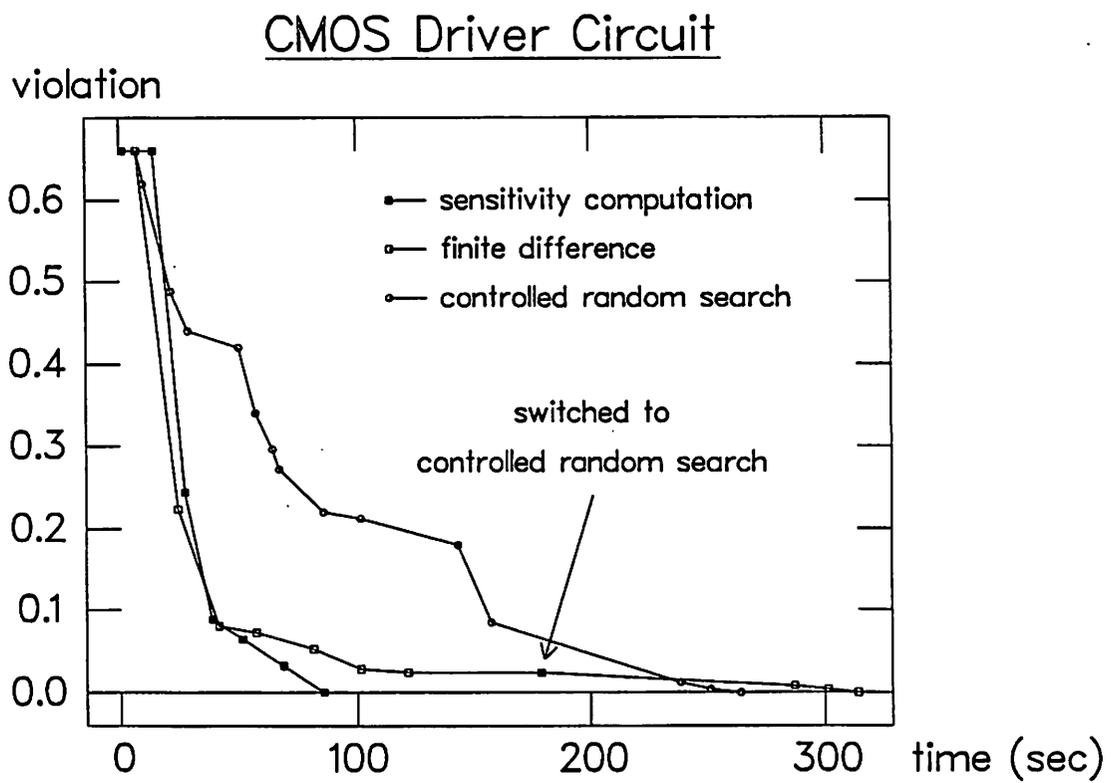
Figure 4.7: Computational Statistics for CMOS I/O Driver Example
