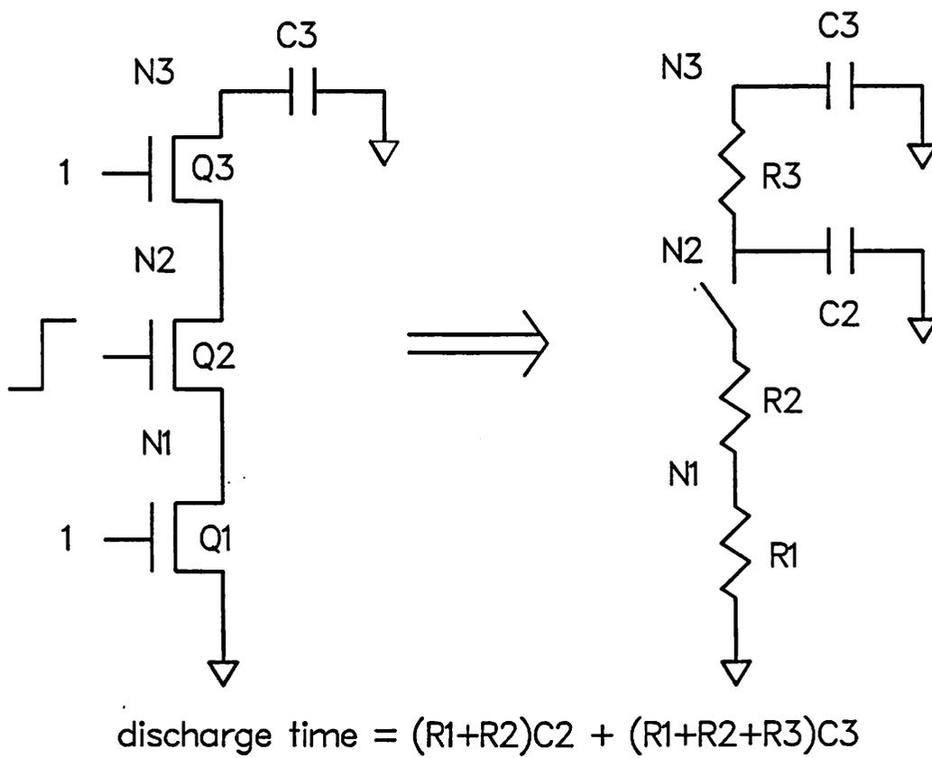
Figure 5.3: RC Delay Model
