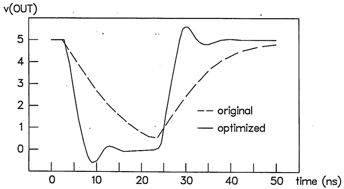
Figure 4.8: Optimization of CMOS I/O Driver Circuit
