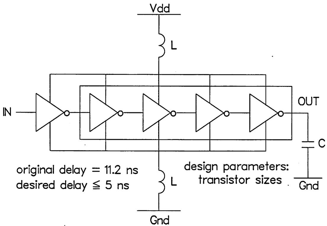
Figure 4.6: CMOS I/O Driver Circuit
